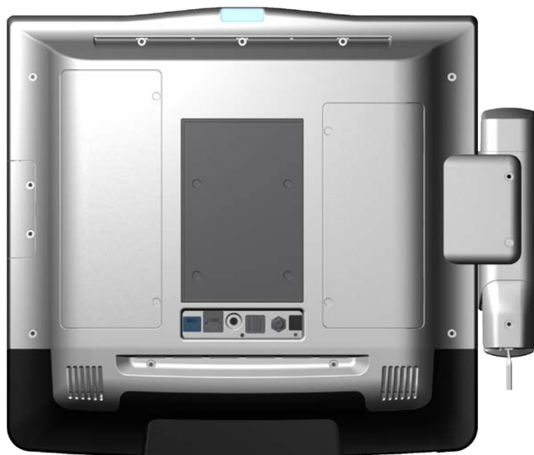
Figure 2.3: Rear view of the Obie Smart Terminal™
