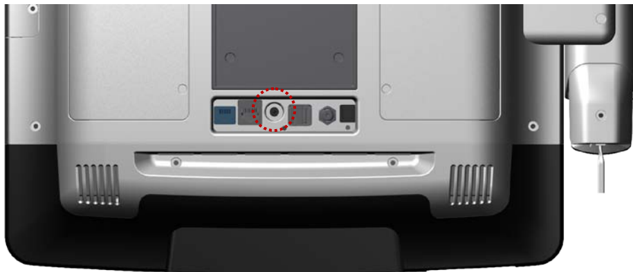
Figure 2.4: Connecting the power cord
