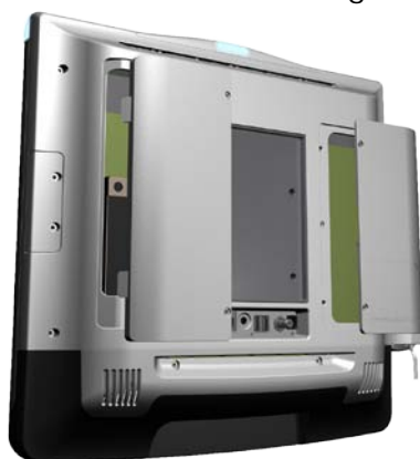
Figure C.1: Disassembling the plastic rear cover of the Obie Unscrew the screws that secure the plastic rear cover, and then remove the covers
