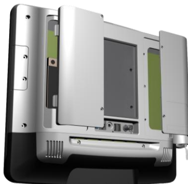
Figure C.1: Disassembling the plastic rear cover of the Jima Unscrew the screws that secure the plastic rear cover, and then remove the covers
