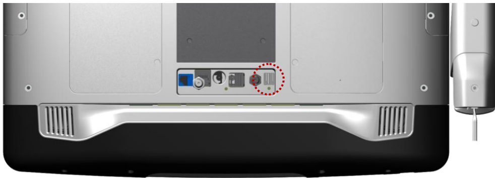
Figure 2.4: Connecting the power cord
