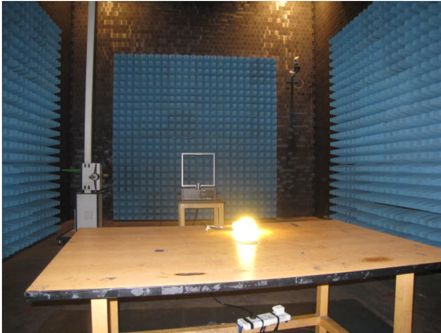
Radiated Emission Test Set-up
