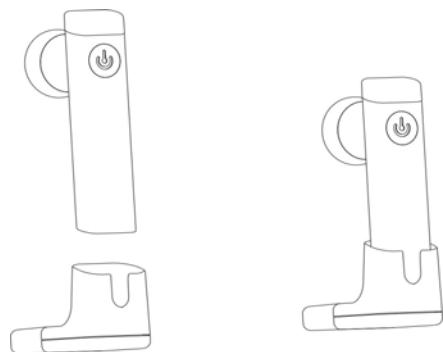
B. When the battery is fully charged. The red indicator light turns off and the blue indicator light turns on. Disconnect the charger from the computer or wall outlet and the headset.
