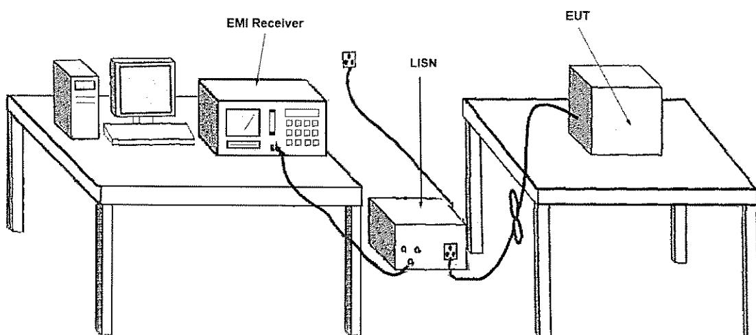
1. The above measurement is made in a shielded room.
