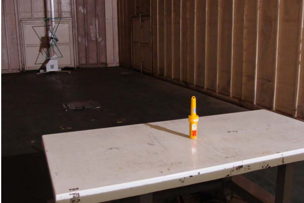
Front View of Radiated Emission Test (Bilog)
