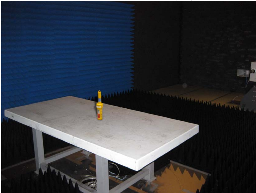
Front View of Radiated Emission Test (Horn)
