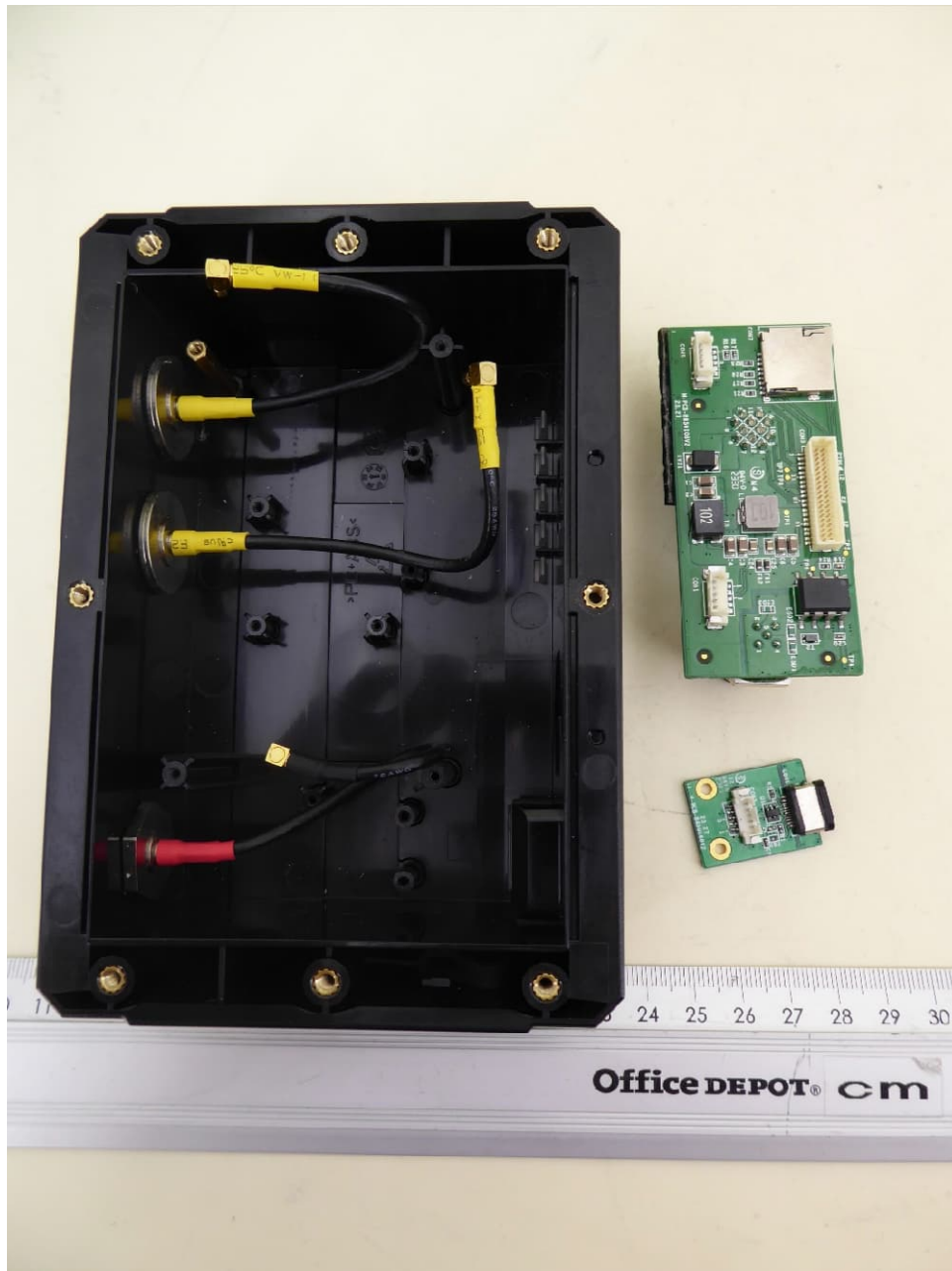
B650S, internal view 3, all PCBs removed
