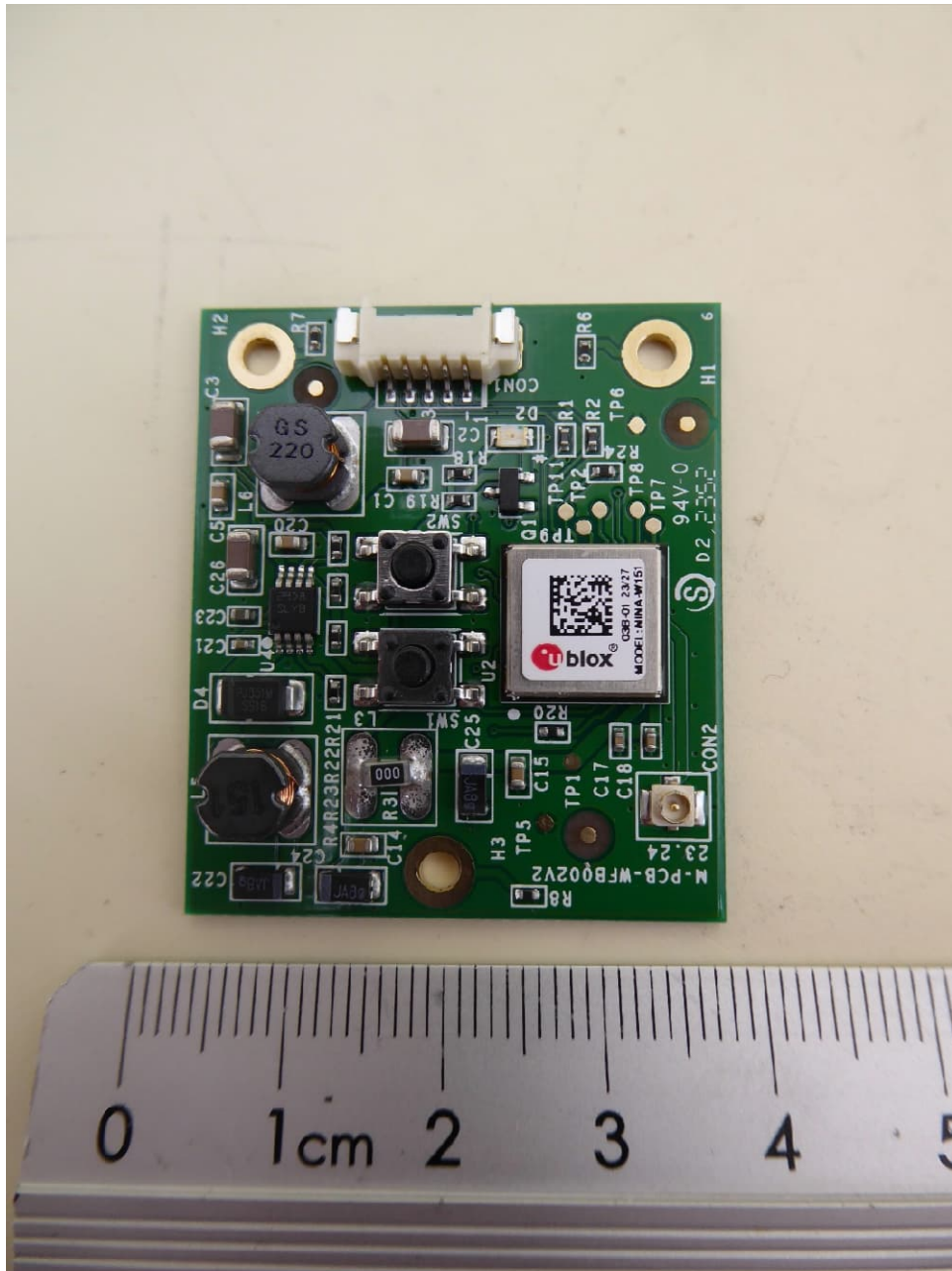
B650WS, Wi-Fi-module, top view
