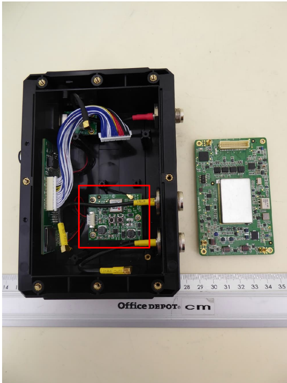
B650WS (with certified Wifi Module FCC ID: WZ7-W151 / IC ID 9547A-W151), internal view 2, main PCB removed
