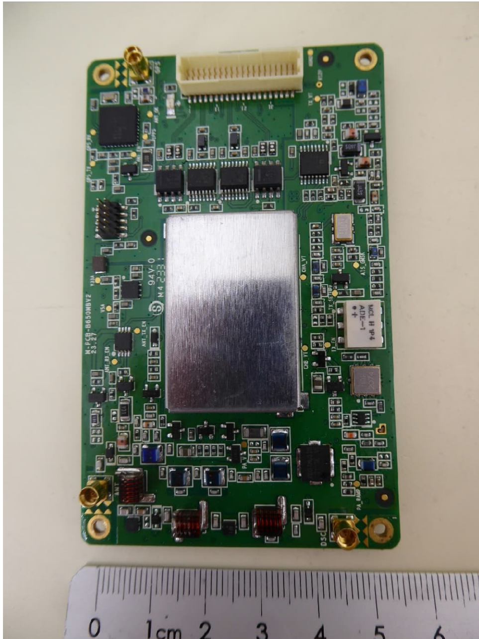
B650S / B650WS, main PCB, top view
