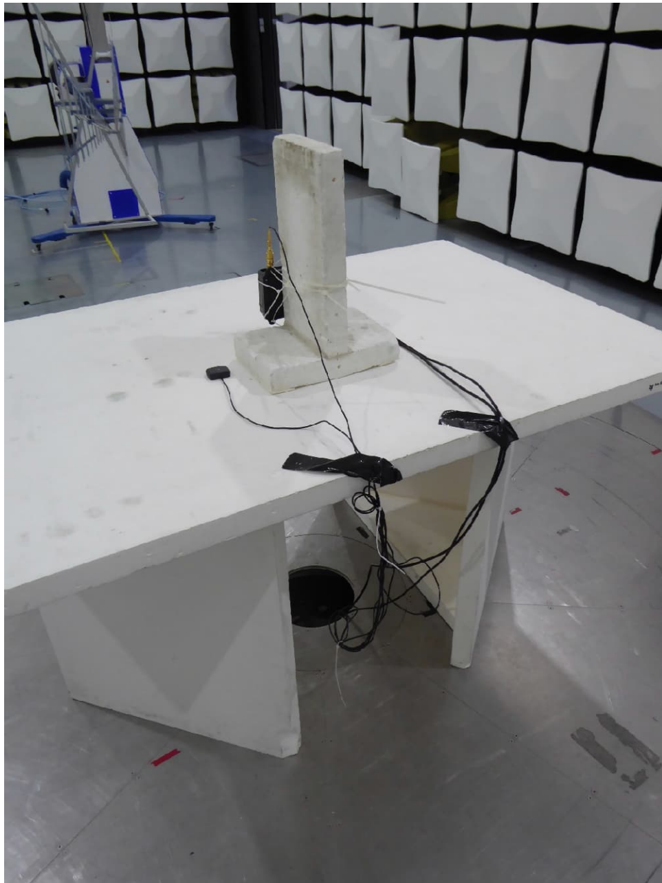
Test setup semi anechoic chamber (30 MHz to 1 GHz, position 3)
