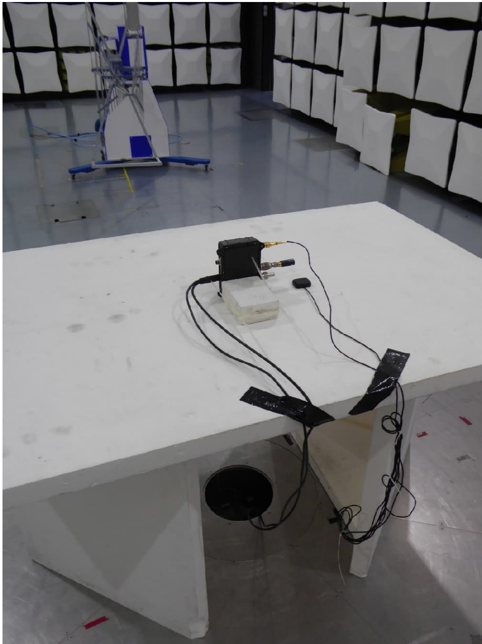
Test setup semi anechoic chamber (30 MHz to 1 GHz, position 2)
