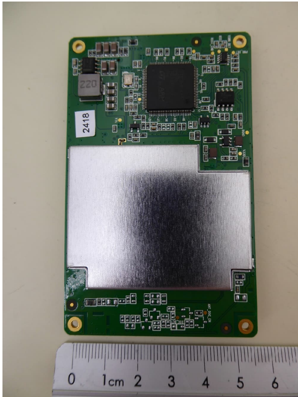
B650 / B650W, main PCB, bottom view
