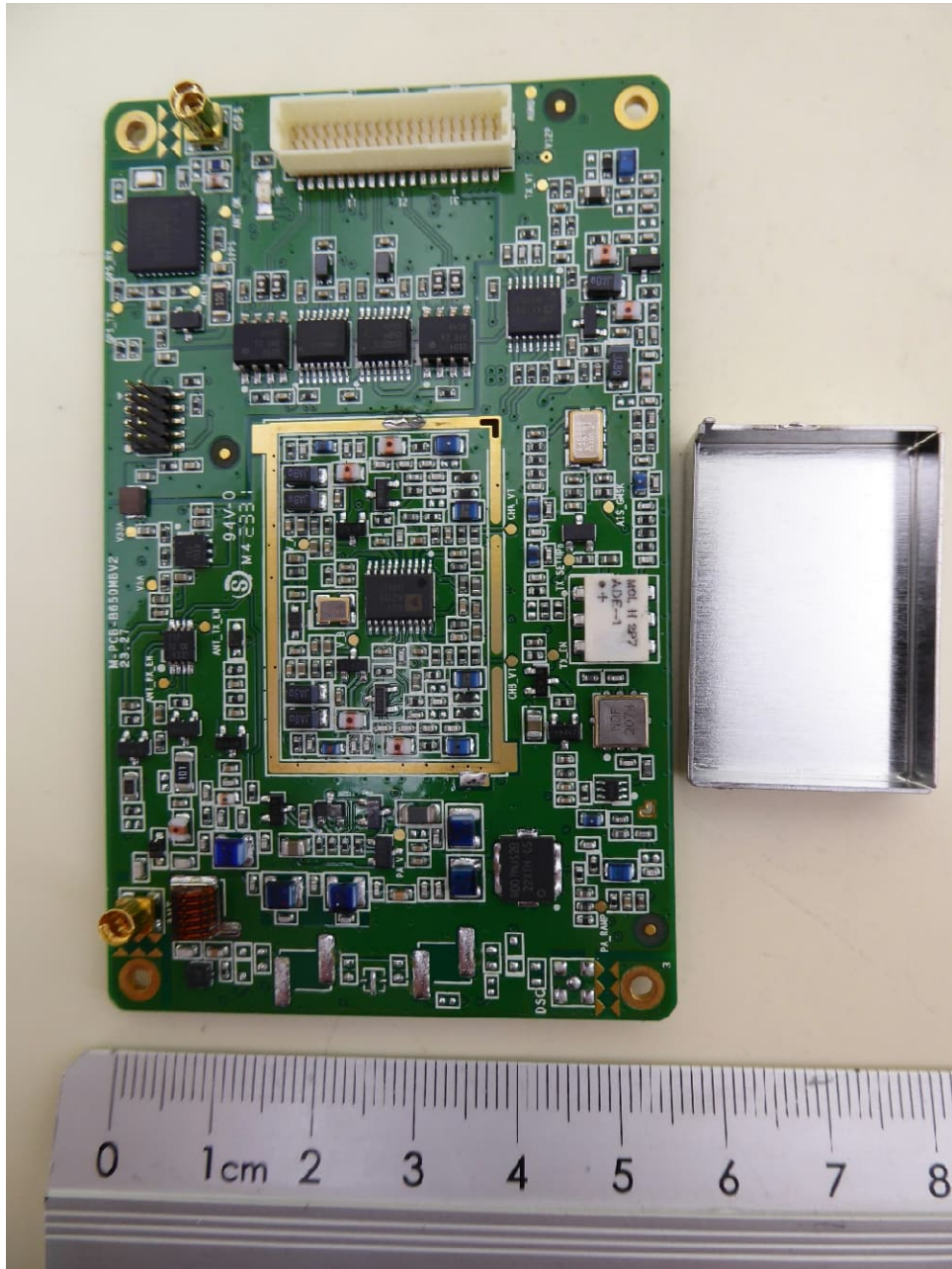
B620 / B620W, main PCB, top view, shielding removed
