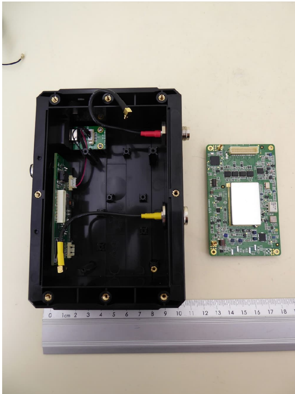
B620, internal view 2, main PCB removed
