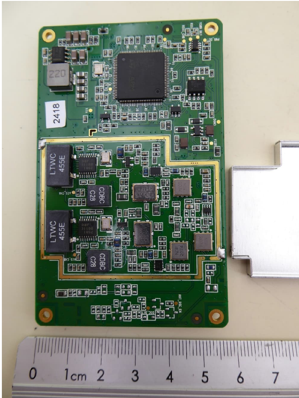
B620 / B620W, main PCB, bottom view, shielding removed
