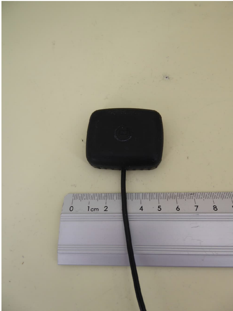
GPS antenna used for radiated tests
