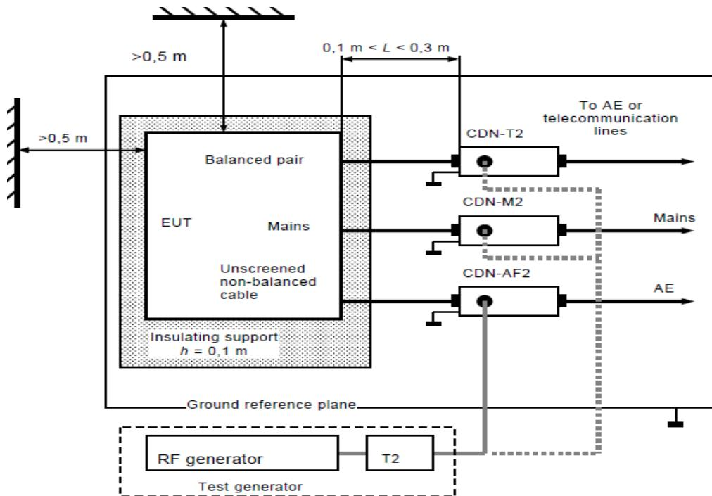
**Note:** 1. The CDNs and / or EM clamp used for real test depends on ports and cables configuration of EUT.
