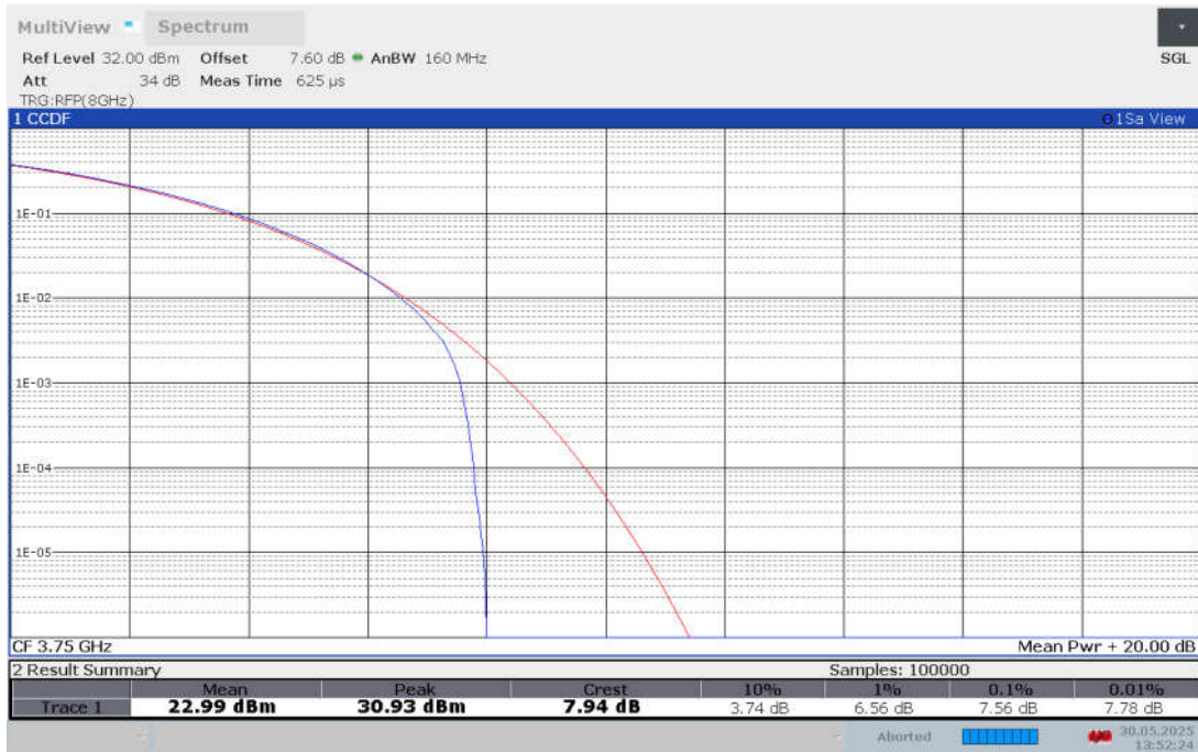
Band n78H , 100MHz Bandwidth,CP-64QAM
