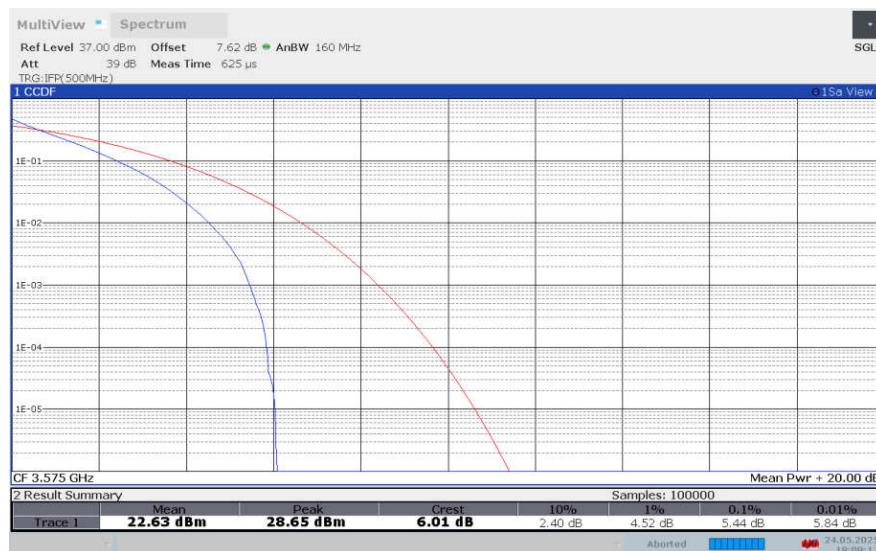
**LTE band 42 , 10MHz Bandwidth,16QAM**
