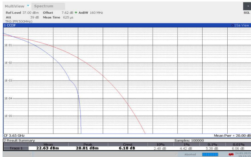
**LTE band 43 , 5MHz Bandwidth,16QAM**
