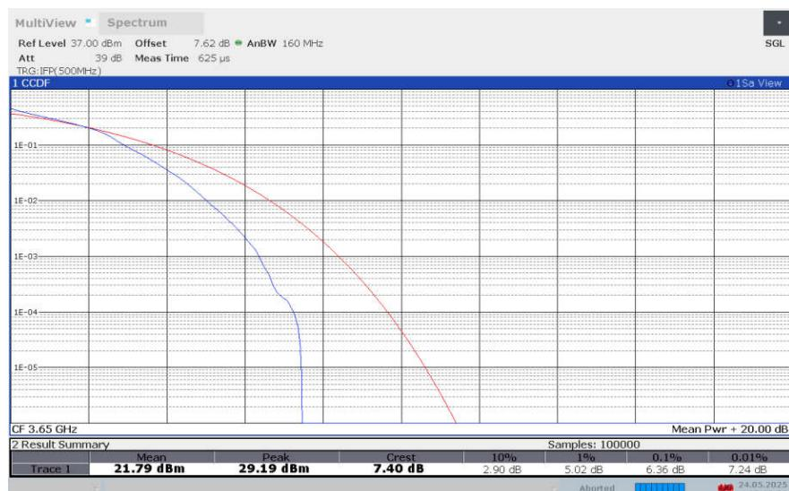
**LTE band 43 , 10MHz Bandwidth,64QAM**
