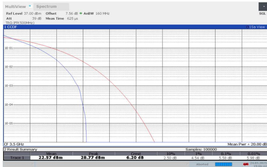
**LTE band 42 , 15MHz Bandwidth,16QAM**
