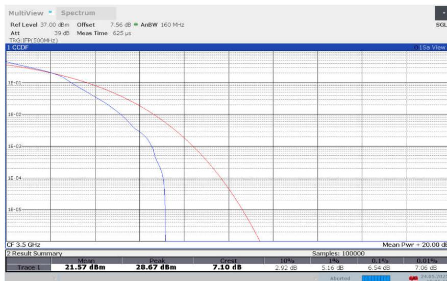
**LTE band 42 , 5MHz Bandwidth,64QAM**
