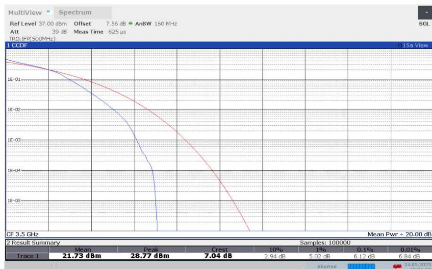
**LTE band 42 , 10MHz Bandwidth,64QAM**
