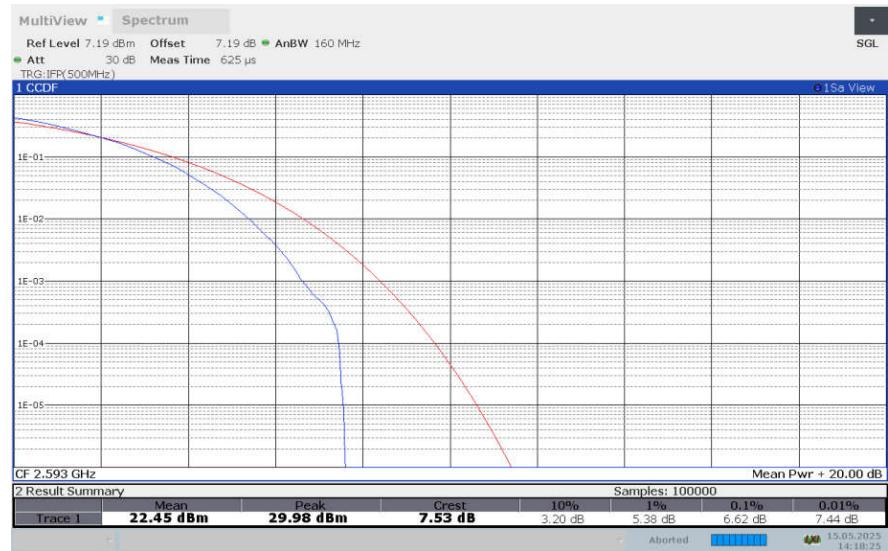
**LTE band 41 , 15MHz Bandwidth,256QAM**
