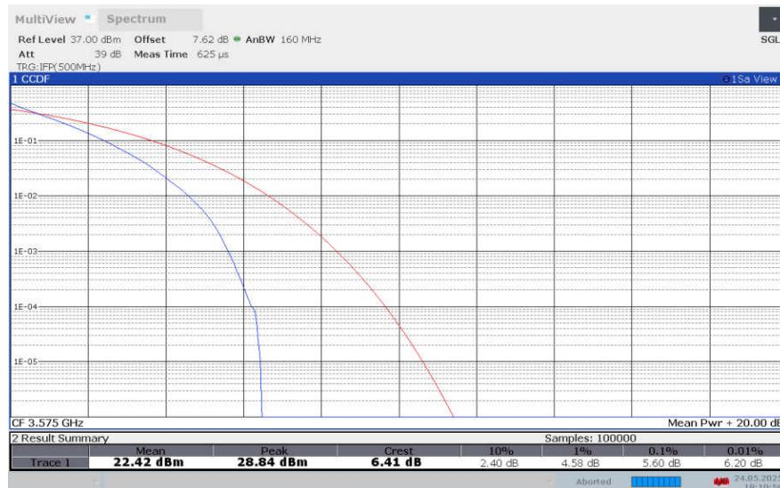
**LTE band 42 , 20MHz Bandwidth,16QAM**
