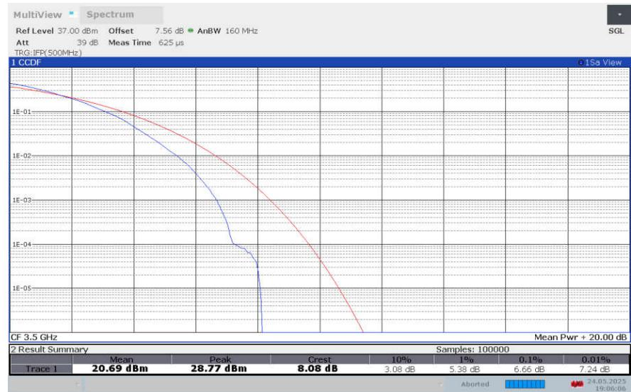
**LTE band 42 , 10MHz Bandwidth,256QAM**
