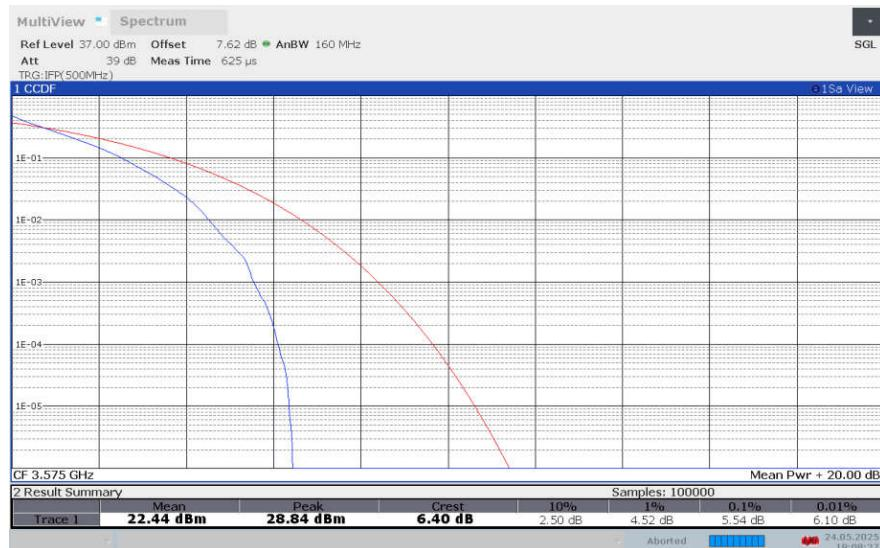
**LTE band 42 , 5MHz Bandwidth,16QAM**
