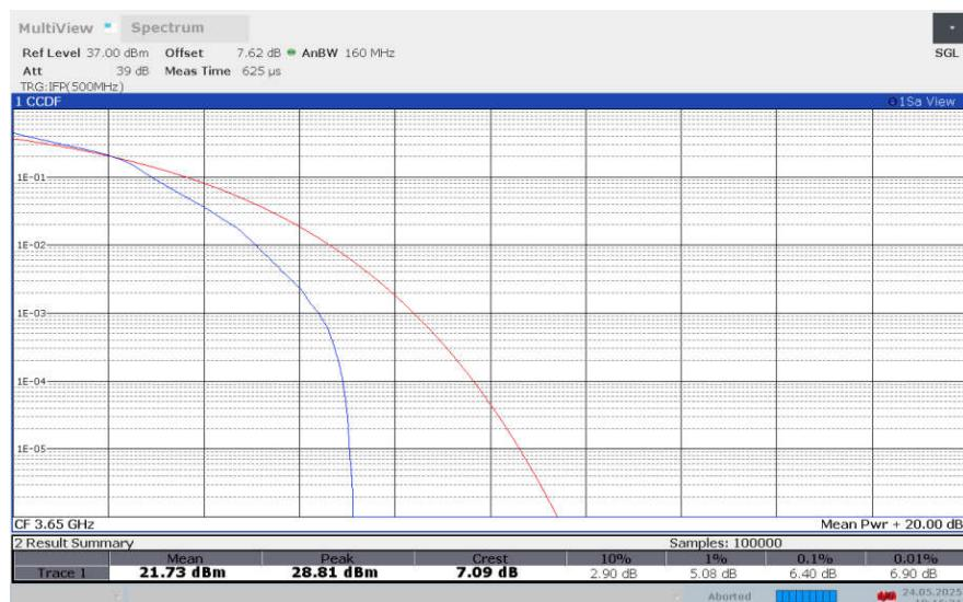
**LTE band 43 , 5MHz Bandwidth,64QAM**
