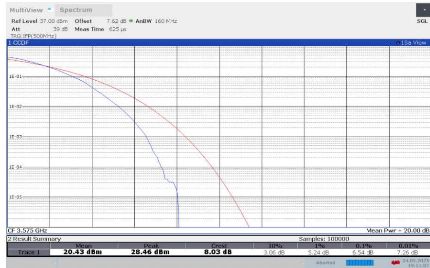
**LTE band 42 , 20MHz Bandwidth,256QAM**
