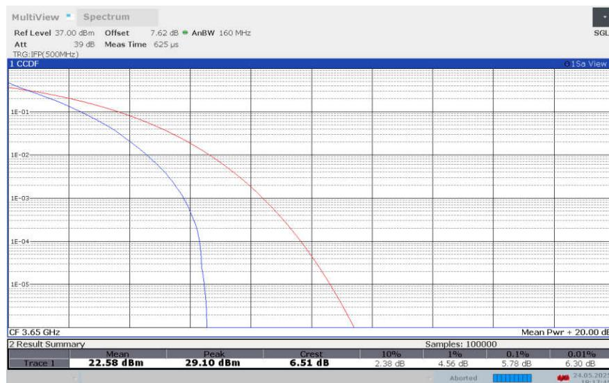
**LTE band 43 , 20MHz Bandwidth,16QAM**
