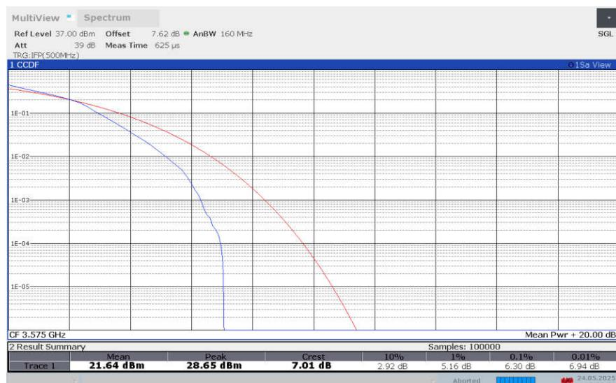
**LTE band 42 , 5MHz Bandwidth,64QAM**
