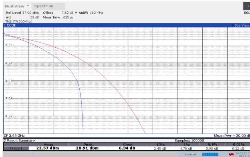
**LTE band 43 , 15MHz Bandwidth,16QAM**
