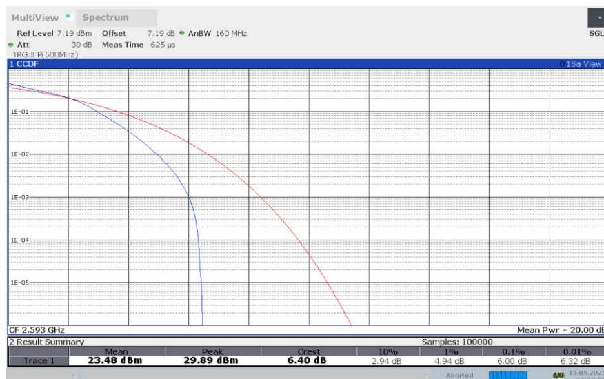
**LTE band 41 , 20MHz Bandwidth,64QAM**
