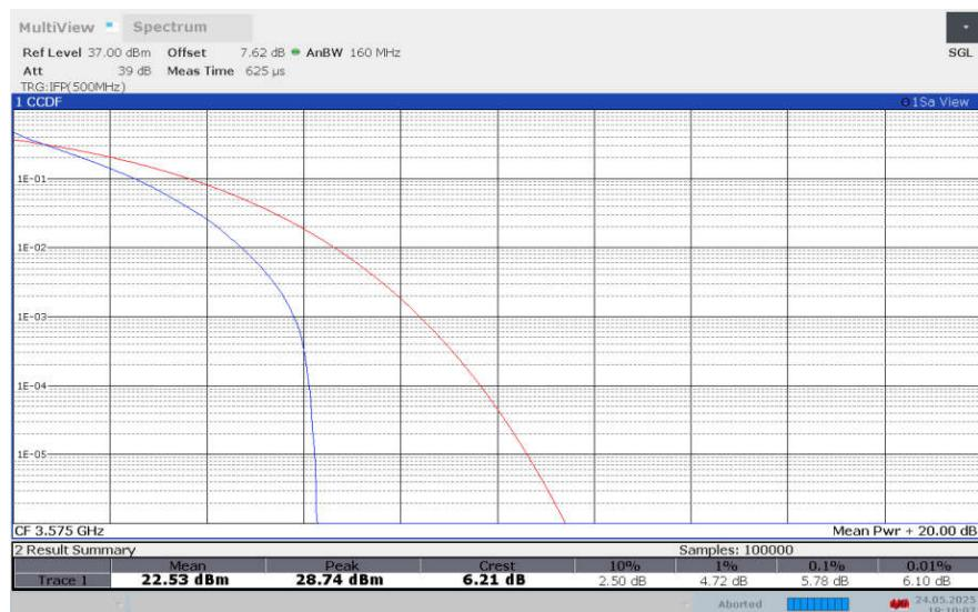
**LTE band 42 , 15MHz Bandwidth,16QAM**
