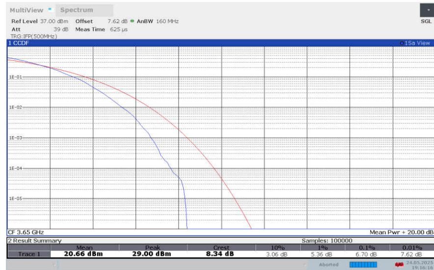
**LTE band 43 , 10MHz Bandwidth,256QAM**
