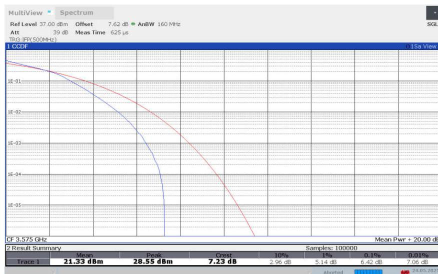
**LTE band 42 , 20MHz Bandwidth,64QAM**
