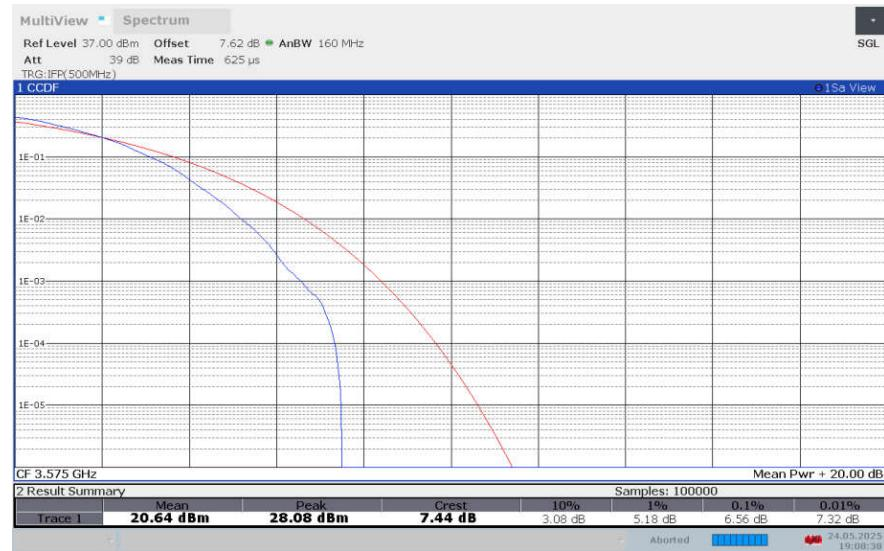
**LTE band 42 , 5MHz Bandwidth,256QAM**
