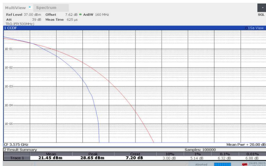
**LTE band 42 , 15MHz Bandwidth,64QAM**
