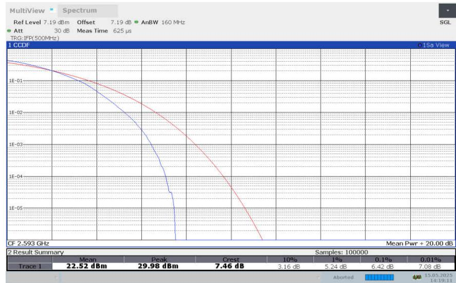
**LTE band 41 , 20MHz Bandwidth,256QAM**
