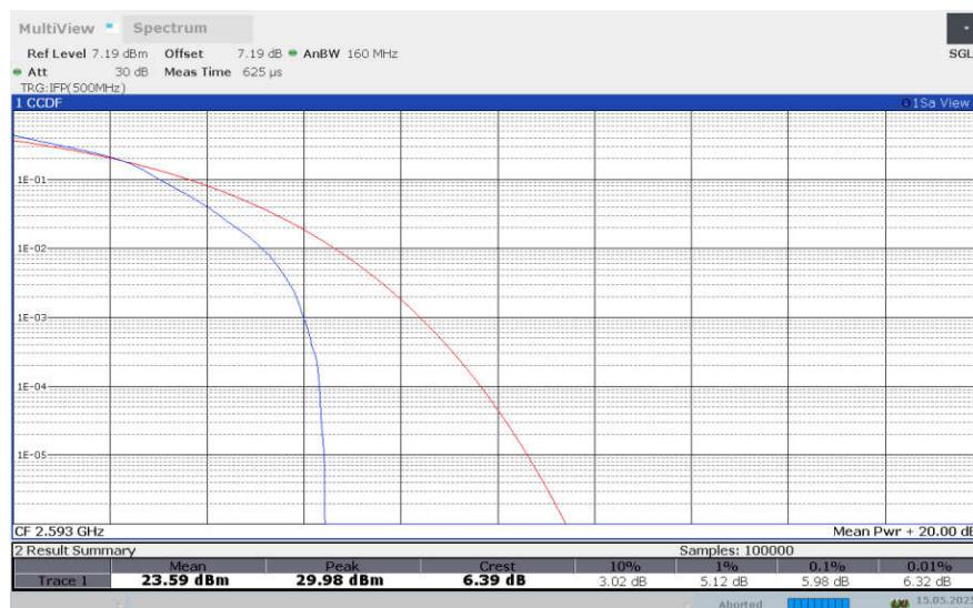
**LTE band 41 , 15MHz Bandwidth,64QAM**
