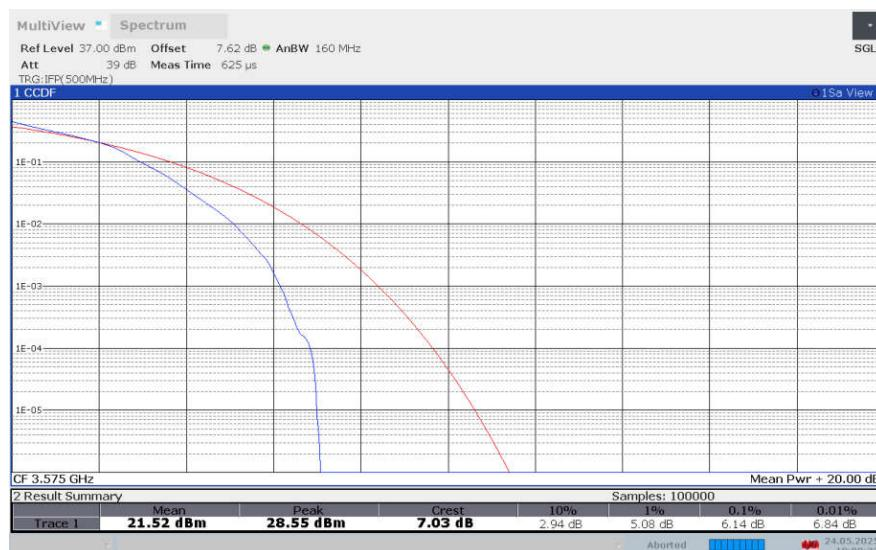
**LTE band 42 , 10MHz Bandwidth,64QAM**
