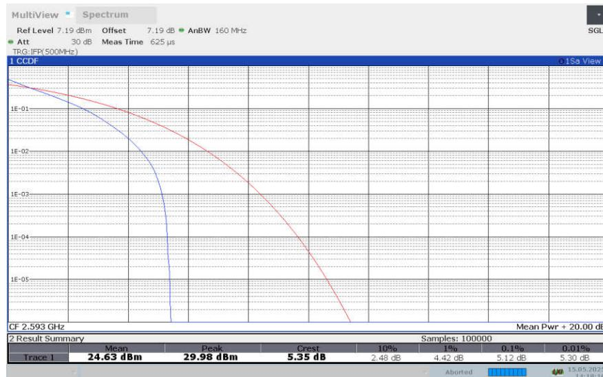
**LTE band 41 , 15MHz Bandwidth,16QAM**
