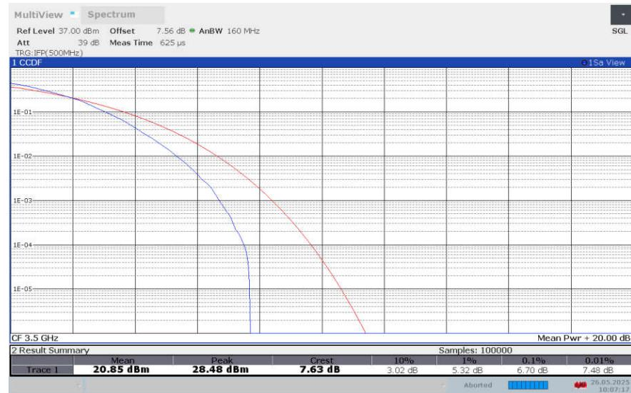
**LTE band 42 , 5MHz Bandwidth,256QAM**
