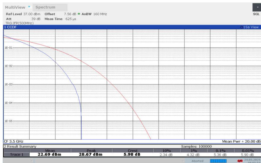
**LTE band 42 , 10MHz Bandwidth,16QAM**
