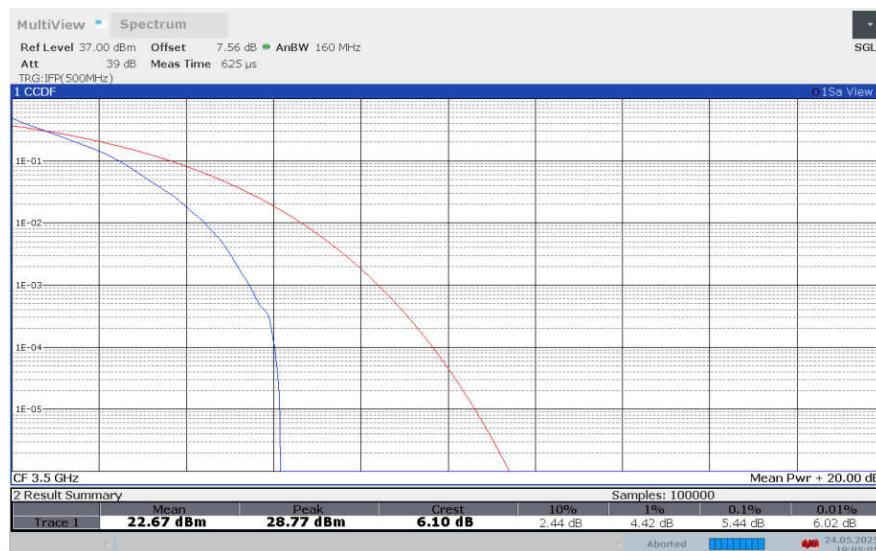
**LTE band 42 , 5MHz Bandwidth,16QAM**
