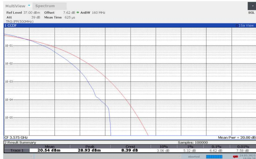
**LTE band 42 , 10MHz Bandwidth,256QAM**
