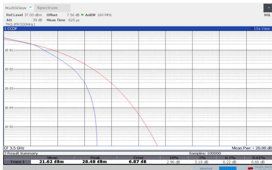
**LTE band 42 , 15MHz Bandwidth,64QAM**
