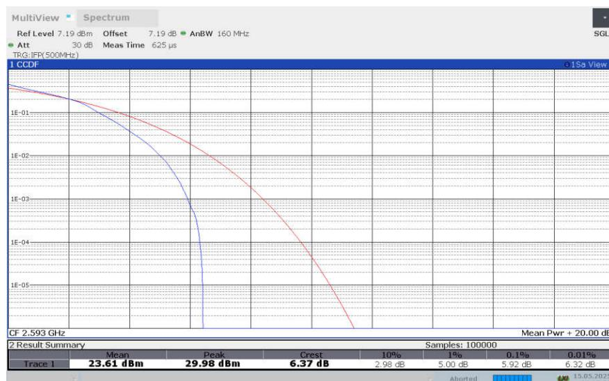
**LTE band 41 , 10MHz Bandwidth,64QAM**
