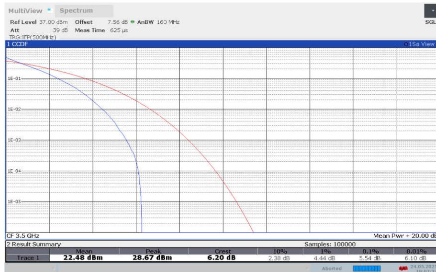
**LTE band 42 , 20MHz Bandwidth,16QAM**
