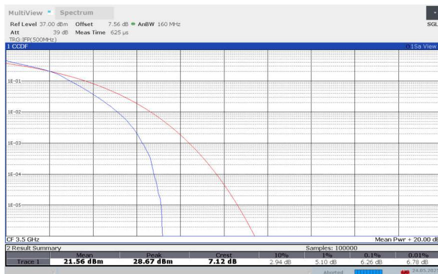
**LTE band 42 , 20MHz Bandwidth,64QAM**
