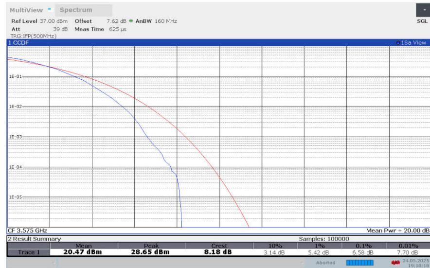
**LTE band 42 , 15MHz Bandwidth,256QAM**
