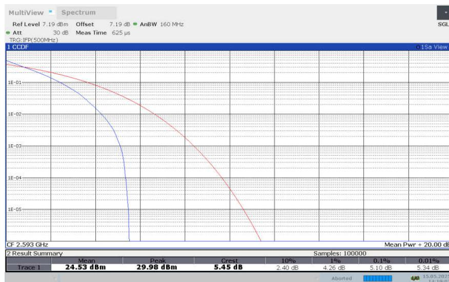
**LTE band 41 , 20MHz Bandwidth,16QAM**
