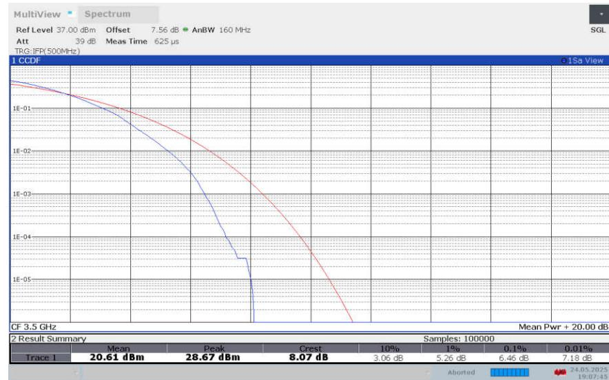
**LTE band 42 , 20MHz Bandwidth,256QAM**
