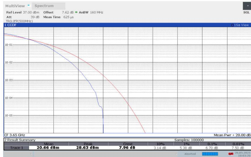
**LTE band 43 , 15MHz Bandwidth,256QAM**
