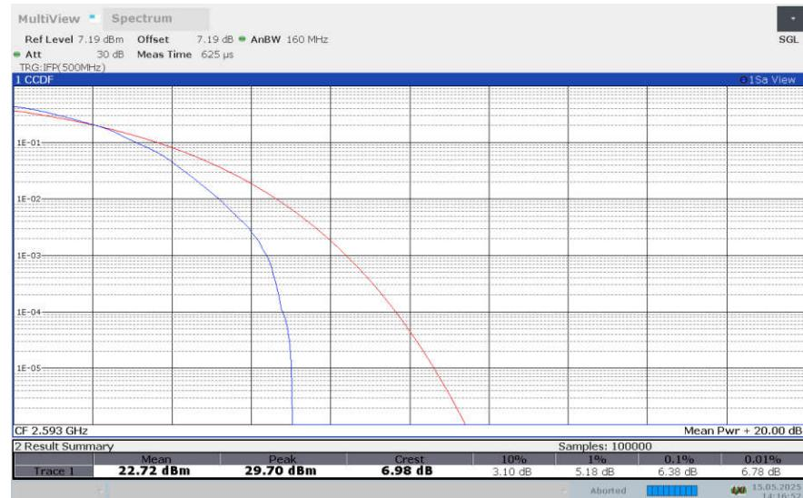
**LTE band 41 , 5MHz Bandwidth,256QAM**
