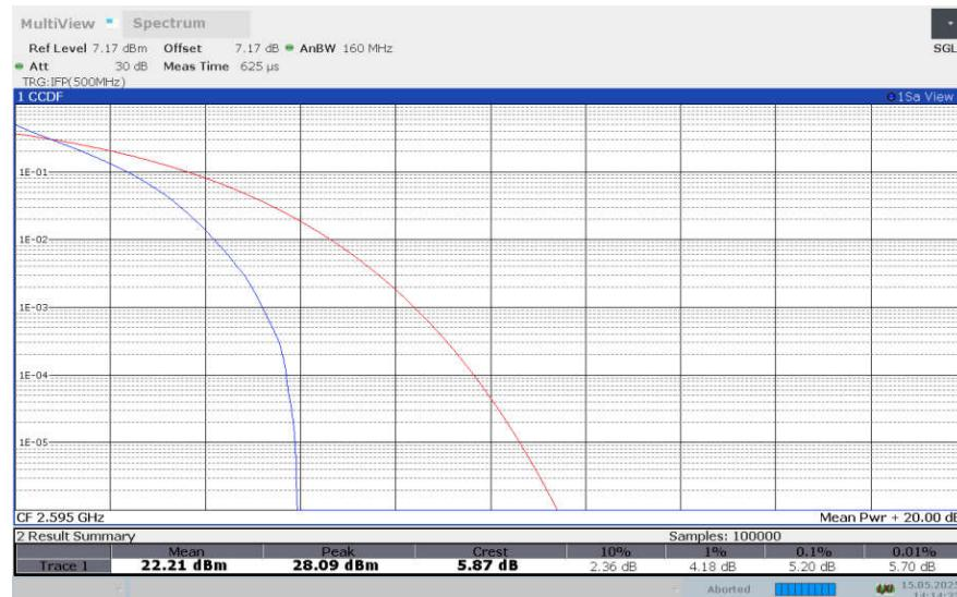
**LTE band 38 , 10MHz Bandwidth,16QAM**
