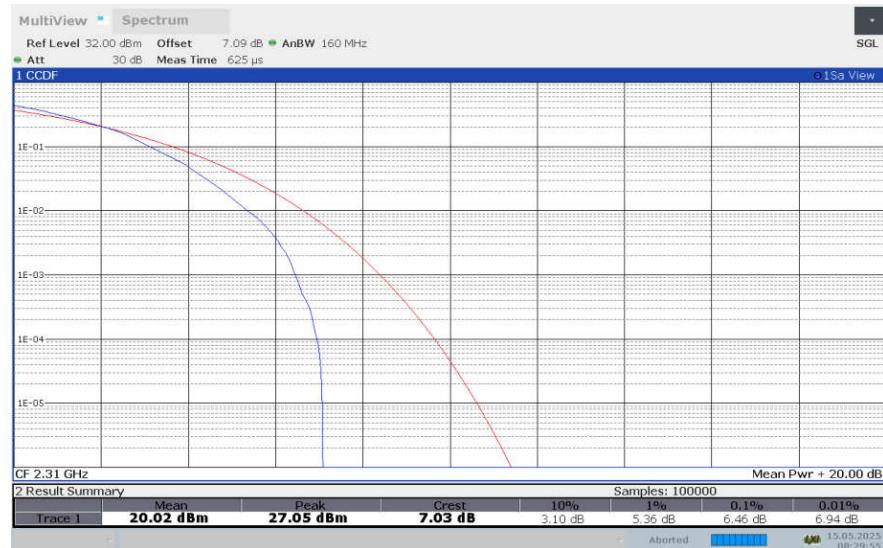
**LTE band 30 , 5MHz Bandwidth,256QAM**
