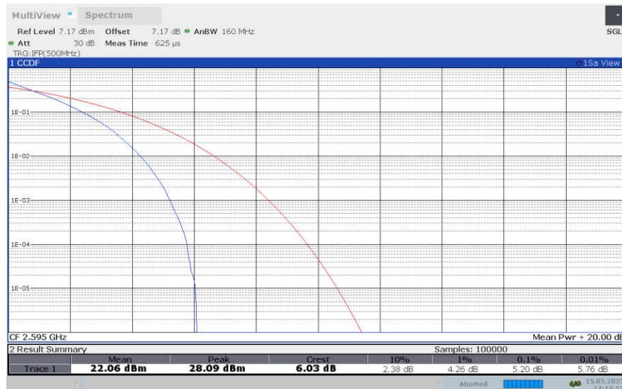
**LTE band 38 , 20MHz Bandwidth,16QAM**
