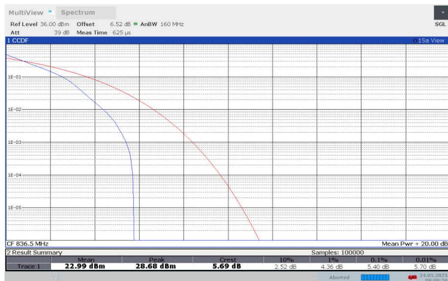
**LTE band 26 , 3MHz Bandwidth,16QAM**
