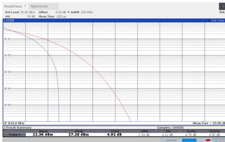
**LTE band 26 , 3MHz Bandwidth,16QAM**
