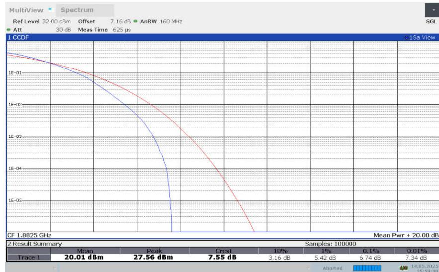
**LTE band 25 , 20MHz Bandwidth,256QAM**
