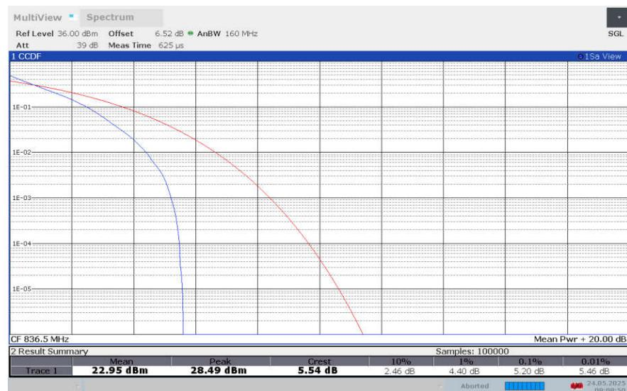
**LTE band 26 , 5MHz Bandwidth,16QAM**
