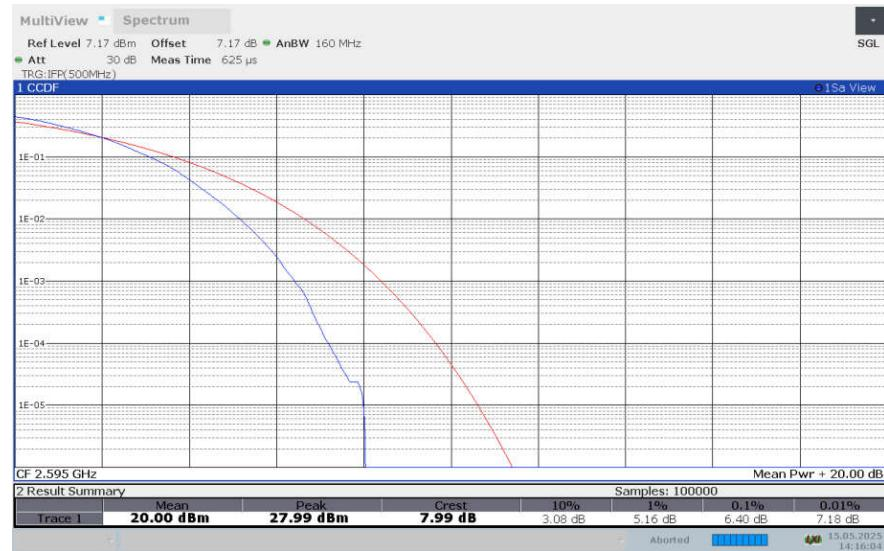
**LTE band 38 , 20MHz Bandwidth,256QAM**
