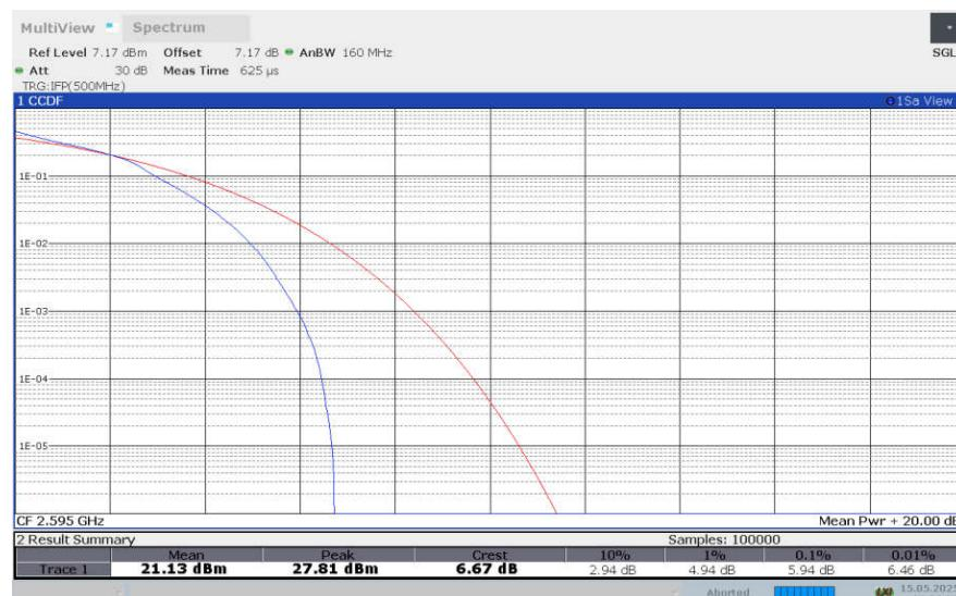
**LTE band 38 , 10MHz Bandwidth,64QAM**
