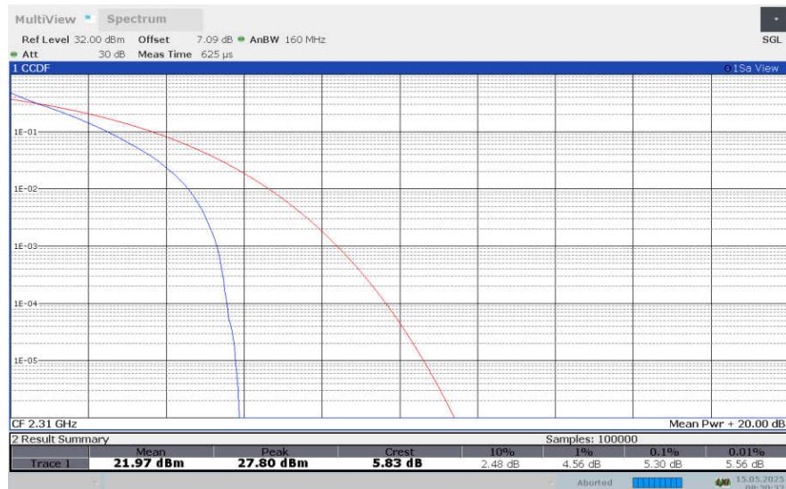
**LTE band 30 , 10MHz Bandwidth,16QAM**
