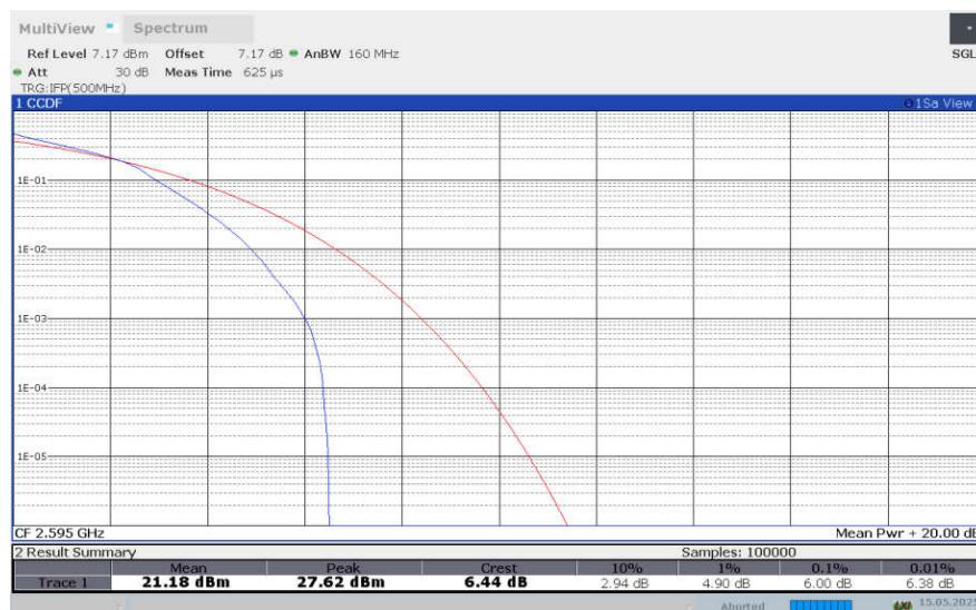
**LTE band 38 , 5MHz Bandwidth,64QAM**
