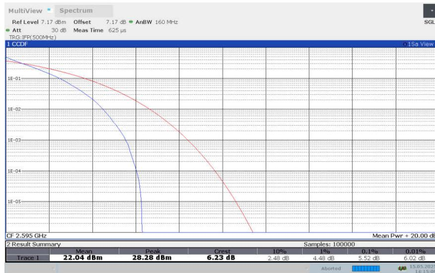
**LTE band 38 , 15MHz Bandwidth,16QAM**
