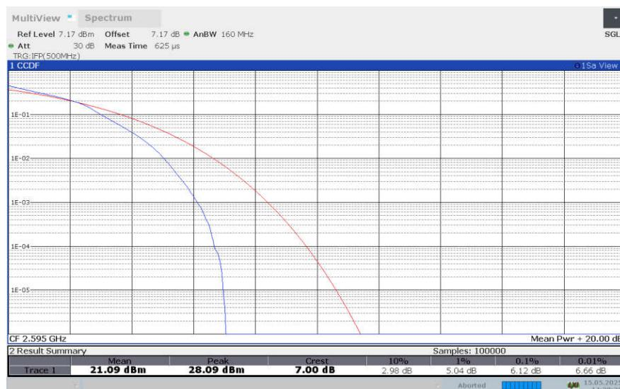
**LTE band 38 , 15MHz Bandwidth,64QAM**
