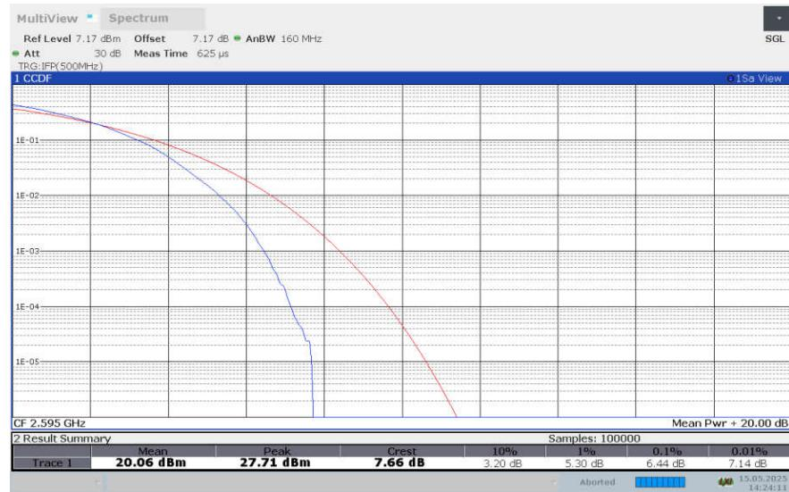
**LTE band 38 , 15MHz Bandwidth,256QAM**
