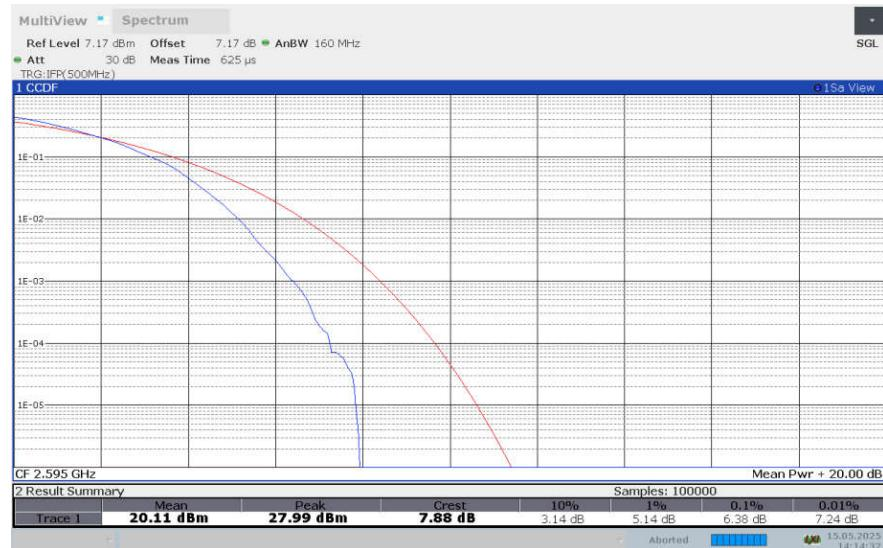
**LTE band 38 , 10MHz Bandwidth,256QAM**
