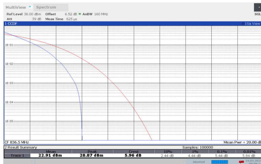
**LTE band 26 , 10MHz Bandwidth,16QAM**
