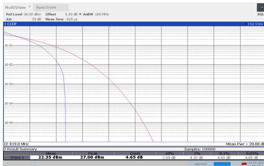
**LTE band 26 , 1.4MHz Bandwidth,16QAM**
