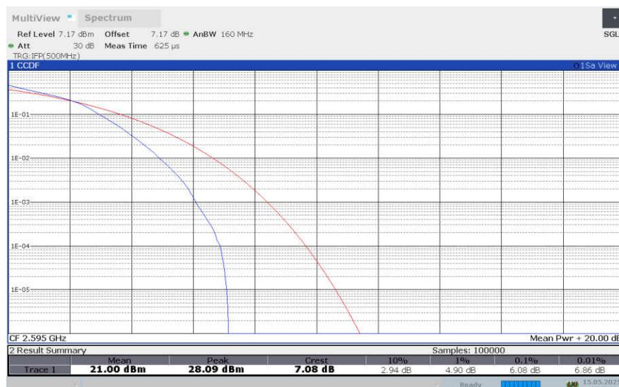
**LTE band 38 , 20MHz Bandwidth,64QAM**
