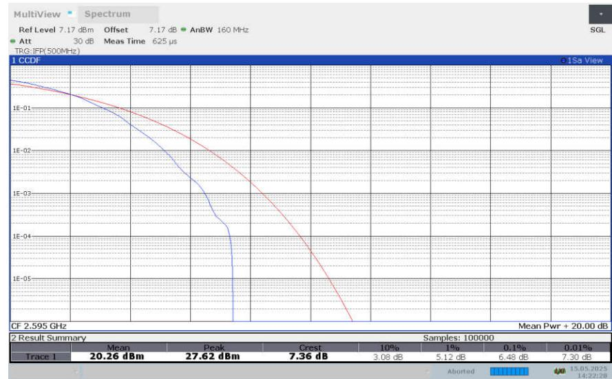
**LTE band 38 , 5MHz Bandwidth,256QAM**
