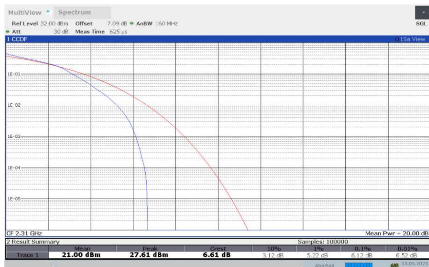
**LTE band 30 , 10MHz Bandwidth,64QAM**
