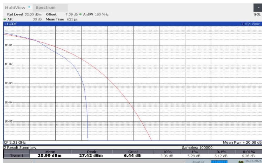
**LTE band 30 , 5MHz Bandwidth,64QAM**
