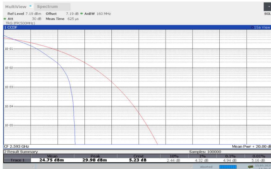
**LTE band 41 , 5MHz Bandwidth,16QAM**
