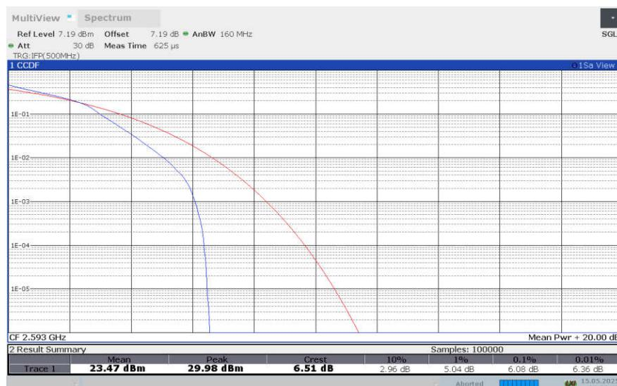
**LTE band 41 , 5MHz Bandwidth,64QAM**
