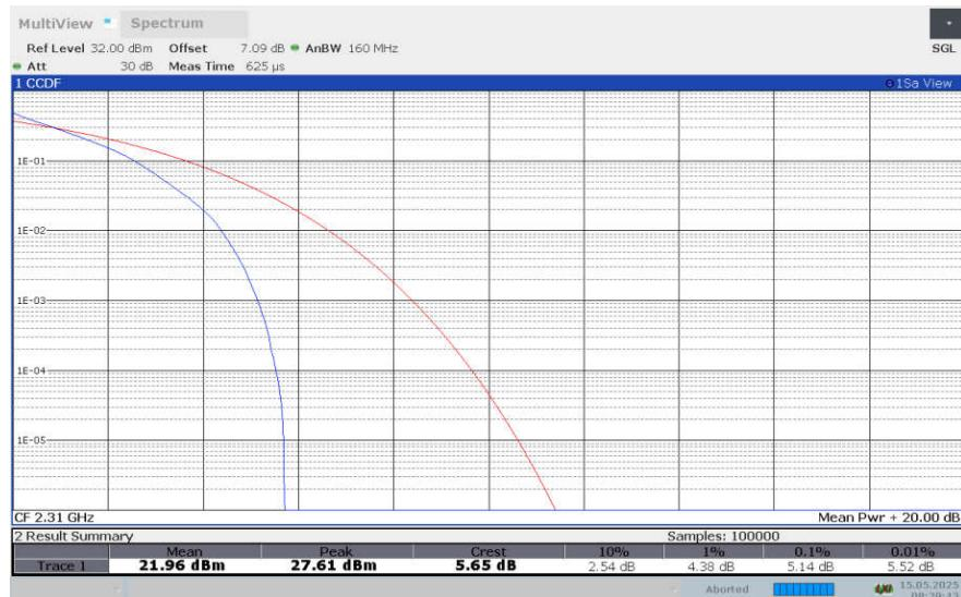
**LTE band 30 , 5MHz Bandwidth,16QAM**
