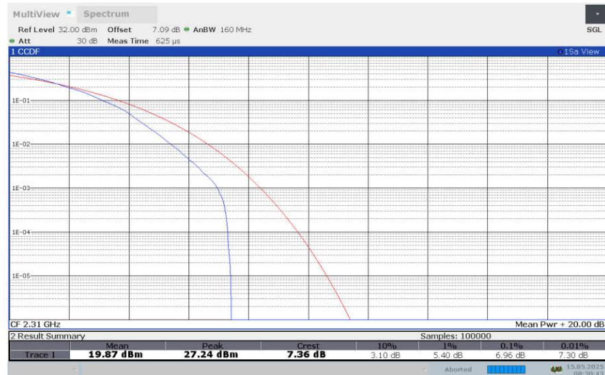
**LTE band 30 , 10MHz Bandwidth,256QAM**
