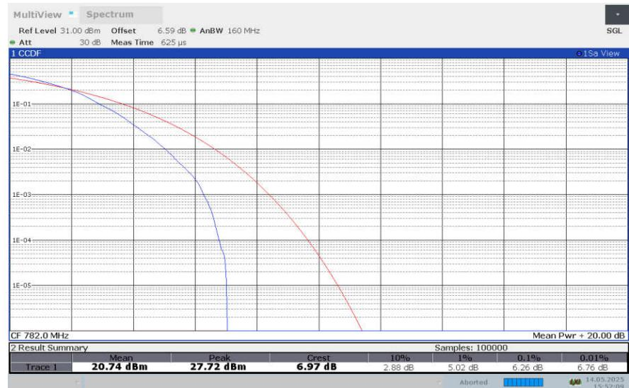
**LTE band 13 , 5MHz Bandwidth,256QAM**
