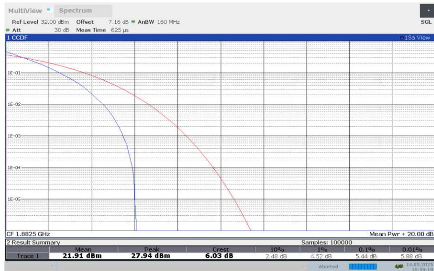
**LTE band 25 , 20MHz Bandwidth,16QAM**
