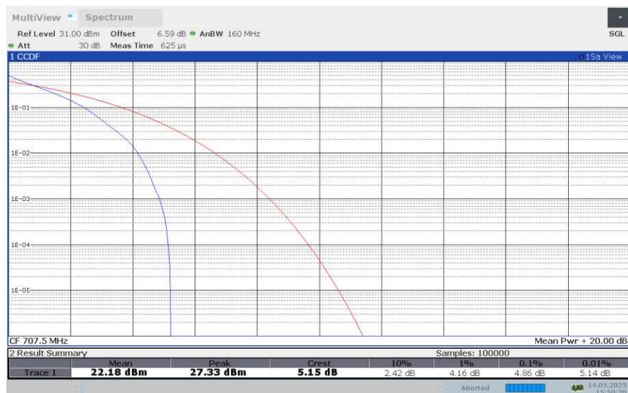
**LTE band 12 , 5MHz Bandwidth,16QAM**
