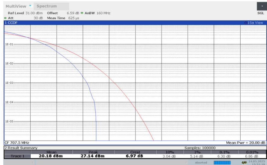
**LTE band 12 , 10MHz Bandwidth,256QAM**
