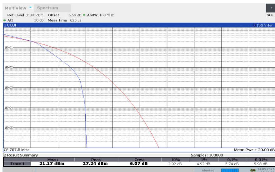
**LTE band 12 , 3MHz Bandwidth,64QAM**
