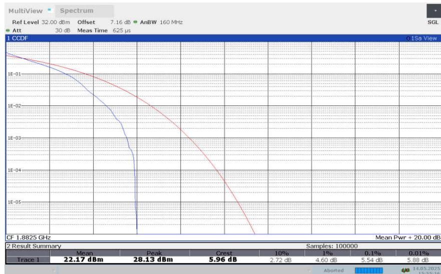
**LTE band 25 , 1.4MHz Bandwidth,16QAM**
