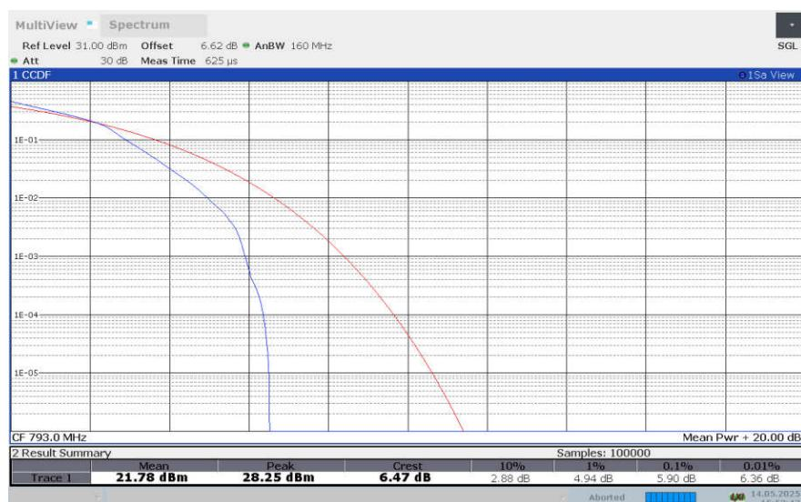
**LTE band 14 , 5MHz Bandwidth,64QAM**
