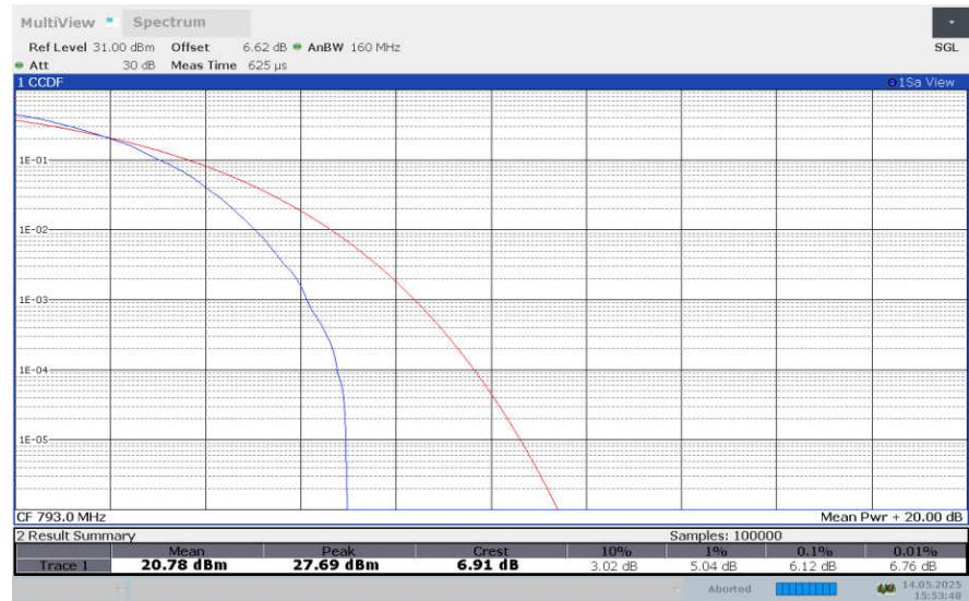
**LTE band 14 , 5MHz Bandwidth,256QAM**
