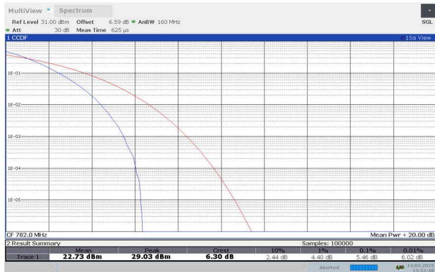
**LTE band 13 , 10MHz Bandwidth,16QAM**
