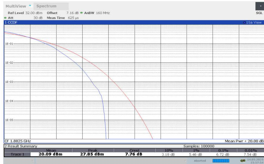
**LTE band 25 , 10MHz Bandwidth,256QAM**
