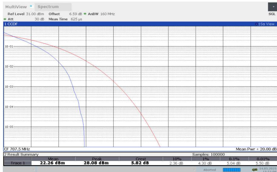
**LTE band 12 , 10MHz Bandwidth,16QAM**
