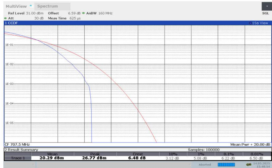
**LTE band 12 , 1.4MHz Bandwidth,256QAM**
