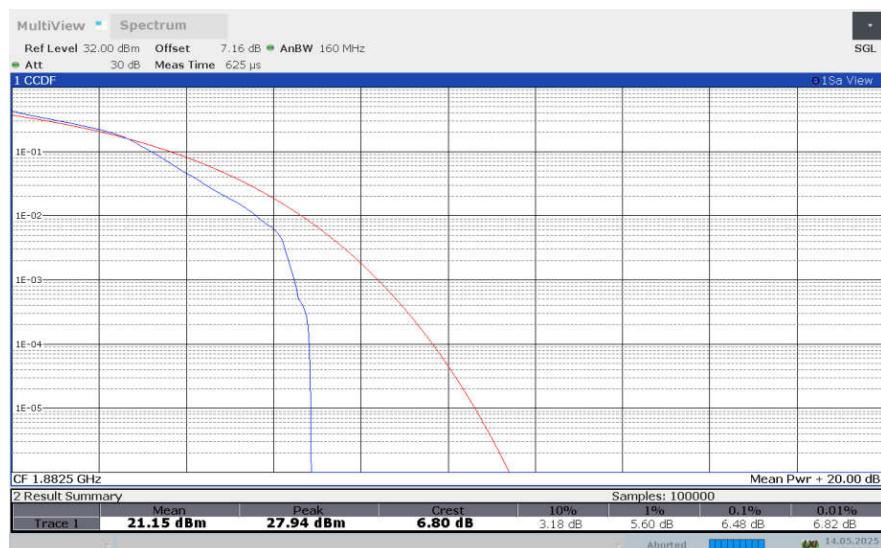
**LTE band 25 , 1.4MHz Bandwidth,64QAM**
