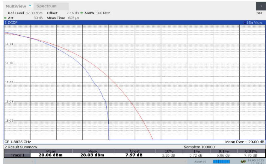
**LTE band 25 , 15MHz Bandwidth,256QAM**
