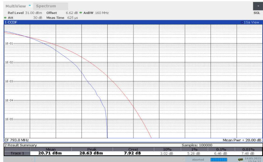
**LTE band 14 , 10MHz Bandwidth,256QAM**
