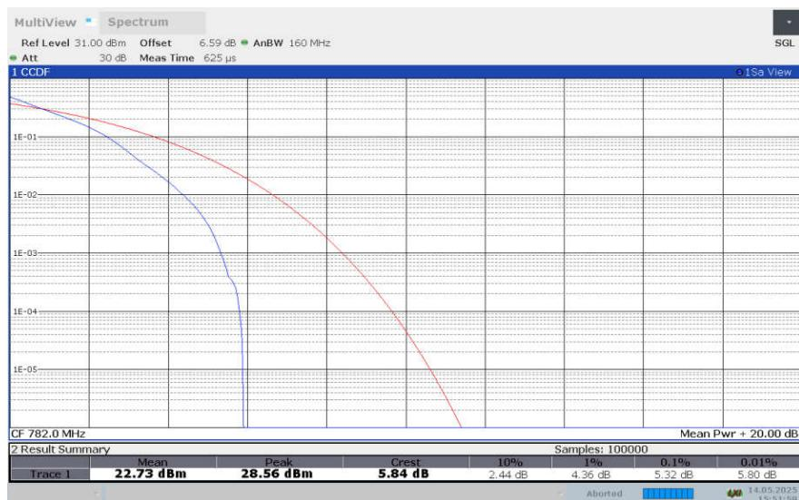
**LTE band 13 , 5MHz Bandwidth,16QAM**
