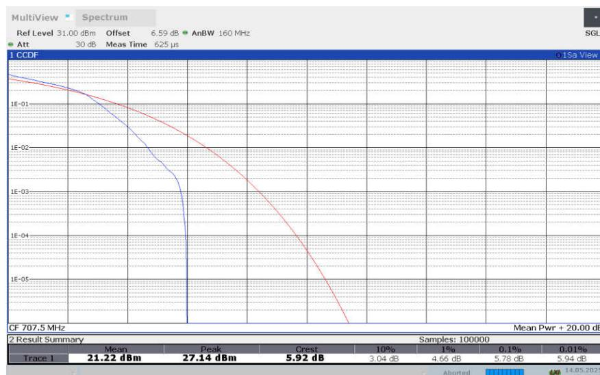
**LTE band 12 , 1.4MHz Bandwidth,64QAM**
