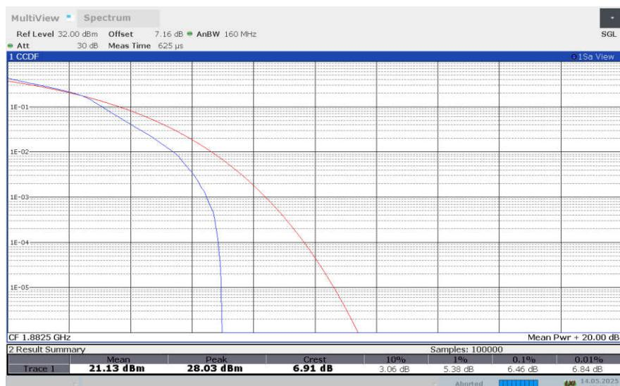
**LTE band 25 , 3MHz Bandwidth,64QAM**
