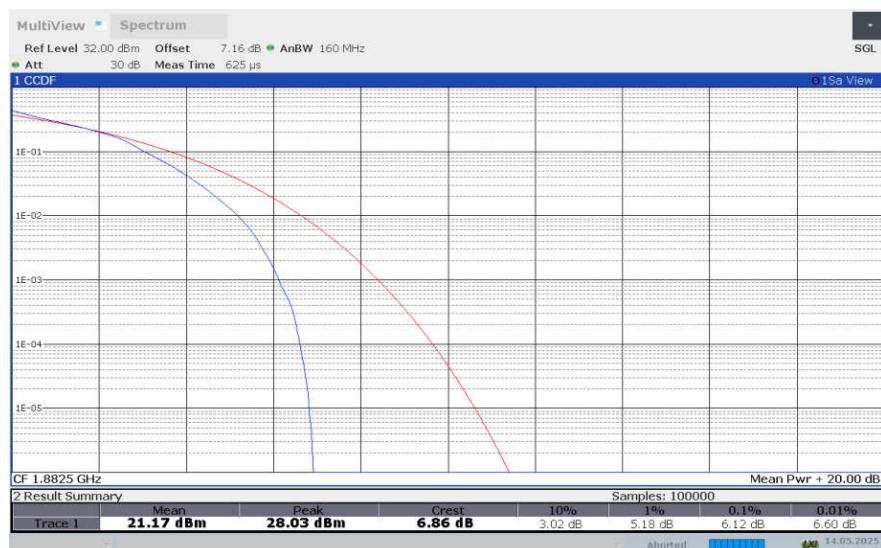
**LTE band 25 , 10MHz Bandwidth,64QAM**
