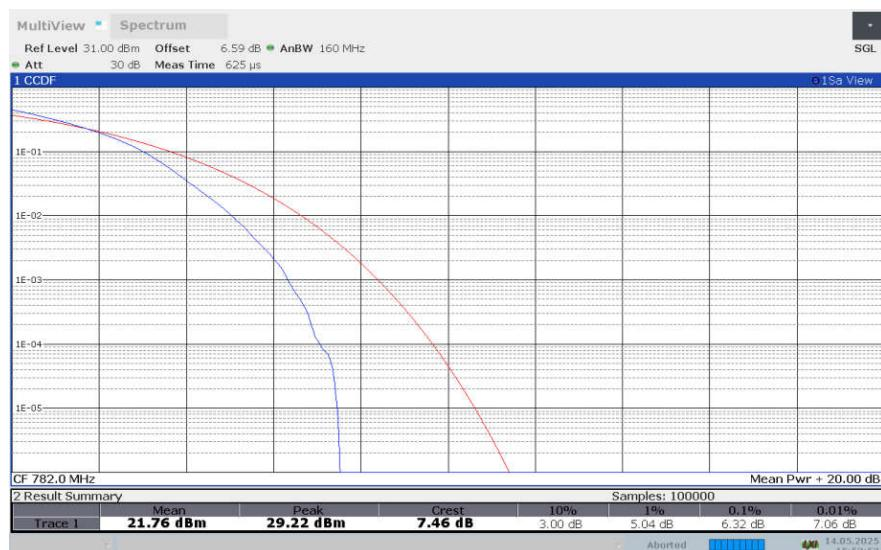
**LTE band 13 , 10MHz Bandwidth,64QAM**
