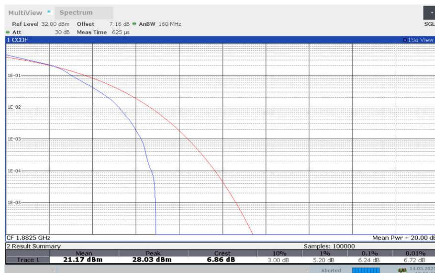
**LTE band 25 , 5MHz Bandwidth,64QAM**
