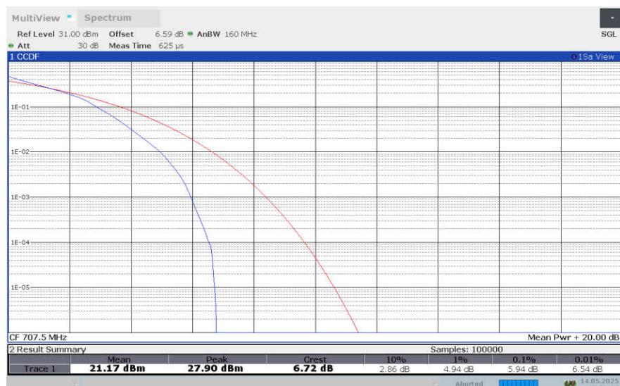
**LTE band 12 , 10MHz Bandwidth,64QAM**
