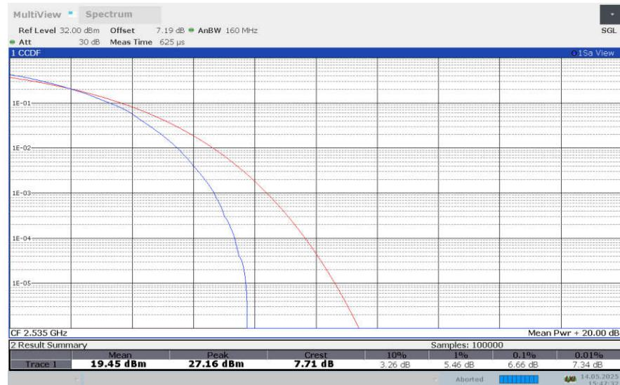
**LTE band 7 , 20MHz Bandwidth,256QAM**
