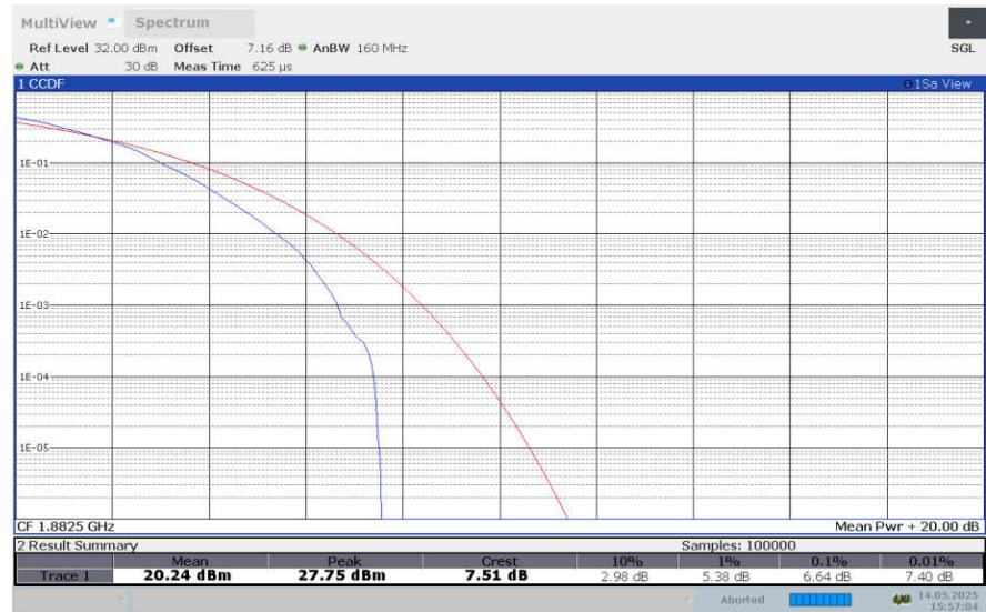
**LTE band 25 , 5MHz Bandwidth,256QAM**
