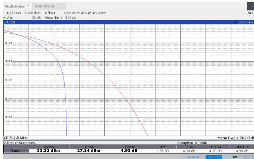
**LTE band 12 , 1.4MHz Bandwidth,16QAM**
