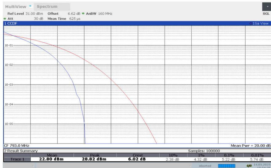
**LTE band 14 , 10MHz Bandwidth,16QAM**
