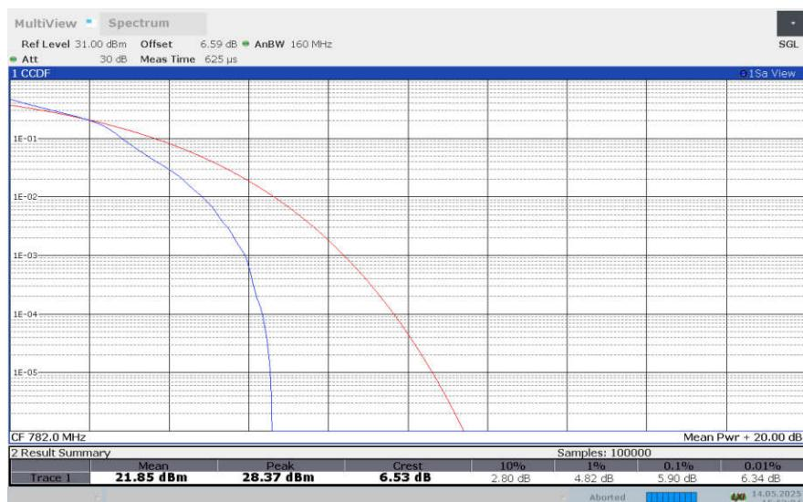
**LTE band 13 , 5MHz Bandwidth,64QAM**
