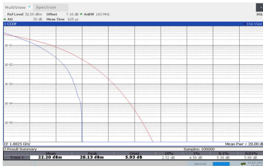
**LTE band 25 , 5MHz Bandwidth,16QAM**
