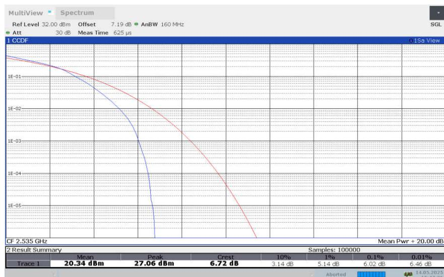
**LTE band 7 , 20MHz Bandwidth,64QAM**
