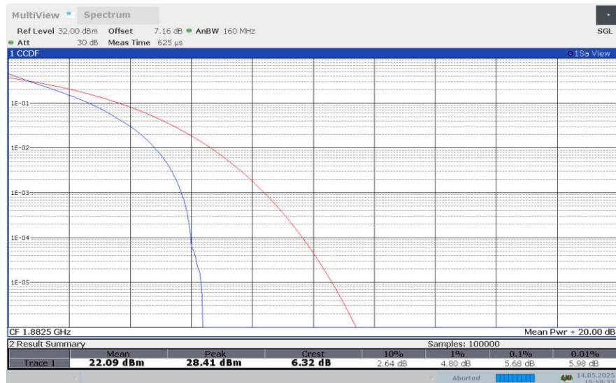
**LTE band 25 , 15MHz Bandwidth,16QAM**
