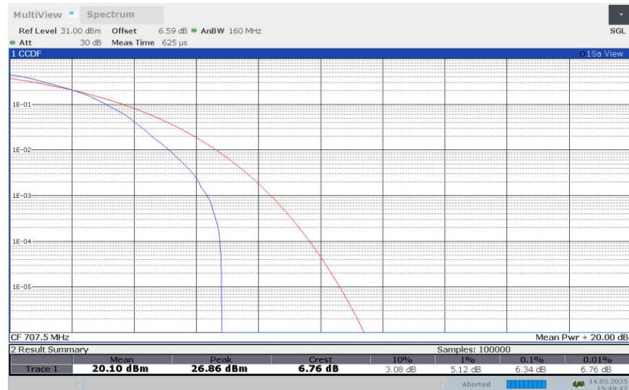
**LTE band 12 , 3MHz Bandwidth,256QAM**
