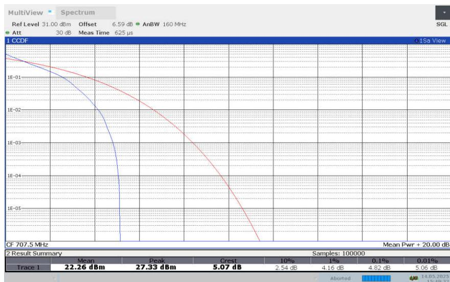
**LTE band 12 , 3MHz Bandwidth,16QAM**
