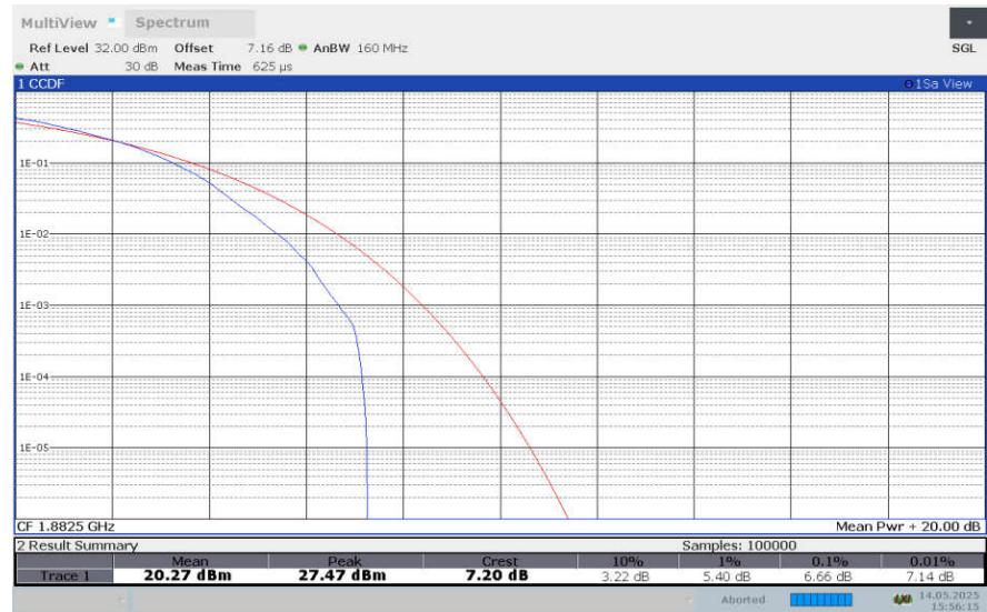
**LTE band 25 , 3MHz Bandwidth,256QAM**
