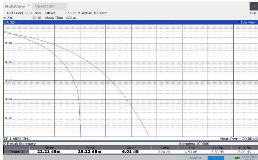
**LTE band 25 , 10MHz Bandwidth,16QAM**
