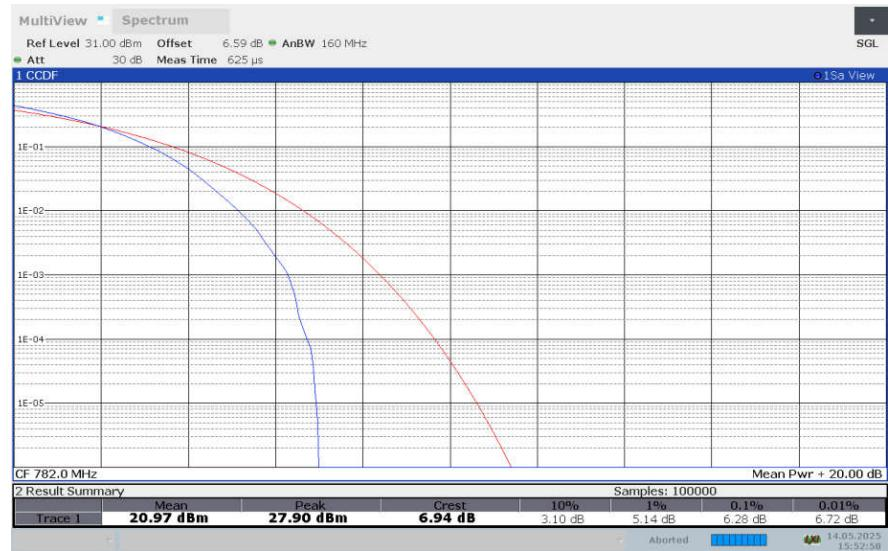
**LTE band 13 , 10MHz Bandwidth,256QAM**
