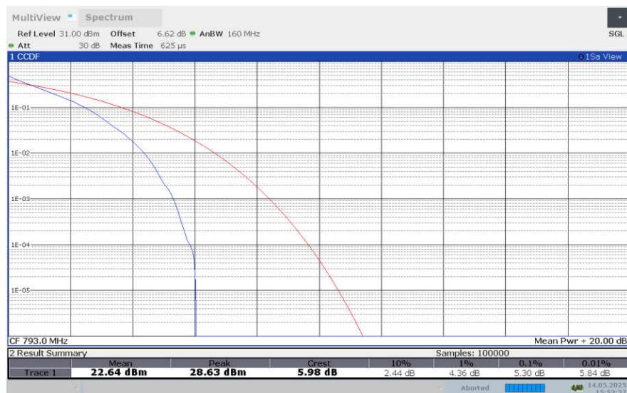
**LTE band 14 , 5MHz Bandwidth,16QAM**
