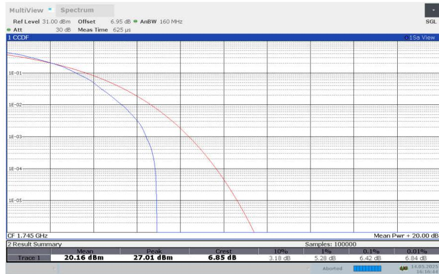
**LTE band 66 , 3MHz Bandwidth,256QAM**
