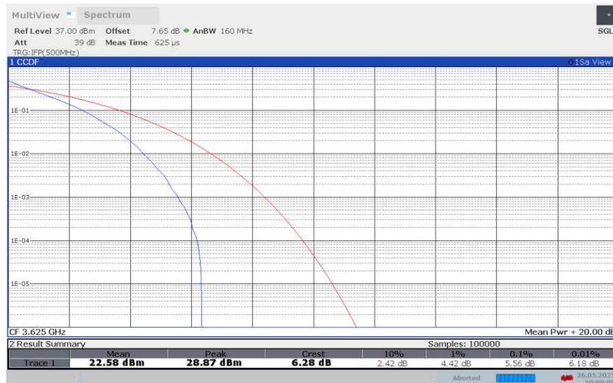
**LTE band 48 , 5MHz Bandwidth,16QAM**
