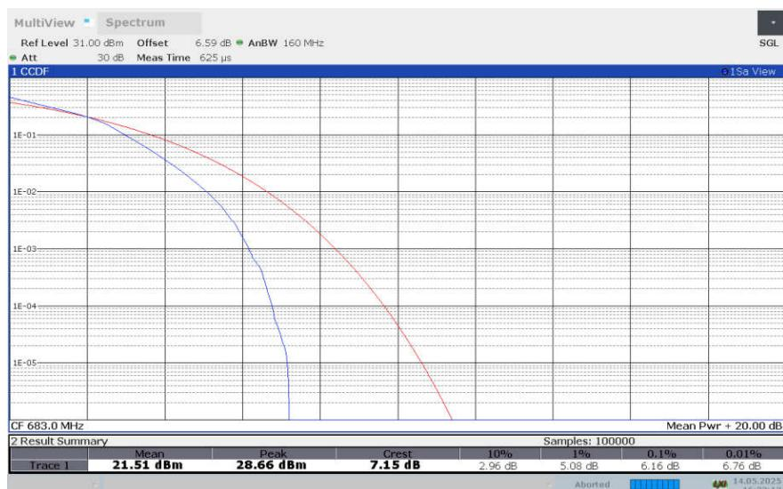
**LTE band 71 , 20MHz Bandwidth,64QAM**
