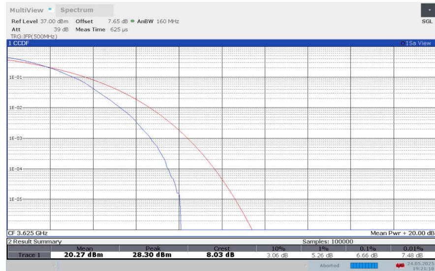
**LTE band 48 , 20MHz Bandwidth,256QAM**
