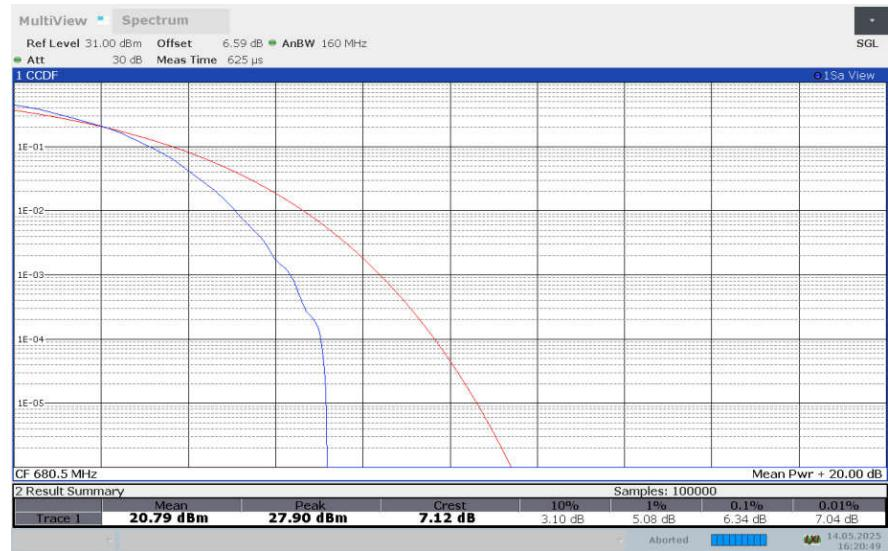
**LTE band 71 , 5MHz Bandwidth,256QAM**
