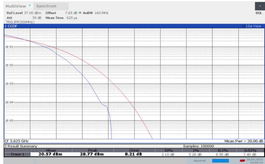
**LTE band 48 , 10MHz Bandwidth,256QAM**
