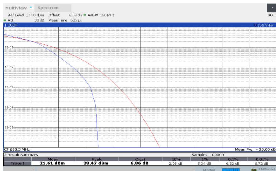
**LTE band 71 , 10MHz Bandwidth,64QAM**
