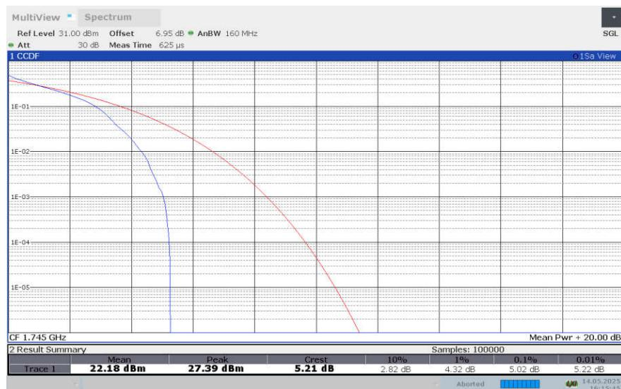
**LTE band 66 , 1.4MHz Bandwidth,16QAM**
