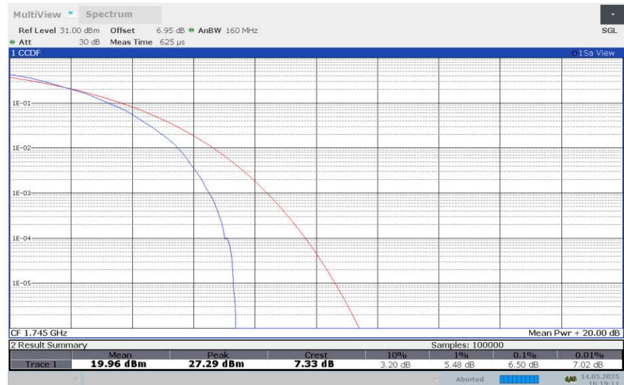
**LTE band 66 , 15MHz Bandwidth,256QAM**
