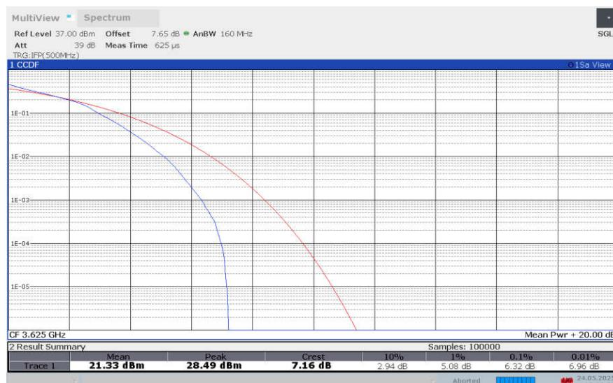
**LTE band 48 , 10MHz Bandwidth,64QAM**
