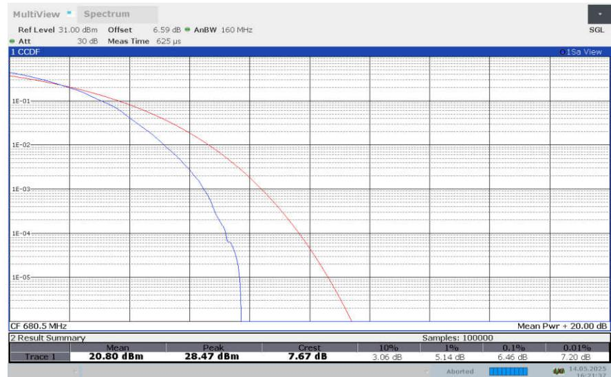
**LTE band 71 , 10MHz Bandwidth,256QAM**
