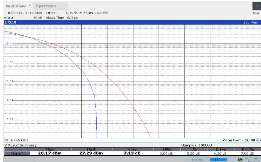
**LTE band 66 , 5MHz Bandwidth,256QAM**
