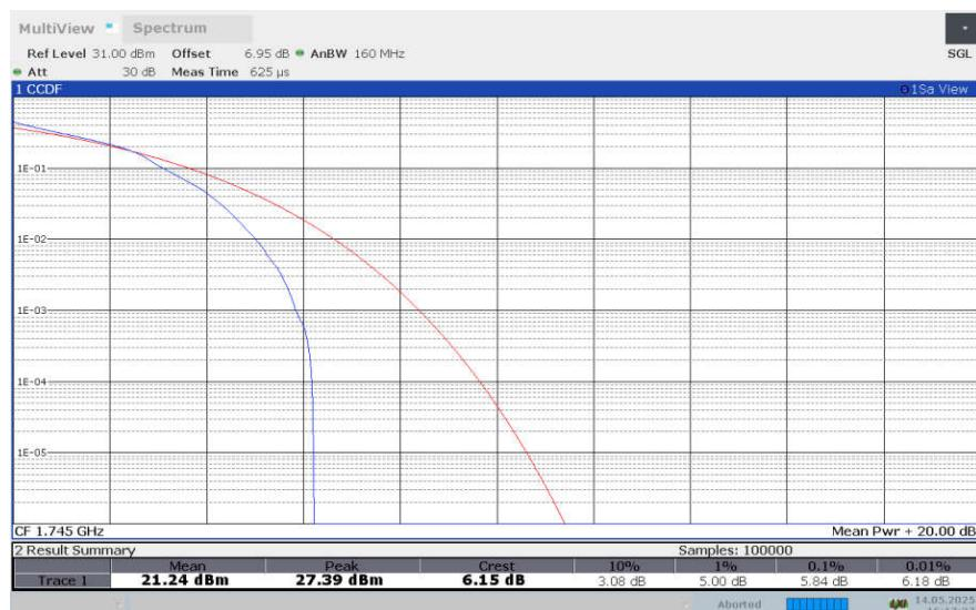
**LTE band 66 , 5MHz Bandwidth,64QAM**
