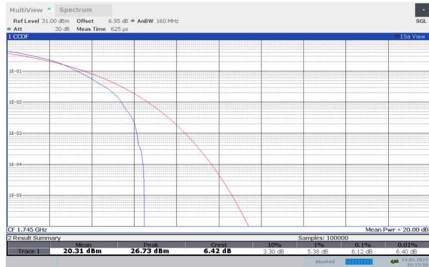
**LTE band 66 , 1.4MHz Bandwidth,256QAM**
