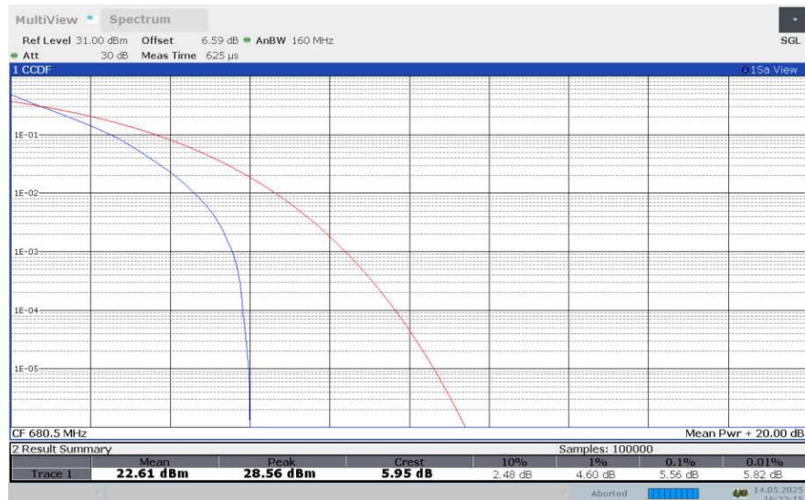
**LTE band 71 , 15MHz Bandwidth,16QAM**
