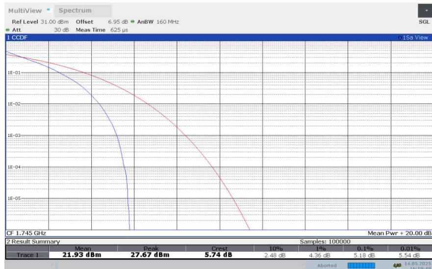
**LTE band 66 , 20MHz Bandwidth,16QAM**
