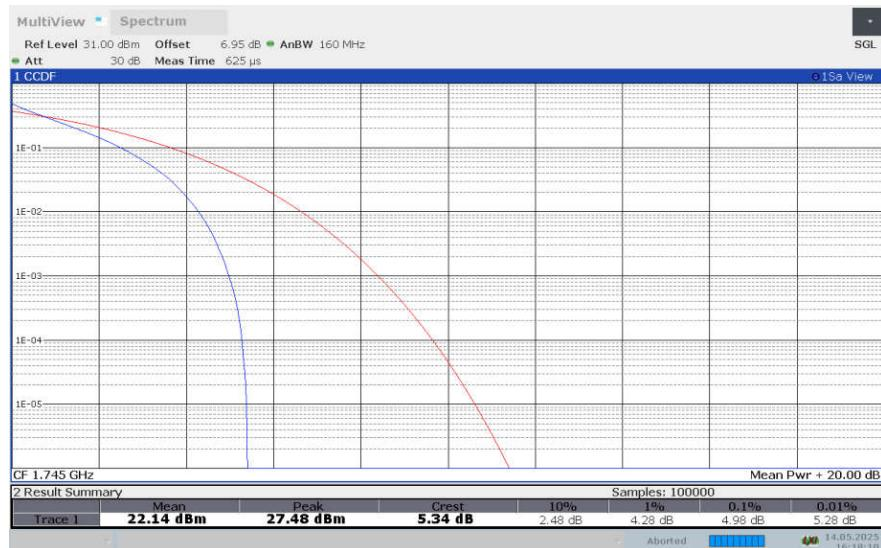
**LTE band 66, 10MHz Bandwidth, 16QAM**
