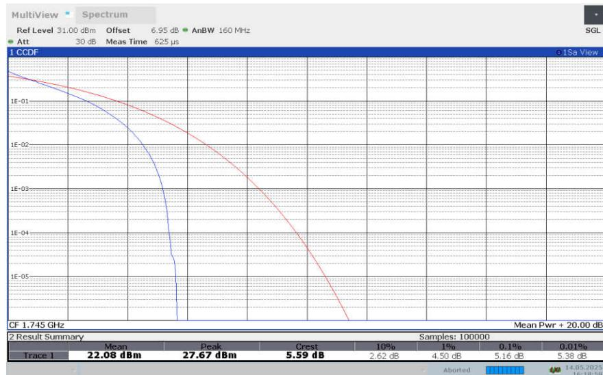
**LTE band 66, 15MHz Bandwidth, 16QAM**
