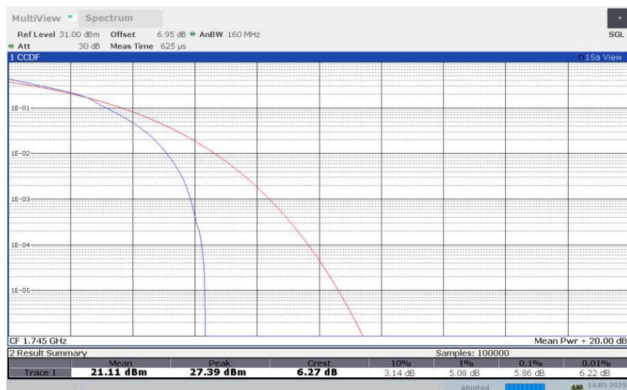
**LTE band 66 , 15MHz Bandwidth,64QAM**
