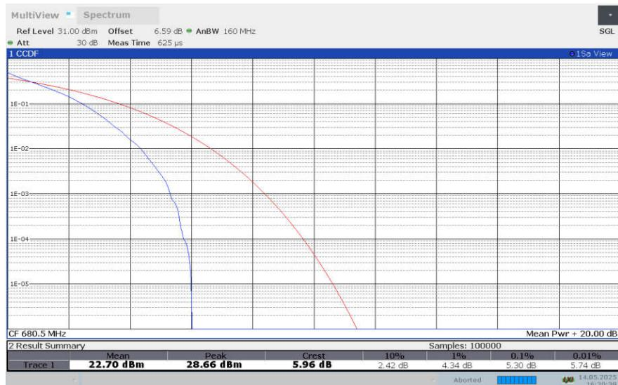
**LTE band 71 , 5MHz Bandwidth,16QAM**
