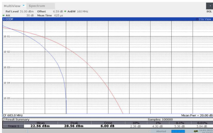
**LTE band 71 , 20MHz Bandwidth,16QAM**
