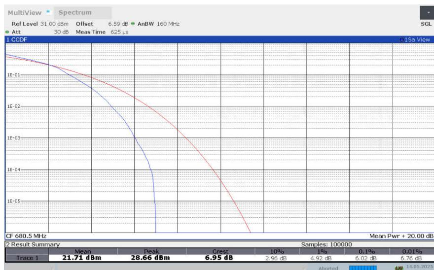
**LTE band 71 , 5MHz Bandwidth,64QAM**
