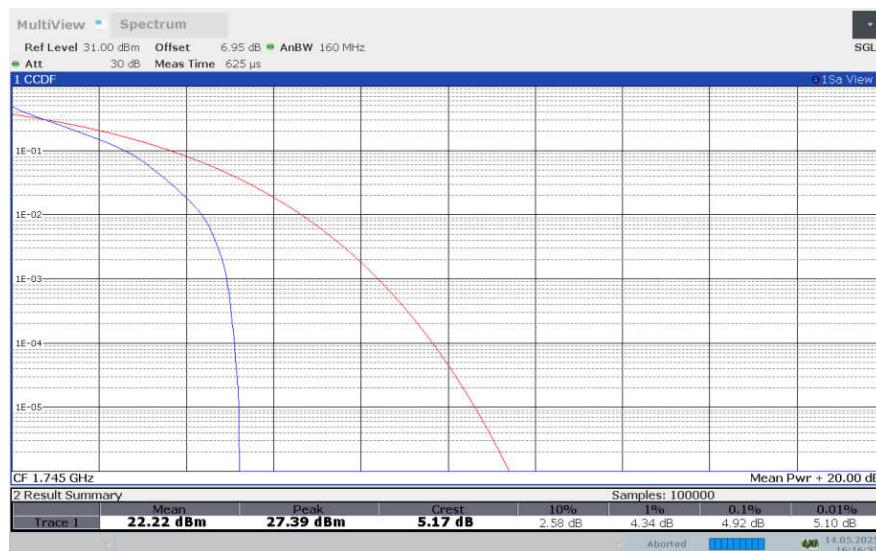
**LTE band 66, 3MHz Bandwidth, 16QAM**
