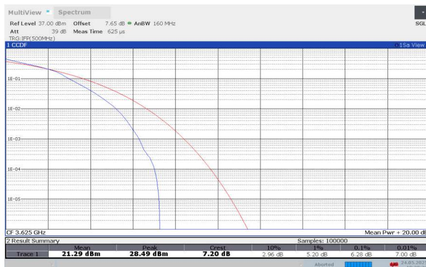
**LTE band 48 , 15MHz Bandwidth,64QAM**
