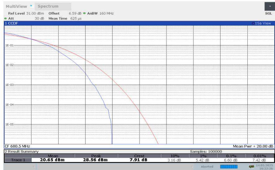
**LTE band 71 , 15MHz Bandwidth,256QAM**
