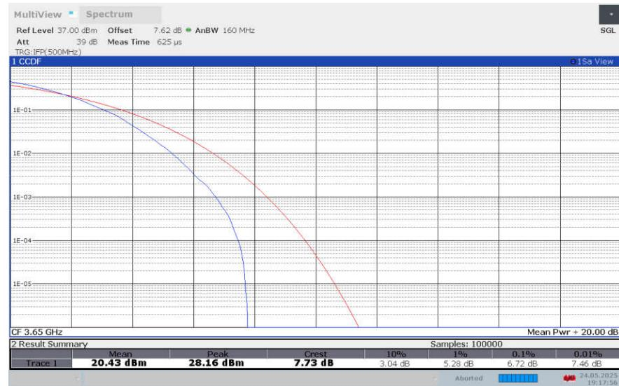
**LTE band 43 , 20MHz Bandwidth,256QAM**
