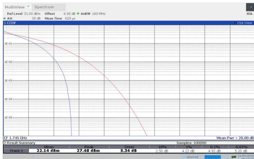
**LTE band 66 , 5MHz Bandwidth,16QAM**
