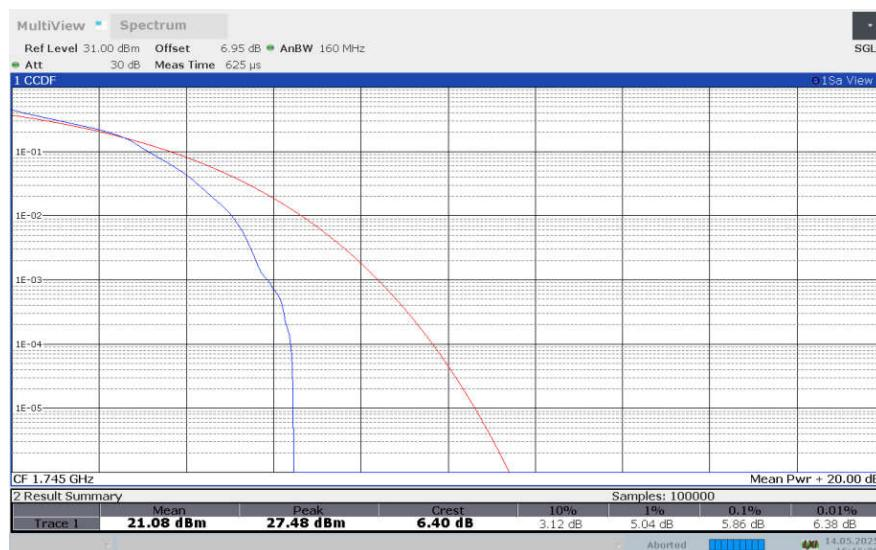
**LTE band 66 , 3MHz Bandwidth,64QAM**
