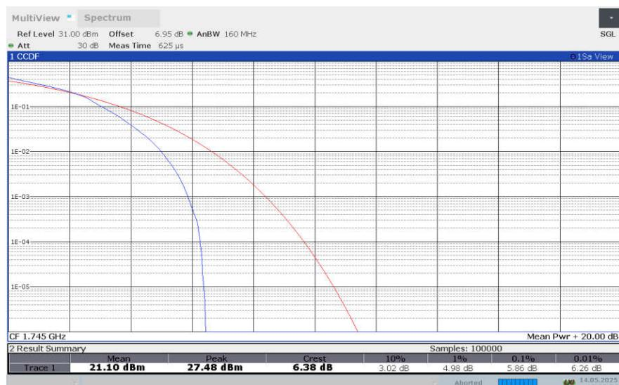
**LTE band 66 , 20MHz Bandwidth,64QAM**
