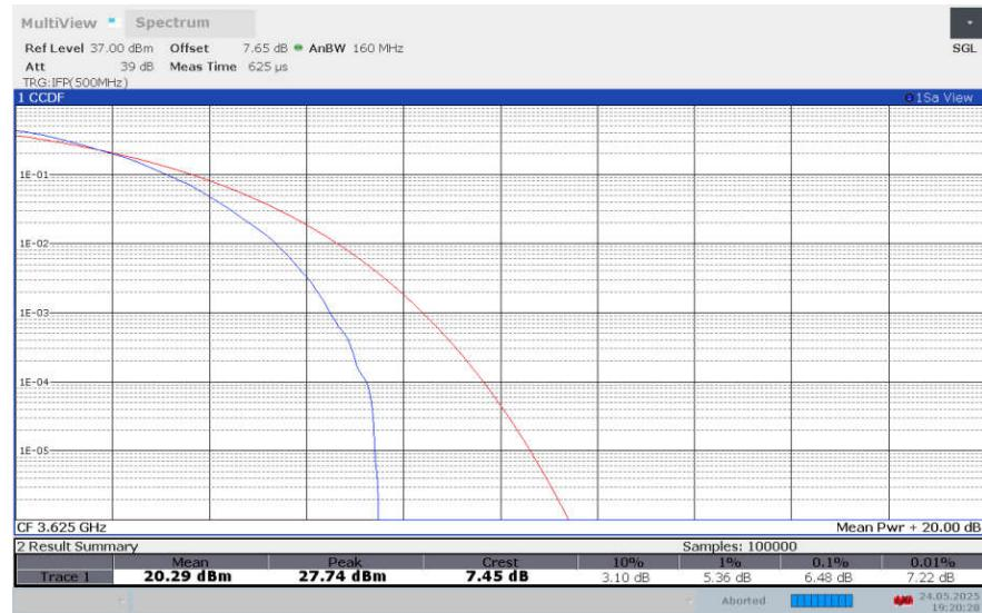
**LTE band 48 , 15MHz Bandwidth,256QAM**
