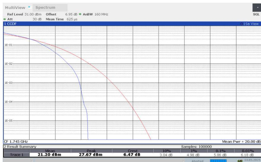
**LTE band 66 , 10MHz Bandwidth,64QAM**
