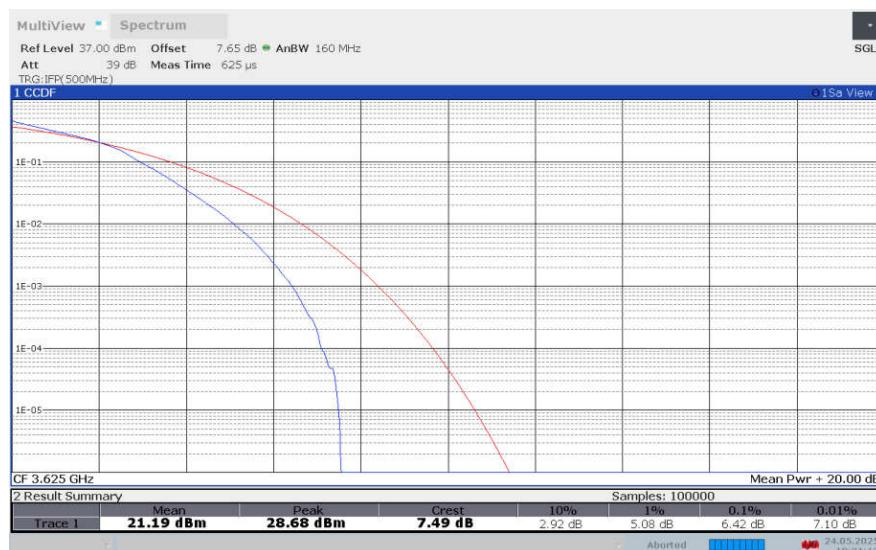
**LTE band 48 , 20MHz Bandwidth,64QAM**
