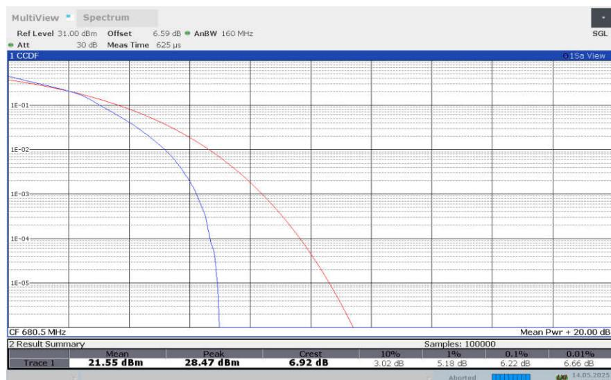
**LTE band 71 , 15MHz Bandwidth,64QAM**
