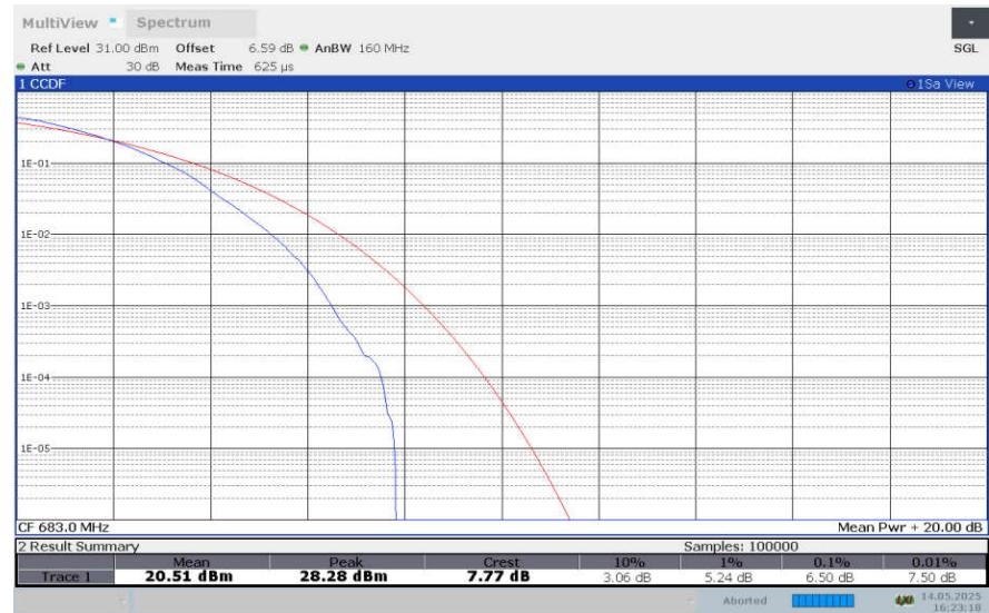
**LTE band 71 , 20MHz Bandwidth,256QAM**
