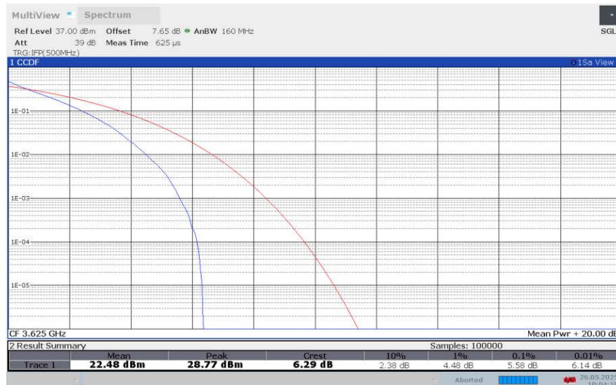
**LTE band 48 , 10MHz Bandwidth,16QAM**
