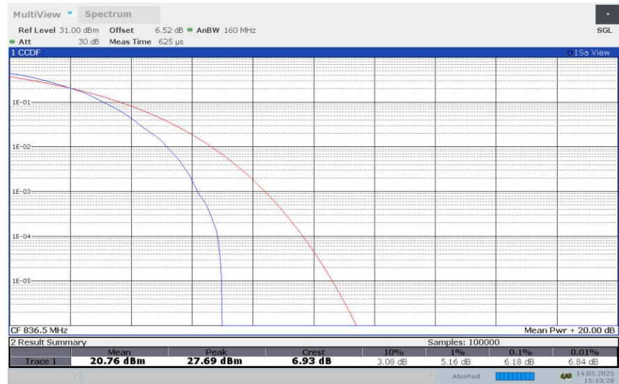
**LTE band 5 , 5MHz Bandwidth,256QAM**
