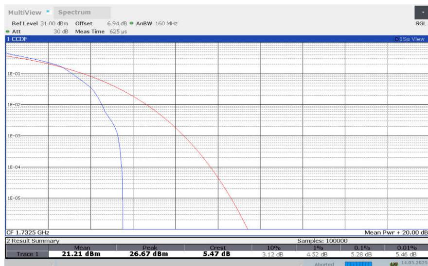
**LTE band 4 , 1.4MHz Bandwidth,64QAM**
