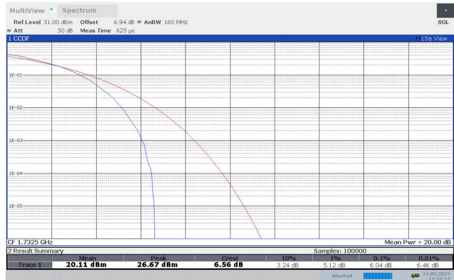
**LTE band 4 , 3MHz Bandwidth,256QAM**
