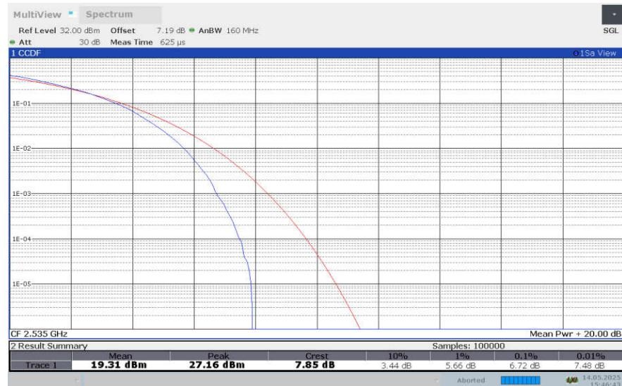
**LTE band 7 , 15MHz Bandwidth,256QAM**
