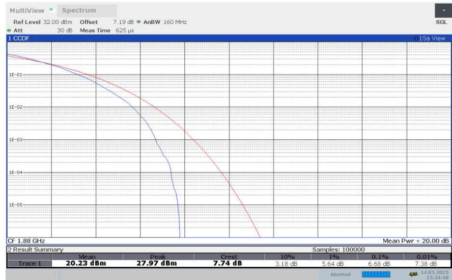
**LTE band 2 , 15MHz Bandwidth,256QAM**
