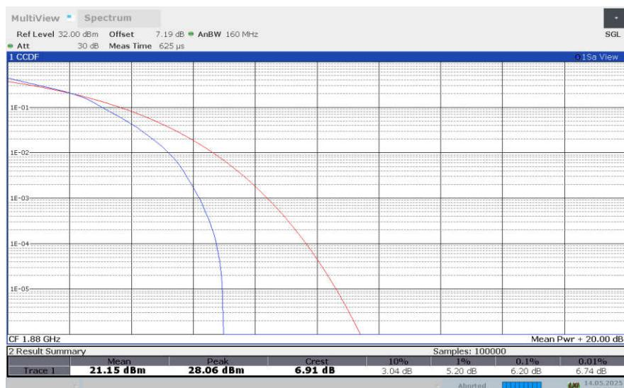
**LTE band 2 , 20MHz Bandwidth,64QAM**
