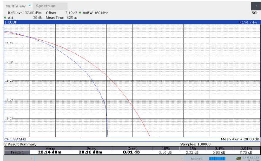
**LTE band 2 , 20MHz Bandwidth,256QAM**
