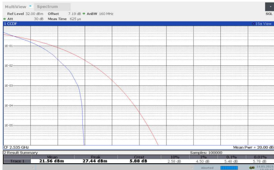
**LTE band 7 , 10MHz Bandwidth,16QAM**
