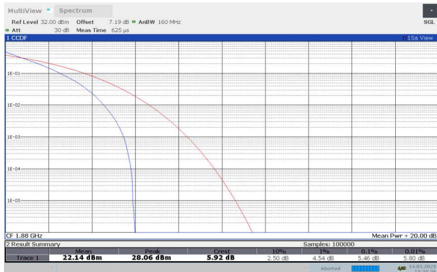
**LTE band 2 , 20MHz Bandwidth,16QAM**
