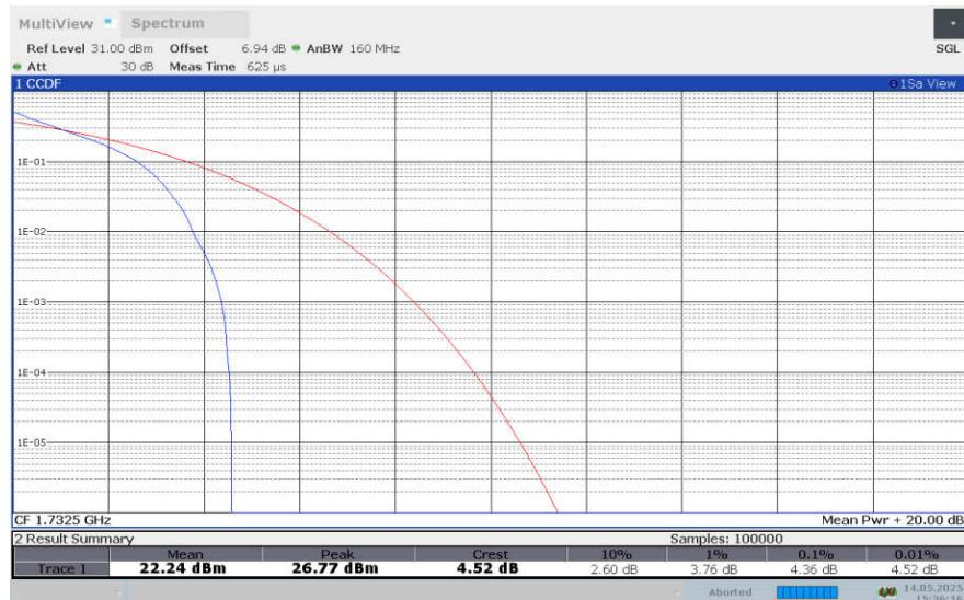
**LTE band 4 , 1.4MHz Bandwidth,16QAM**
