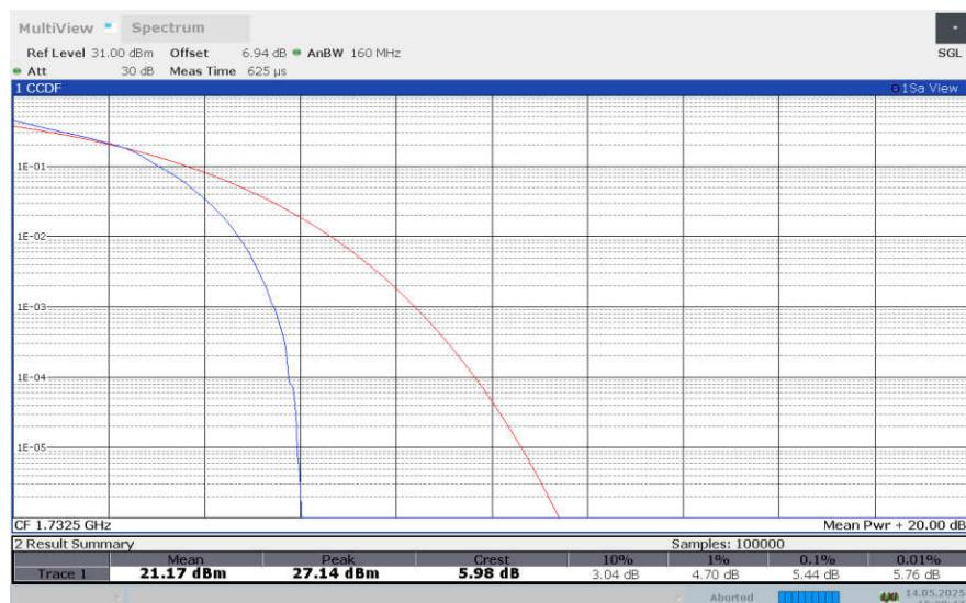
**LTE band 4 , 10MHz Bandwidth,64QAM**
