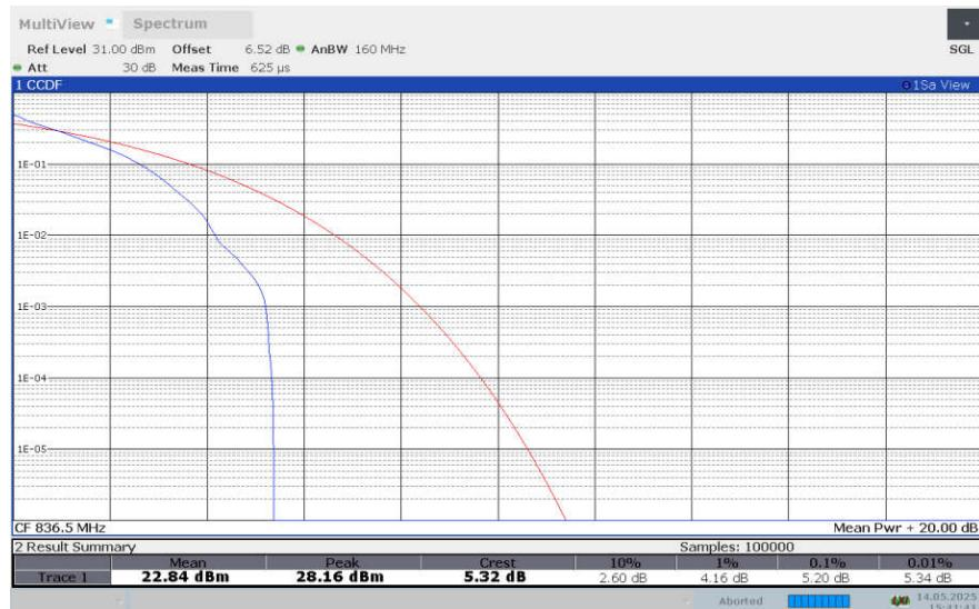
**LTE band 5 , 1.4MHz Bandwidth,16QAM**
