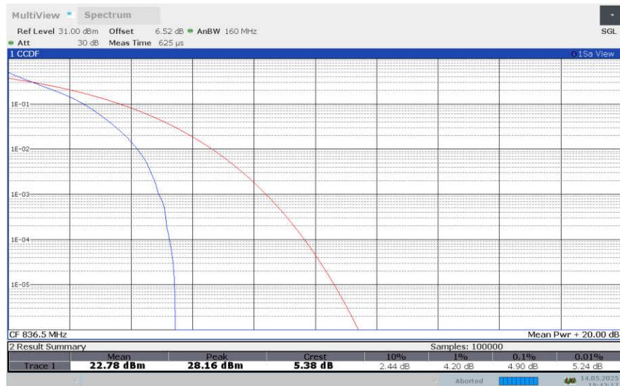
**LTE band 5, 5MHz Bandwidth, 16QAM**
