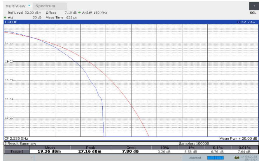
**LTE band 7 , 5MHz Bandwidth,256QAM**
