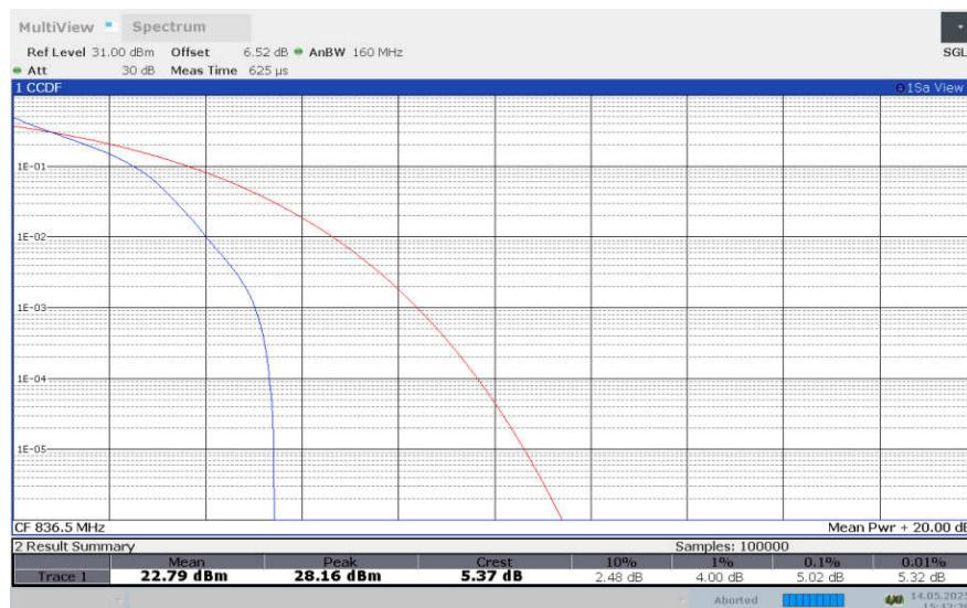
**LTE band 5 , 3MHz Bandwidth,16QAM**
