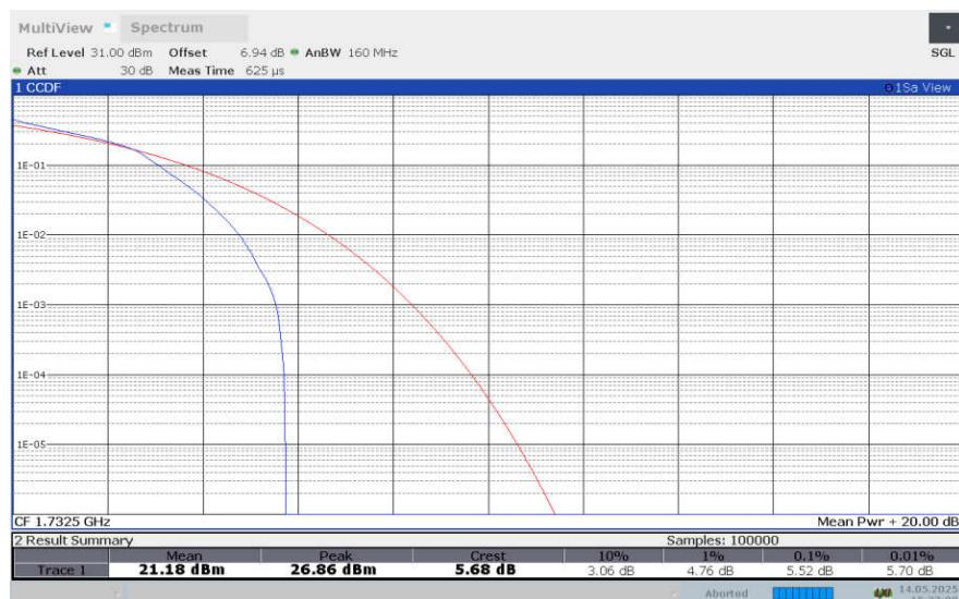
**LTE band 4 , 3MHz Bandwidth,64QAM**
