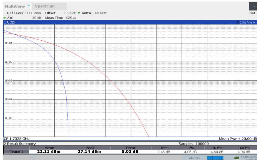
**LTE band 4 , 20MHz Bandwidth,16QAM**
