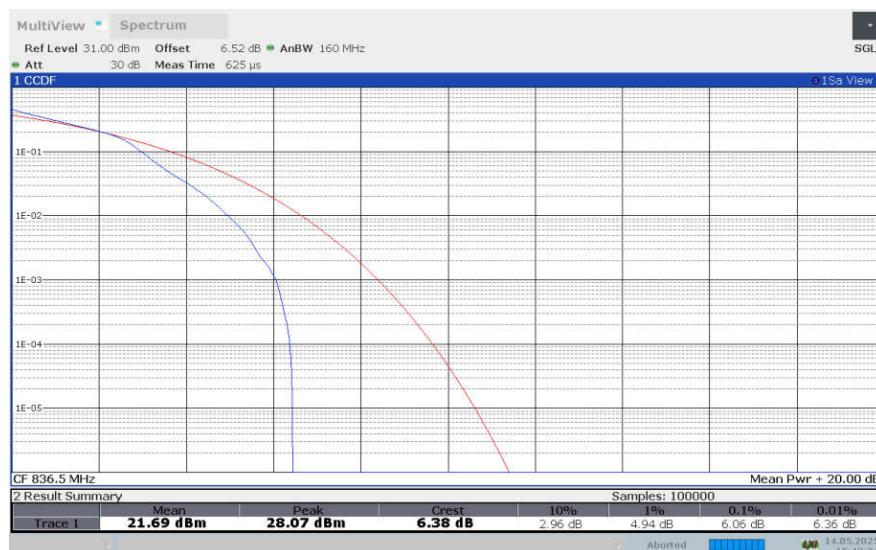
**LTE band 5 , 3MHz Bandwidth,64QAM**
