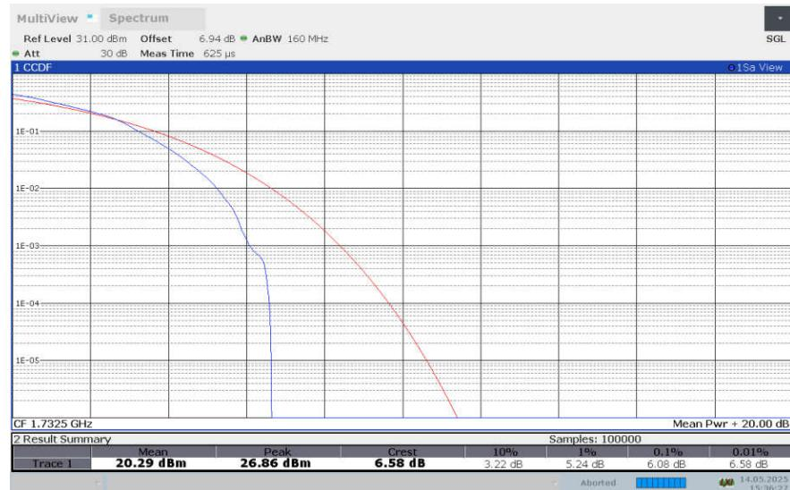
**LTE band 4 , 1.4MHz Bandwidth,256QAM**
