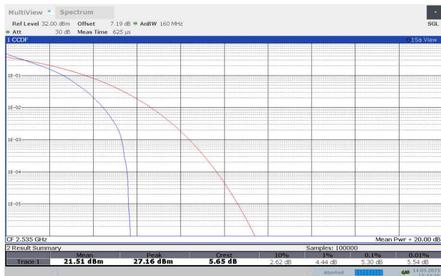
**LTE band 7, 5MHz Bandwidth, 16QAM**
