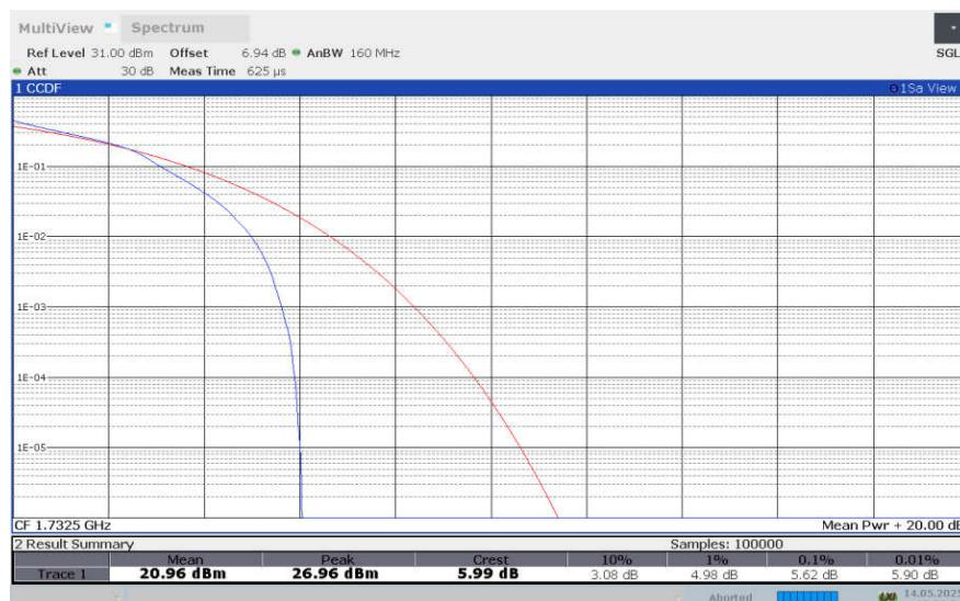
**LTE band 4 , 15MHz Bandwidth,64QAM**
