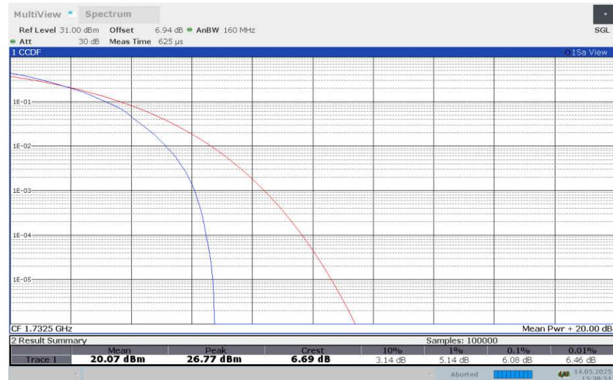
**LTE band 4 , 10MHz Bandwidth,256QAM**
