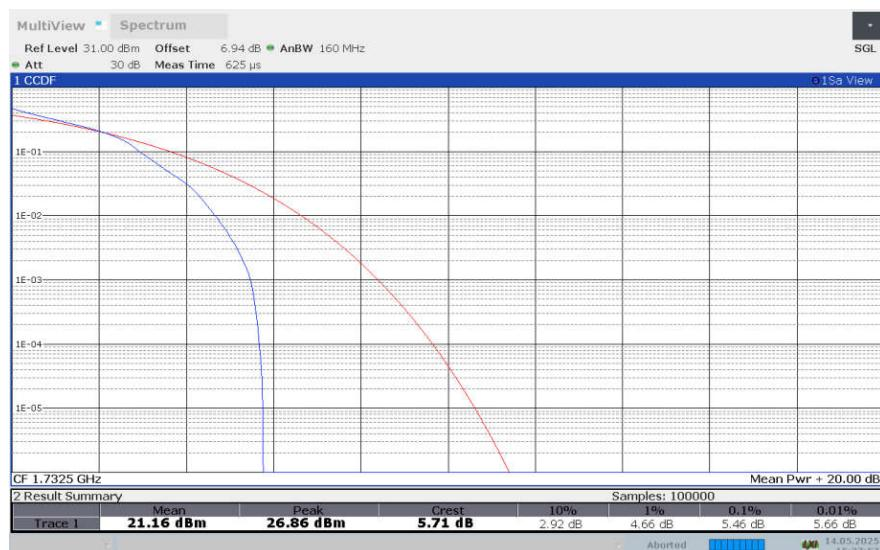
**LTE band 4 , 5MHz Bandwidth,64QAM**
