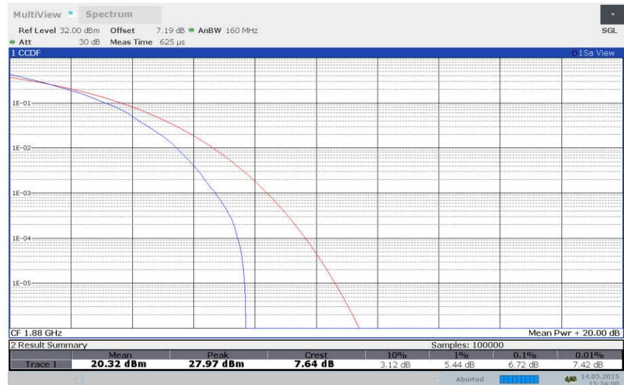
**LTE band 2 , 10MHz Bandwidth,256QAM**
