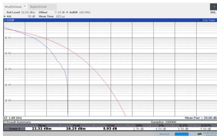
**LTE band 2 , 1.4MHz Bandwidth,16QAM**
