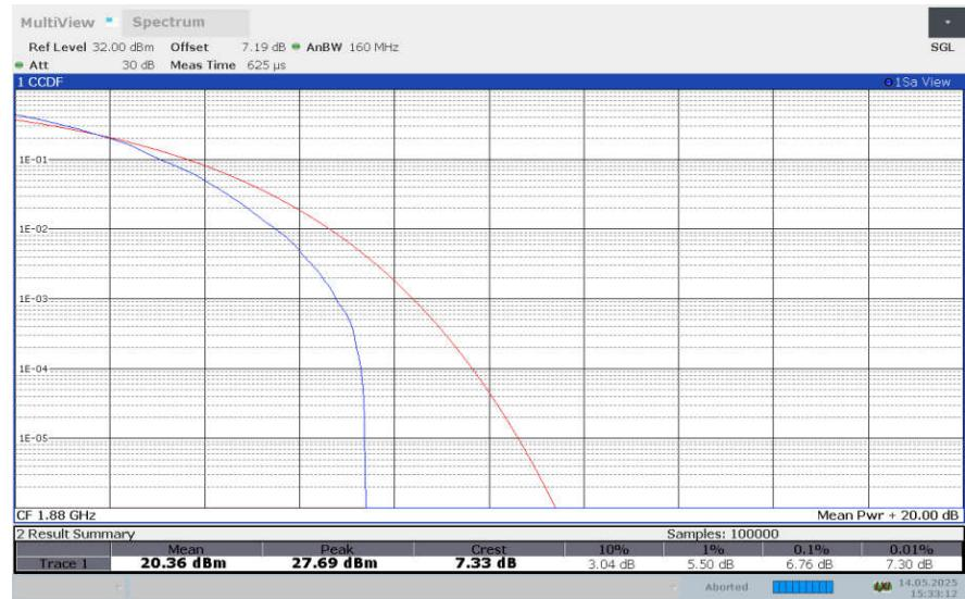
**LTE band 2 , 5MHz Bandwidth,256QAM**
