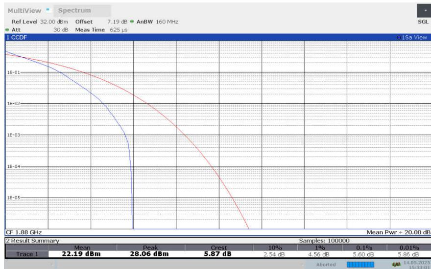
**LTE band 2, 5MHz Bandwidth, 16QAM**
