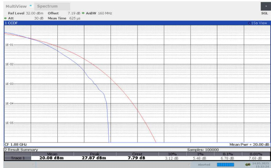
**LTE band 2 , 3MHz Bandwidth,256QAM**
