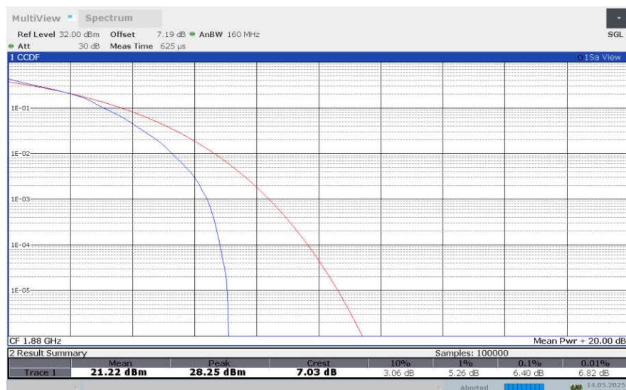
**LTE band 2 , 10MHz Bandwidth,64QAM**
