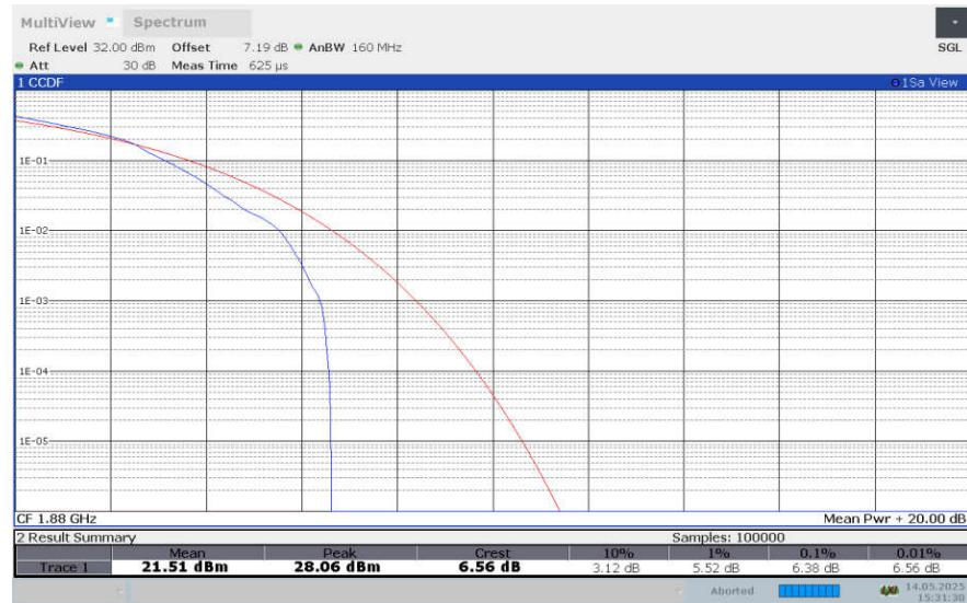
**LTE band 2 , 1.4MHz Bandwidth,64QAM**
