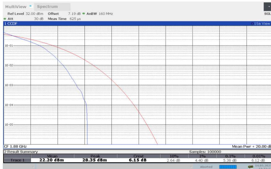
**LTE band 2, 3MHz Bandwidth, 16QAM**
