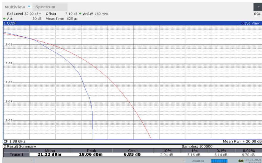
**LTE band 2 , 5MHz Bandwidth,64QAM**
