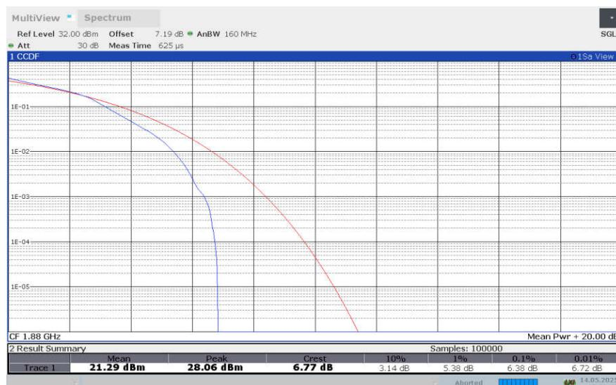
**LTE band 2 , 3MHz Bandwidth,64QAM**
