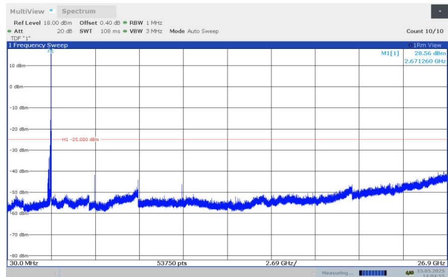
**LTE band 42\_Part27****NOTE: peak above the limit line is the carrier frequency.**
