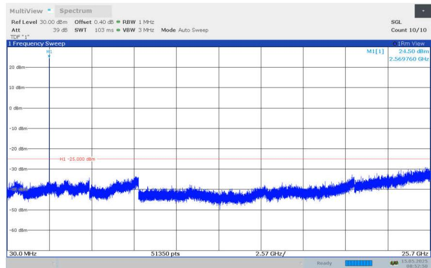
**LTE band 12****NOTE: peak above the limit line is the carrier frequency.**
