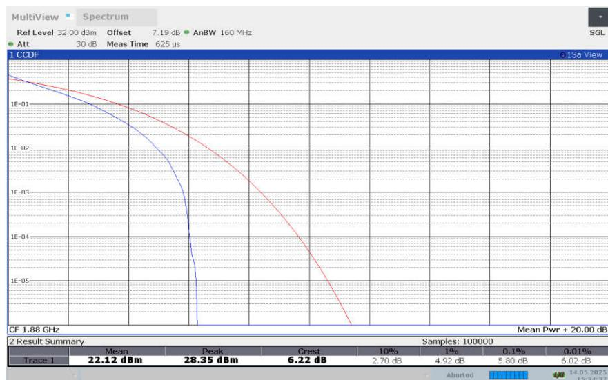
**LTE band 2 , 15MHz Bandwidth,16QAM**
