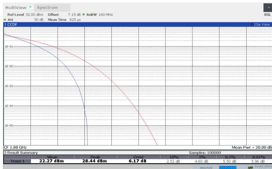
**LTE band 2 , 10MHz Bandwidth,16QAM**
