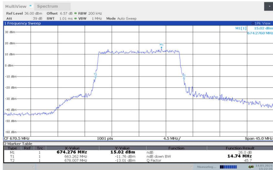
**LTE band 71 , 15MHz Bandwidth,LOW,64QAM (-26dBc BW)**
