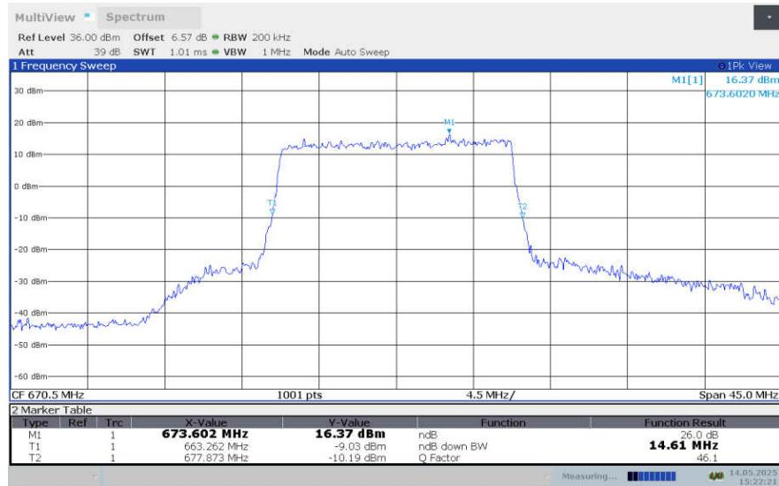
**LTE band 71 , 15MHz Bandwidth,LOW,16QAM (-26dBc BW)**
