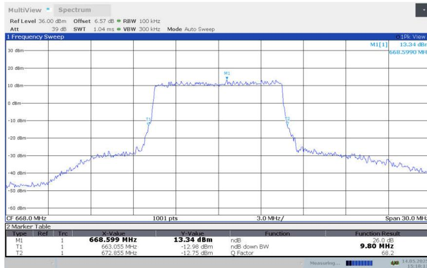
**LTE band 71 , 10MHz Bandwidth,LOW,64QAM (-26dBc BW)**
