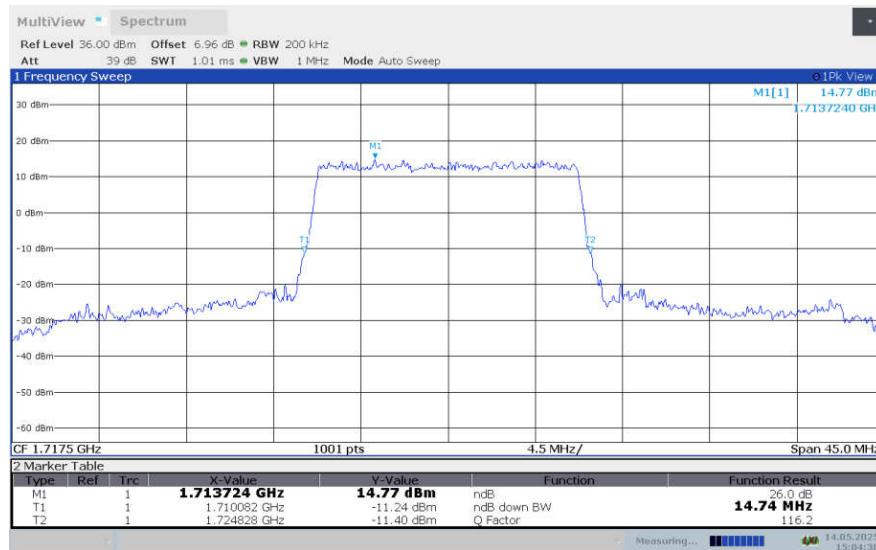
**LTE band 66 , 15MHz Bandwidth,LOW,16QAM (-26dBc BW)**
