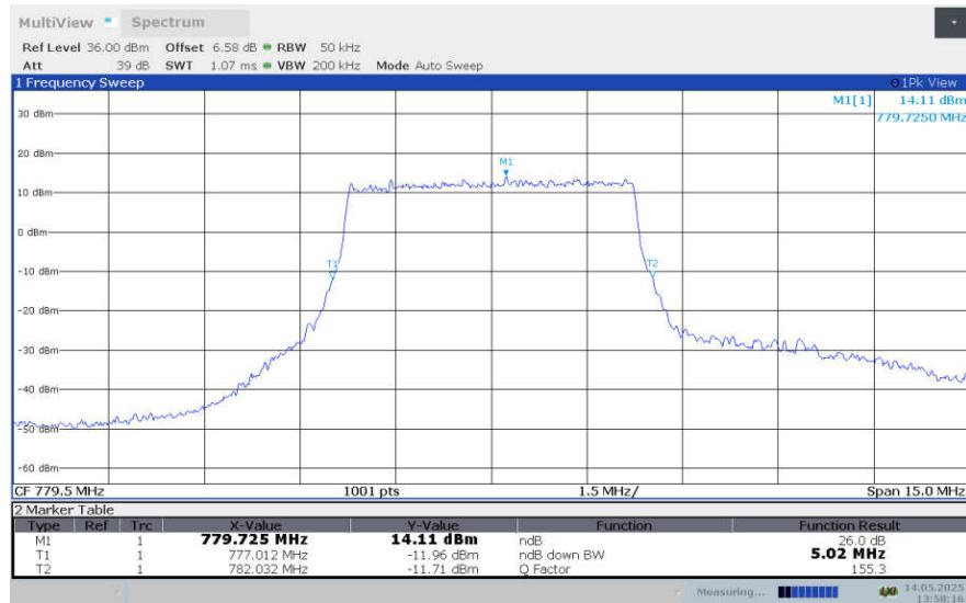
**LTE band 13, 5MHz Bandwidth,LOW,64QAM (-26dBc BW)**
