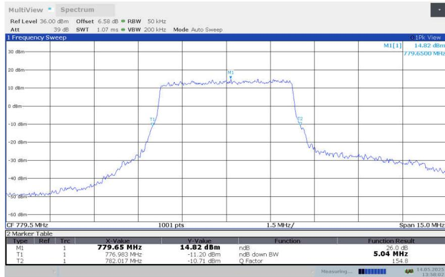
**LTE band 13, 5MHz Bandwidth,LOW,16QAM (-26dBc BW)**
