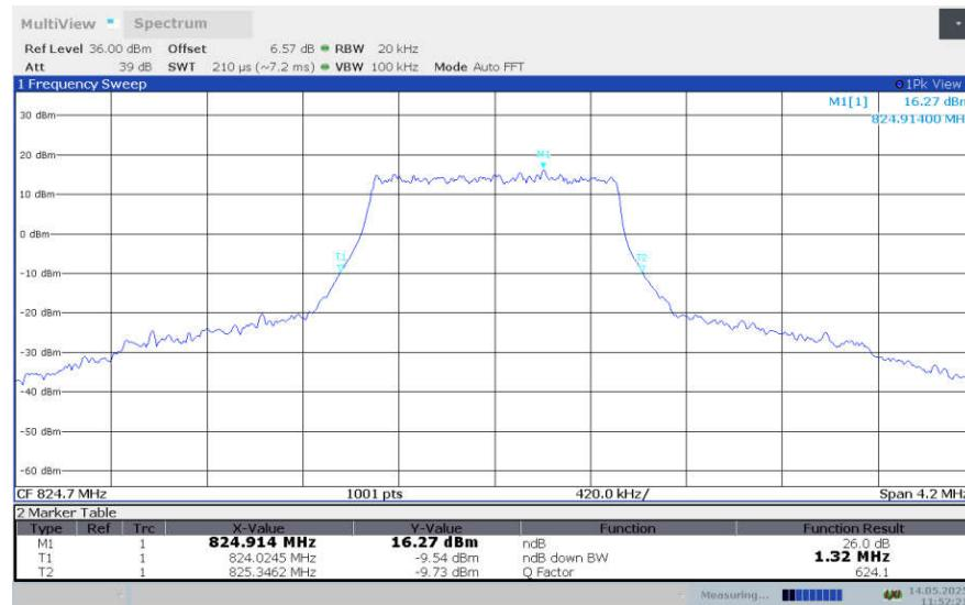
**LTE band 5 , 1.4MHz Bandwidth,LOW,16QAM (-26dBc BW)**
