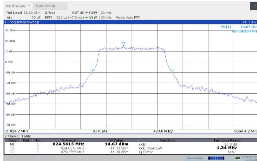
**LTE band 5 , 1.4MHz Bandwidth,LOW,64QAM (-26dBc BW)**
