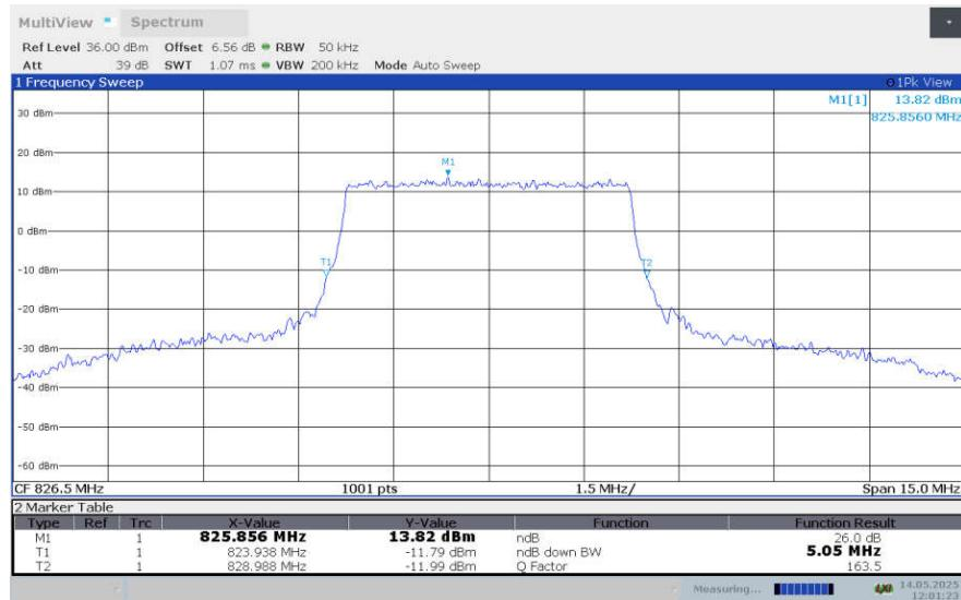
**LTE band 5 , 5MHz Bandwidth,LOW,64QAM (-26dBc BW)**
