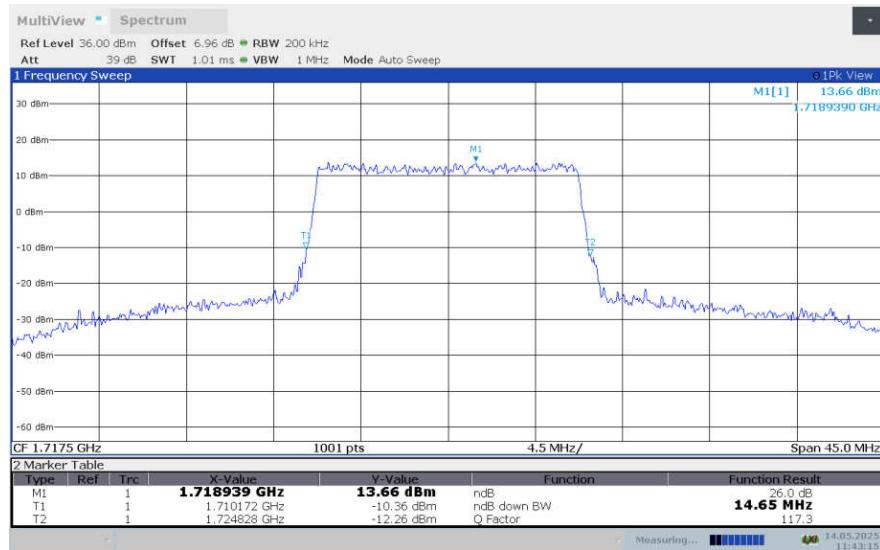
**LTE band 4, 15MHz Bandwidth,LOW,64QAM (-26dBc BW)**
