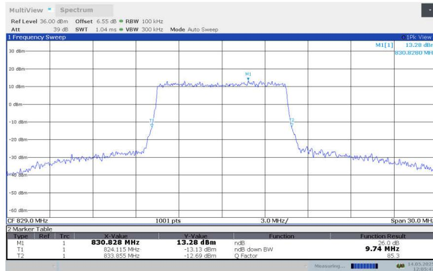
**LTE band 5 , 10MHz Bandwidth,LOW,64QAM (-26dBc BW)**
