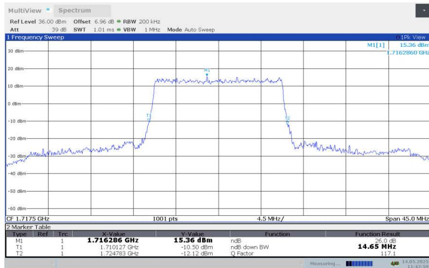
**LTE band 4, 15MHz Bandwidth,LOW,16QAM (-26dBc BW)**
