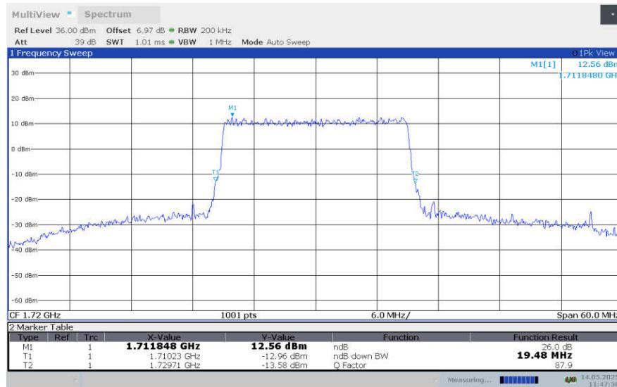
**LTE band 4 , 20MHz Bandwidth,LOW,64QAM (-26dBc BW)**
