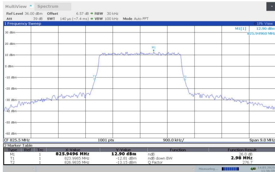
**LTE band 5 , 3MHz Bandwidth,LOW,64QAM (-26dBc BW)**
