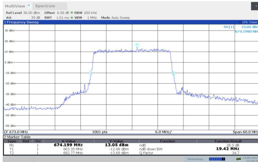
**LTE band 71 , 20MHz Bandwidth,LOW,64QAM (-26dBc BW)**
