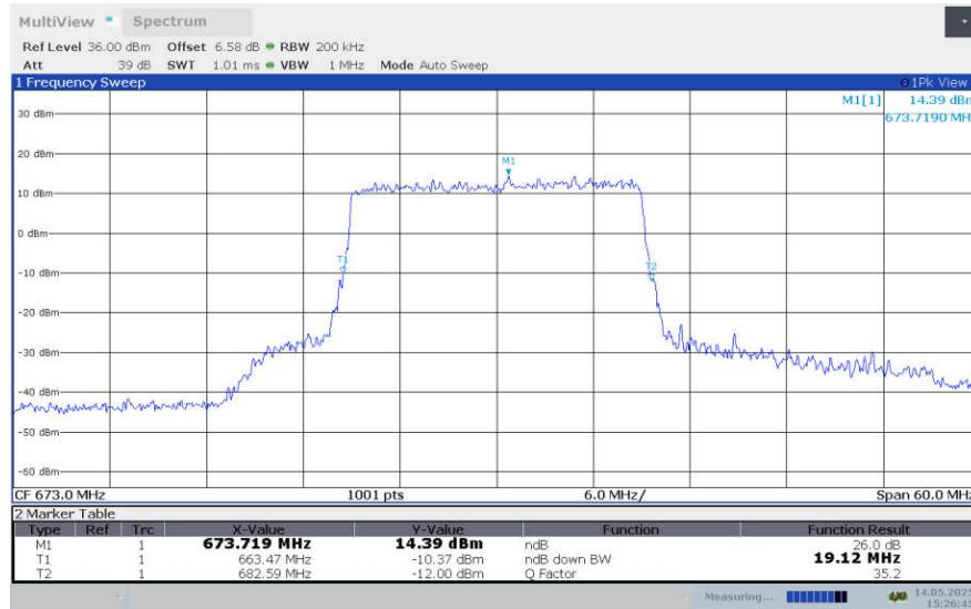
**LTE band 71 , 20MHz Bandwidth,LOW,16QAM (-26dBc BW)**
