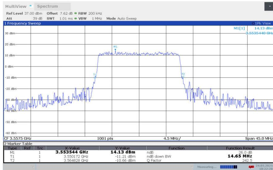
**LTE band 48 , 15MHz Bandwidth,LOW,64QAM (-26dBc BW)**
