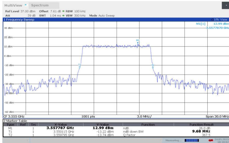
**LTE band 48 , 10MHz Bandwidth,LOW,64QAM (-26dBc BW)**
