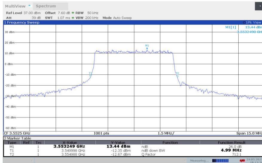
**LTE band 48 , 5MHz Bandwidth,LOW,64QAM (-26dBc BW)**
