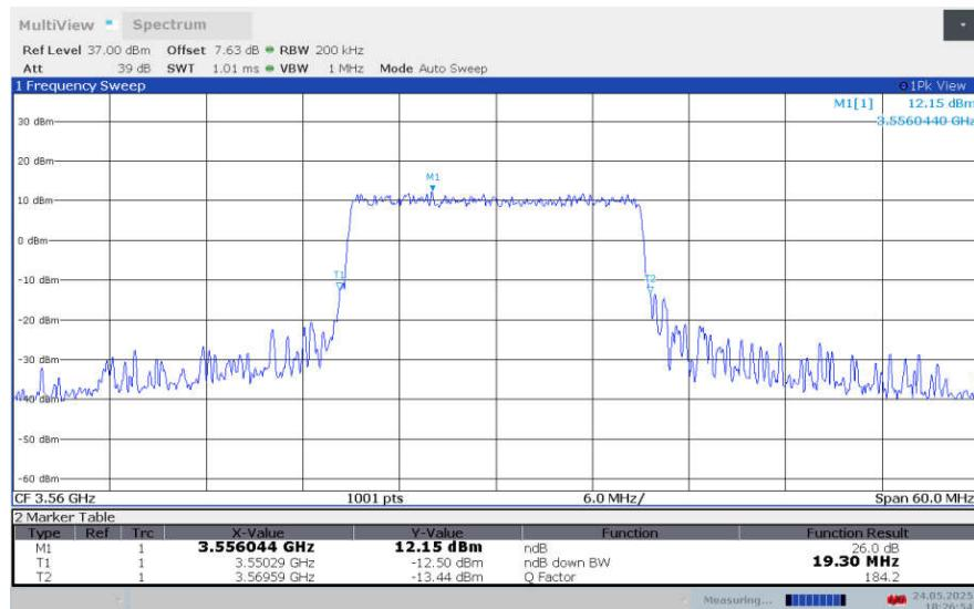
**LTE band 48 , 20MHz Bandwidth,LOW,64QAM (-26dBc BW)**
