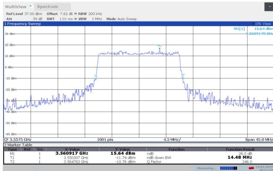
**LTE band 48 , 15MHz Bandwidth,LOW,16QAM (-26dBc BW)**
