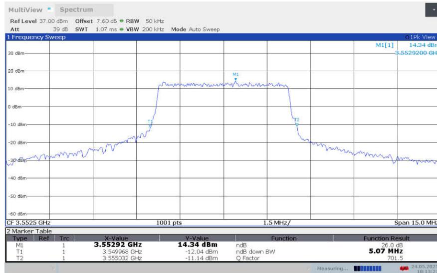
**LTE band 48 , 5MHz Bandwidth,LOW,16QAM (-26dBc BW)**
