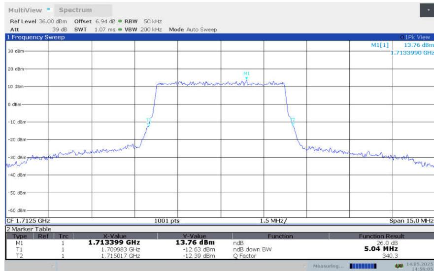
**LTE band 66 , 5MHz Bandwidth,LOW,64QAM (-26dBc BW)**
