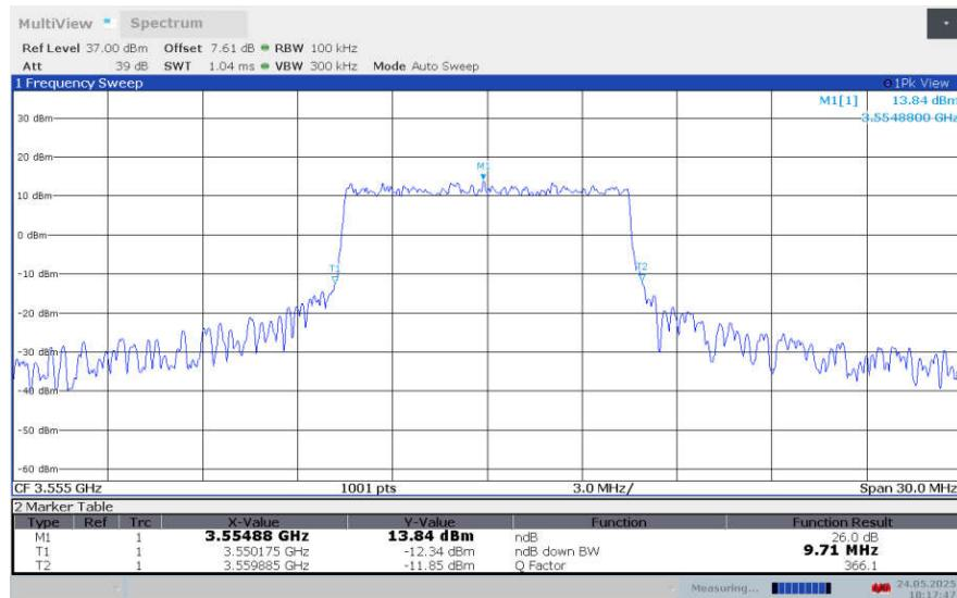
**LTE band 48 , 10MHz Bandwidth,LOW,16QAM (-26dBc BW)**
