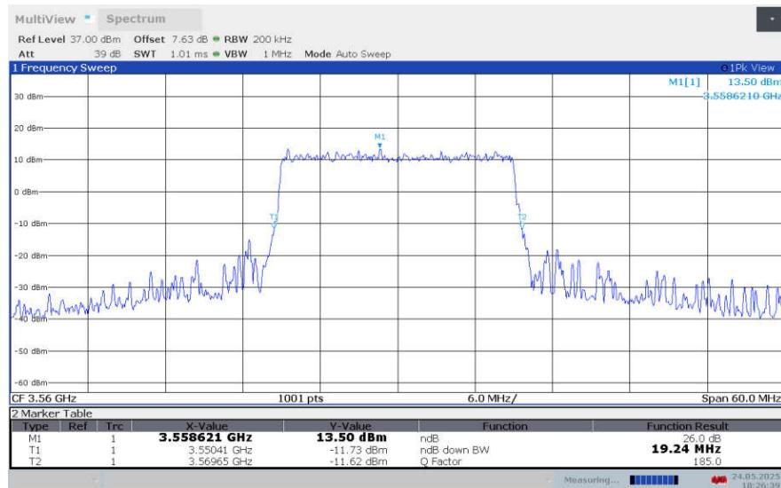
**LTE band 48 , 20MHz Bandwidth,LOW,16QAM (-26dBc BW)**
