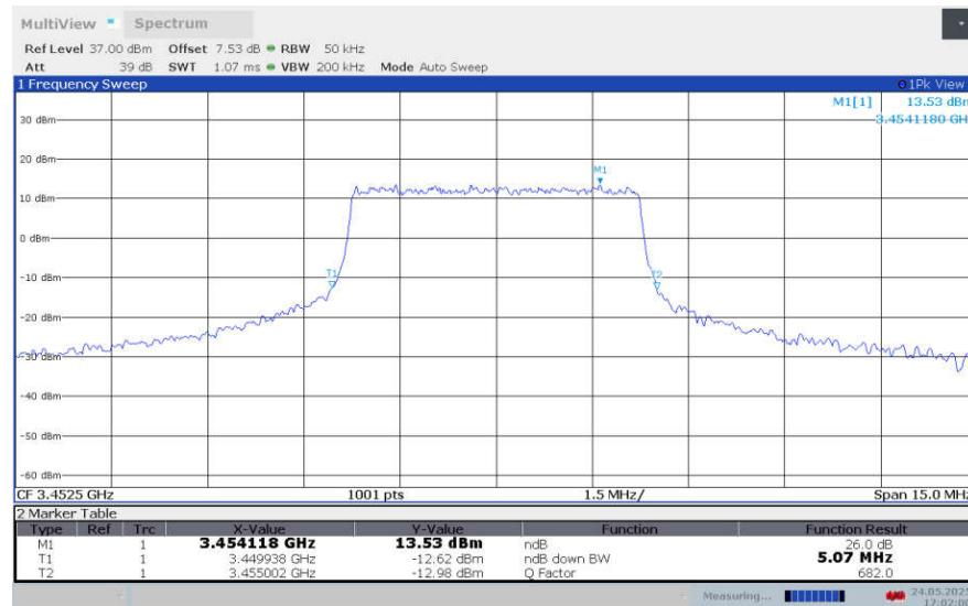
**LTE band 42 , 5MHz Bandwidth,LOW,16QAM (-26dBc BW)**
