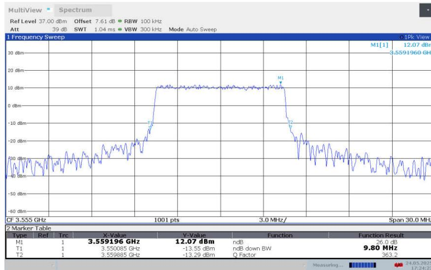
**LTE band 42 , 10MHz Bandwidth,LOW,64QAM (-26dBc BW)**
