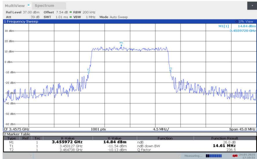
**LTE band 42 , 15MHz Bandwidth,LOW,16QAM (-26dBc BW)**
