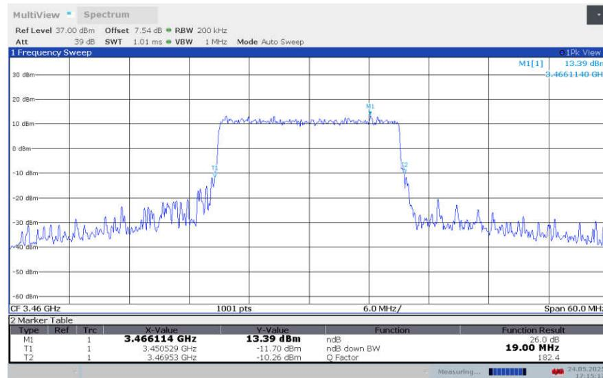
**LTE band 42 , 20MHz Bandwidth,LOW,16QAM (-26dBc BW)**
