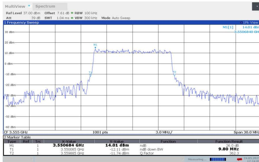
**LTE band 42 , 10MHz Bandwidth,LOW,16QAM (-26dBc BW)**
