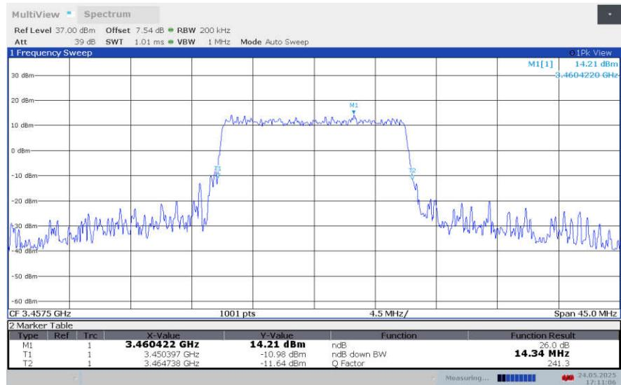
**LTE band 42 , 15MHz Bandwidth,LOW,64QAM (-26dBc BW)**
