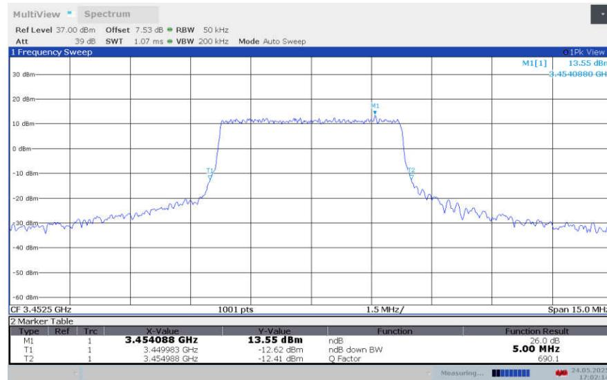
**LTE band 42 , 5MHz Bandwidth,LOW,64QAM (-26dBc BW)**
