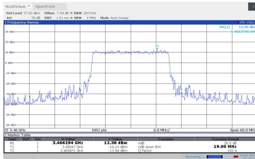
**LTE band 42 , 20MHz Bandwidth,LOW,64QAM (-26dBc BW)**
