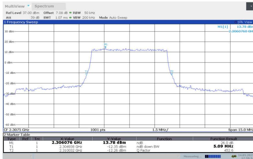
**LTE band 30 , 5MHz Bandwidth,LOW,16QAM (-26dBc BW)**
