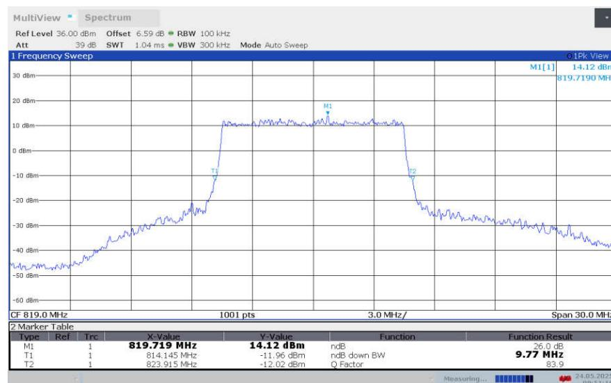
**LTE band 26 , 10MHz Bandwidth,LOW,64QAM (-26dBc BW)**
