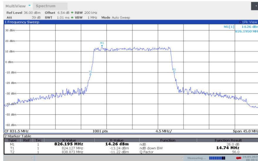
**LTE band 26 , 15MHz Bandwidth,LOW,64QAM (-26dBc BW)**
