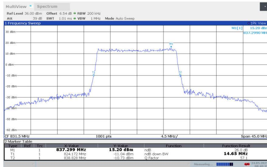
**LTE band 26 , 15MHz Bandwidth,LOW,16QAM (-26dBc BW)**
