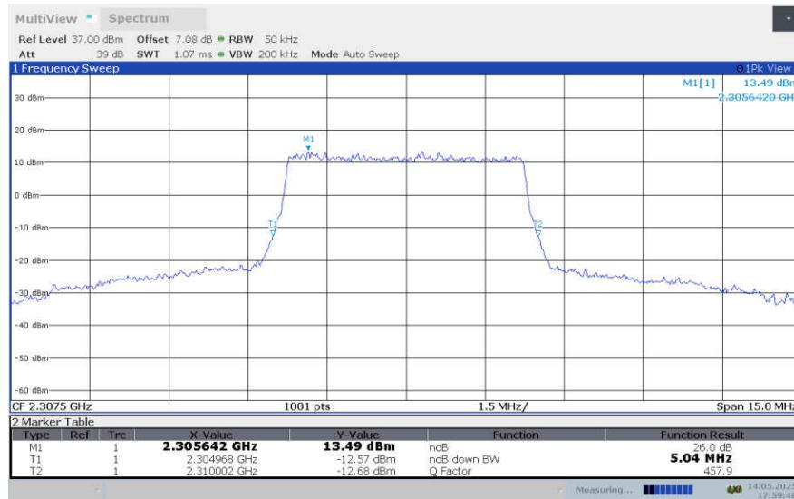
**LTE band 30 , 5MHz Bandwidth,LOW,64QAM (-26dBc BW)**
