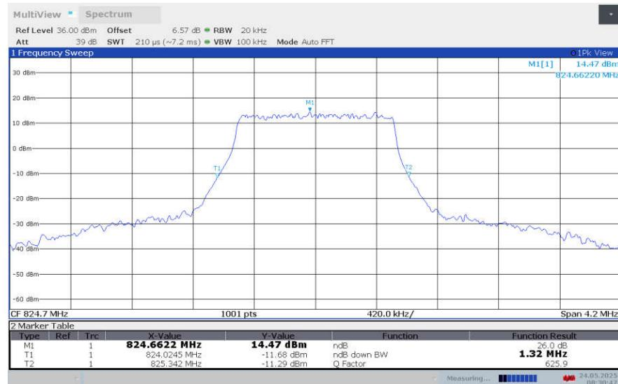
**LTE band 26 , 1.4MHz Bandwidth,LOW,64QAM (-26dBc BW)**
