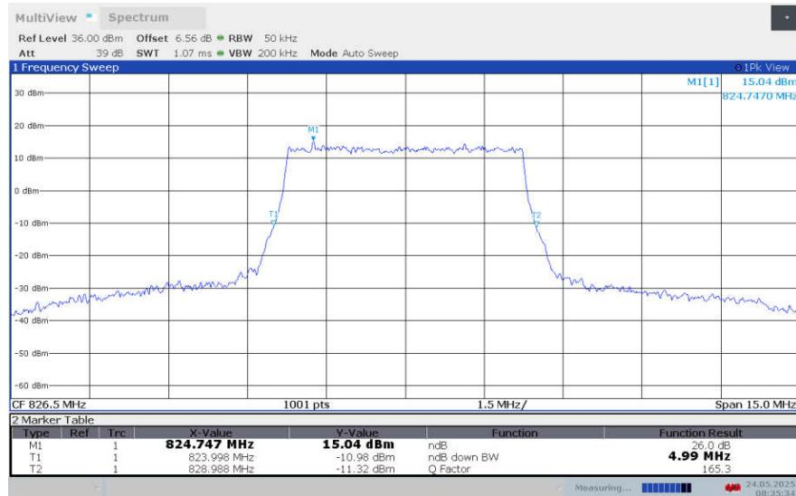
**LTE band 26 , 5MHz Bandwidth,LOW,16QAM (-26dBc BW)**
