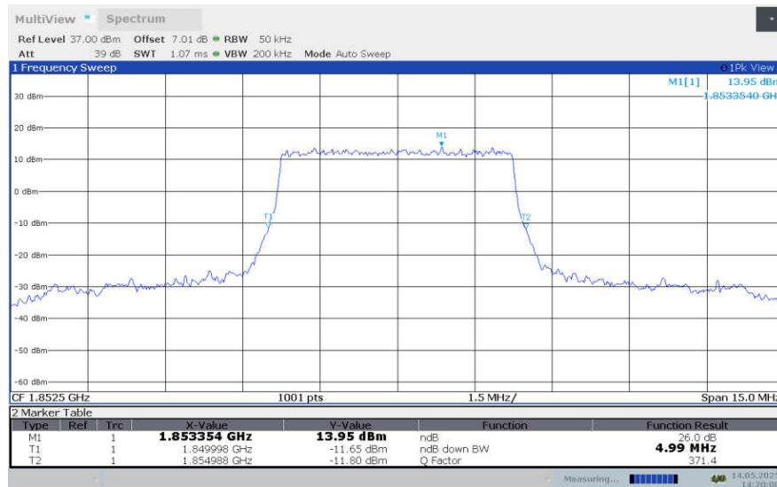
**LTE band 25, 5MHz Bandwidth,LOW,16QAM (-26dBc BW)**
