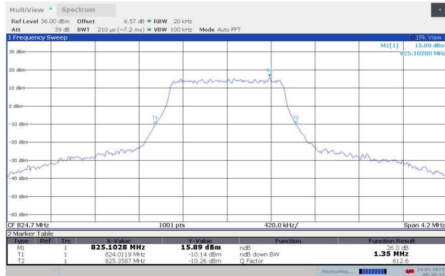
**LTE band 26 , 1.4MHz Bandwidth,LOW,16QAM (-26dBc BW)**
