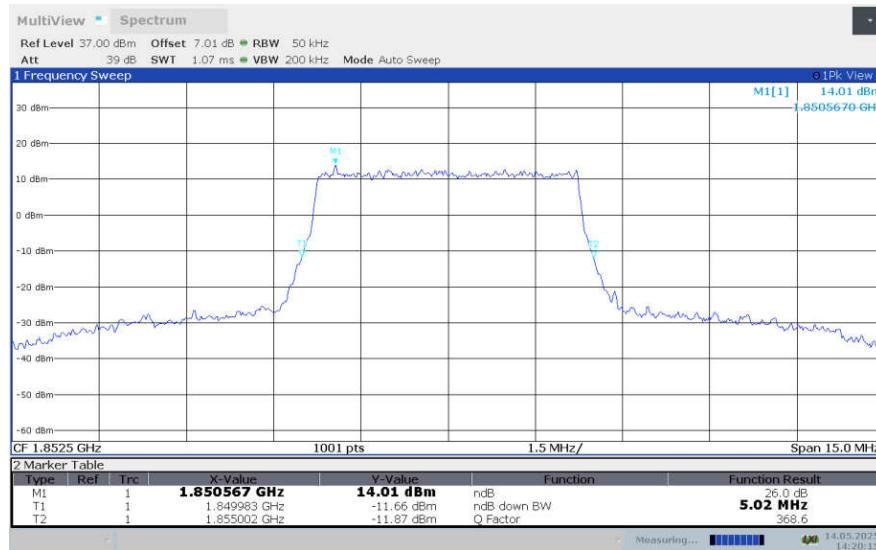
**LTE band 25, 5MHz Bandwidth,LOW,64QAM (-26dBc BW)**
