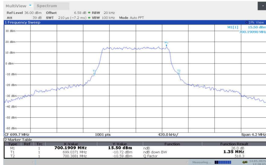
**LTE band 12 , 1.4MHz Bandwidth,LOW,16QAM (-26dBc BW)**
