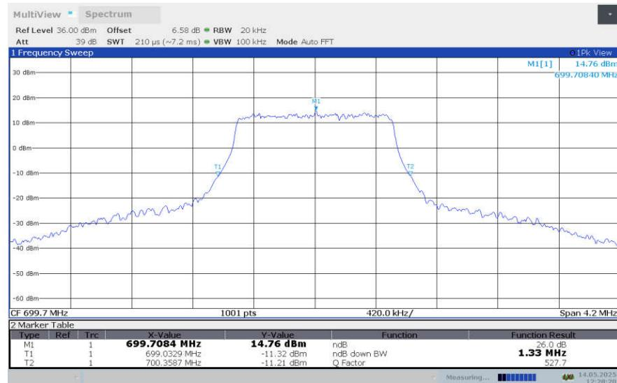
**LTE band 12 , 1.4MHz Bandwidth,LOW,64QAM (-26dBc BW)**
