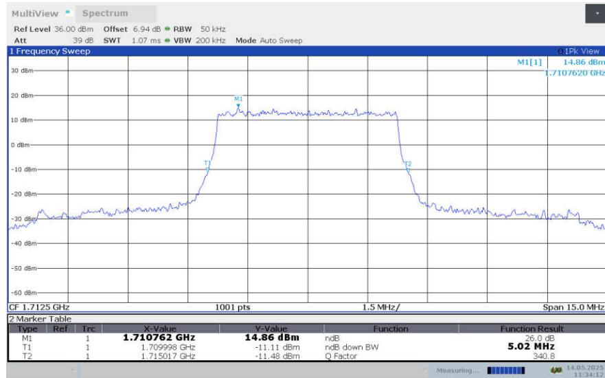
**LTE band 4, 5MHz Bandwidth,LOW,16QAM (-26dBc BW)**
