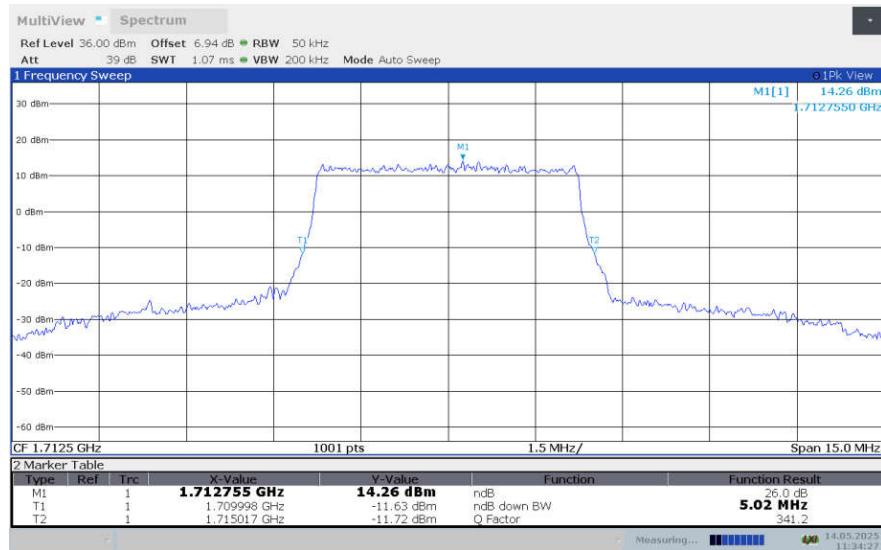
**LTE band 4, 5MHz Bandwidth,LOW,64QAM (-26dBc BW)**
