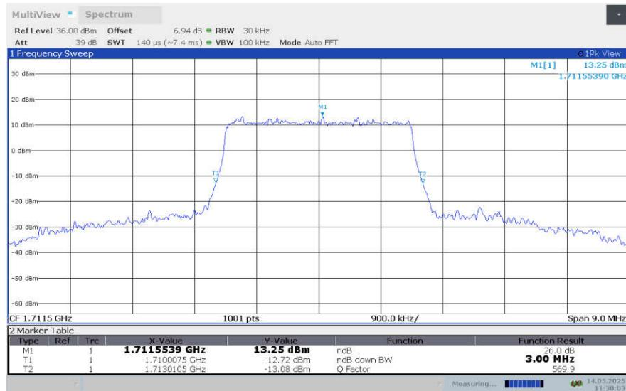
**LTE band 4, 3MHz Bandwidth,LOW,64QAM (-26dBc BW)**
