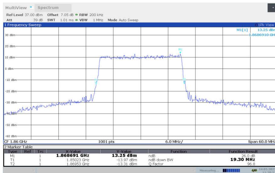
**LTE band 2 , 20MHz Bandwidth,LOW,64QAM (-26dBc BW)**
