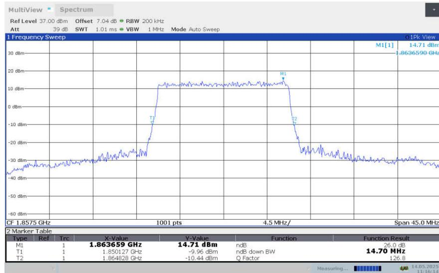
**LTE band 2 , 15MHz Bandwidth,LOW,16QAM (-26dBc BW)**
