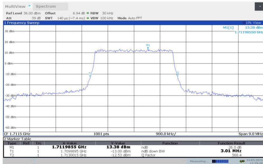
**LTE band 4, 3MHz Bandwidth,LOW,16QAM (-26dBc BW)**
