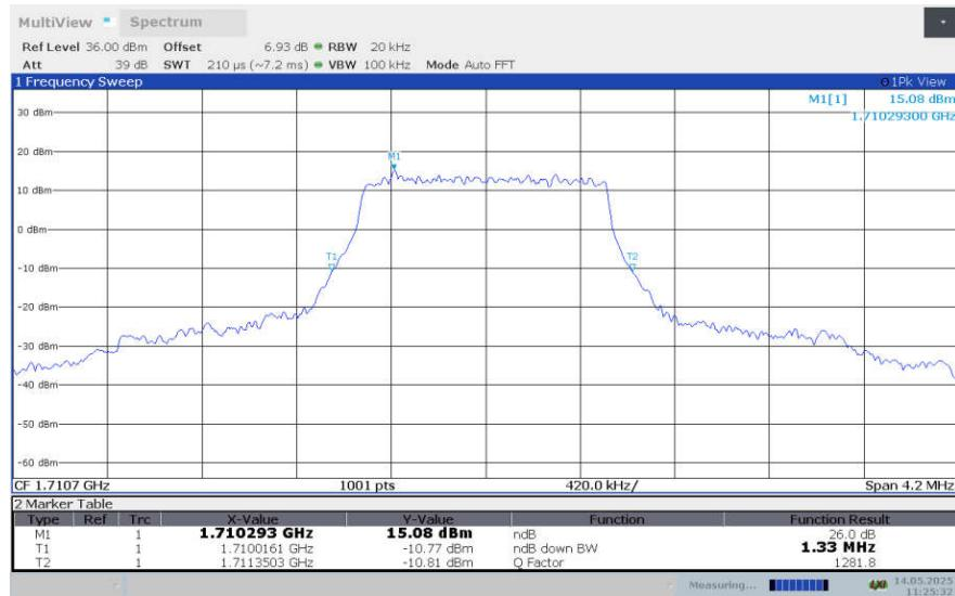
**LTE band 4 , 1.4MHz Bandwidth,LOW,64QAM (-26dBc BW)**
