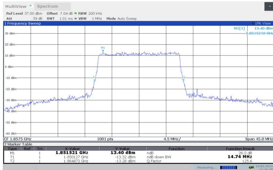
**LTE band 2 , 15MHz Bandwidth,LOW,64QAM (-26dBc BW)**
