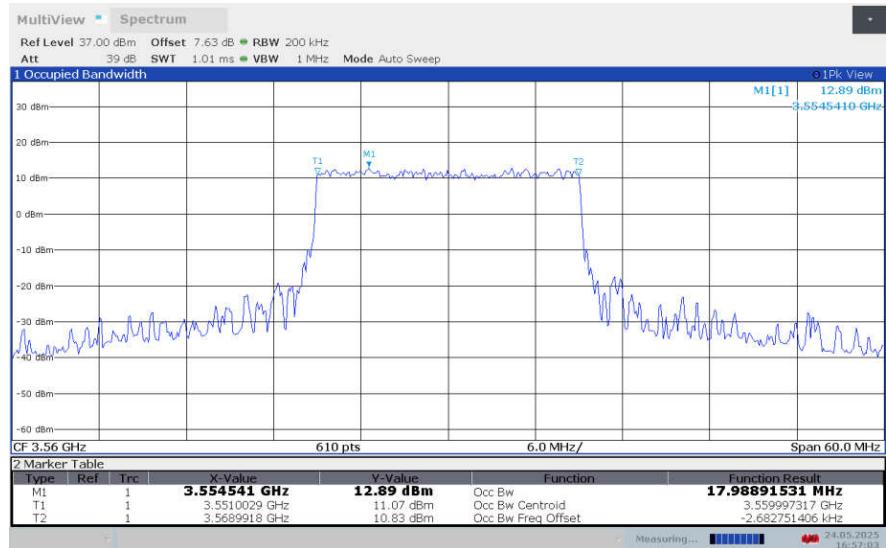
**LTE band 48 , 20MHz Bandwidth,LOW,16QAM (99% BW)**
