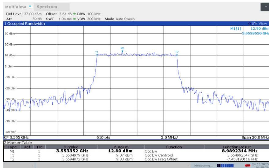
**LTE band 48 , 10MHz Bandwidth,LOW,64QAM (99% BW)**
