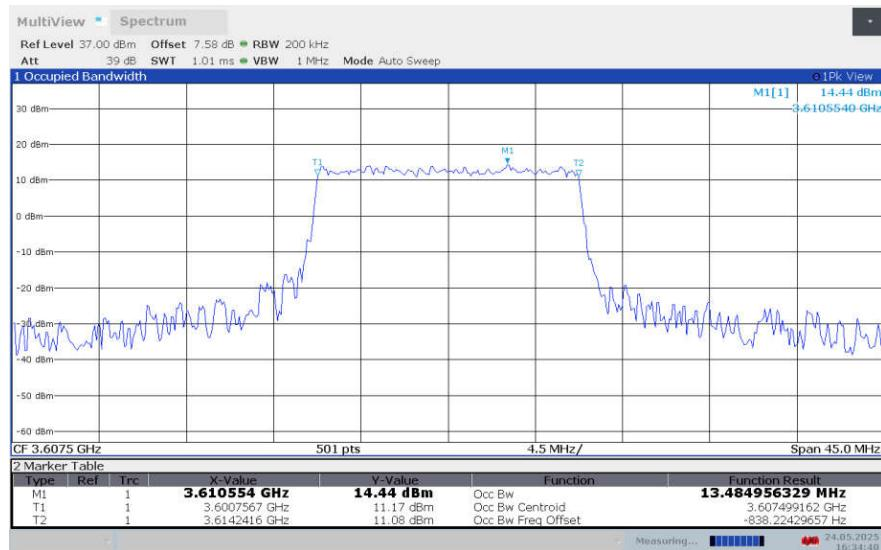
**LTE band 43 , 15MHz Bandwidth,LOW,16QAM (99% BW)**
