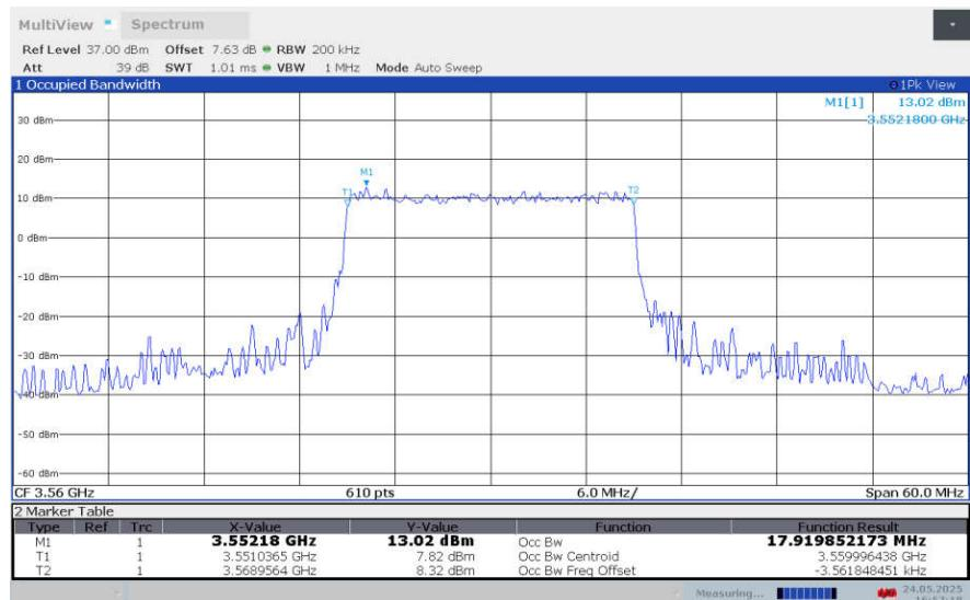
**LTE band 48 , 20MHz Bandwidth,LOW,64QAM (99% BW)**
