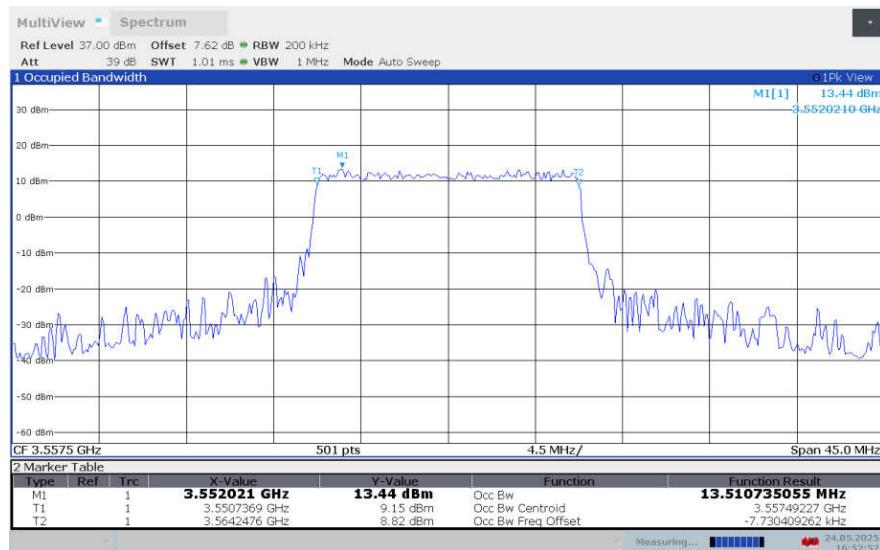
**LTE band 48 , 15MHz Bandwidth,LOW,64QAM (99% BW)**
