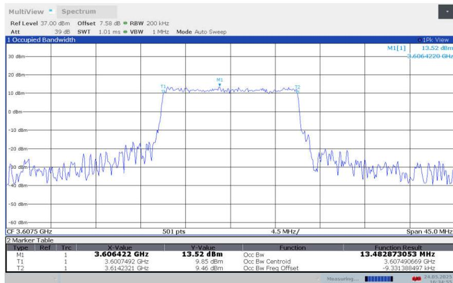
**LTE band 43 , 15MHz Bandwidth,LOW,64QAM (99% BW)**
