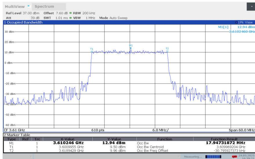
**LTE band 43 , 20MHz Bandwidth,LOW,64QAM (99% BW)**
