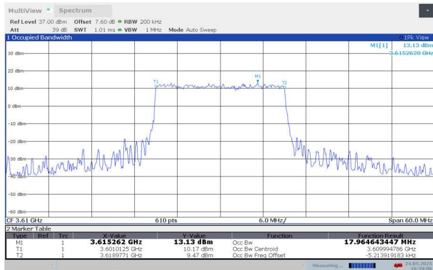
**LTE band 43 , 20MHz Bandwidth,LOW,16QAM (99% BW)**
