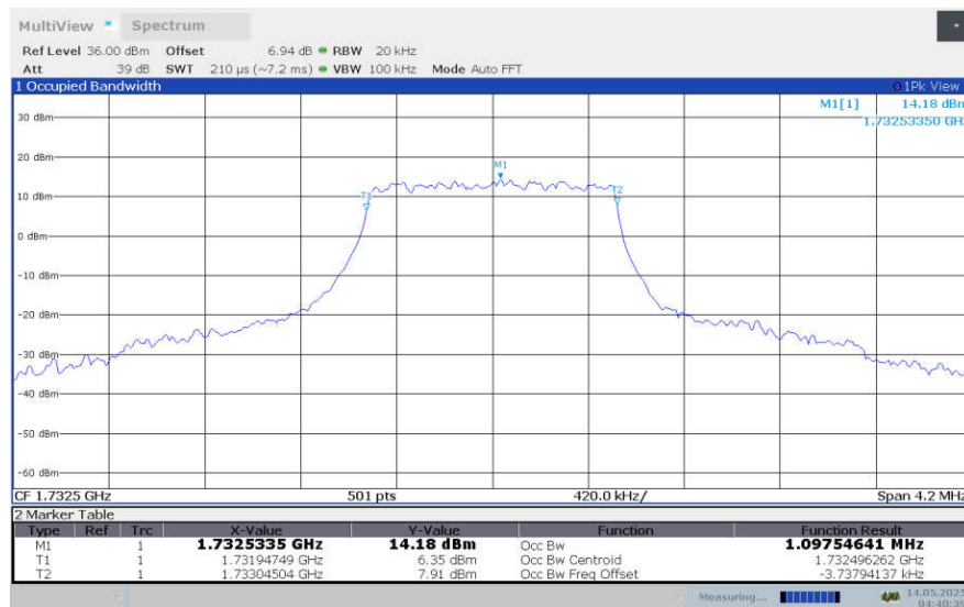
LTE band 4 , 1.4MHz Bandwidth,MID,64QAM (99% BW)
