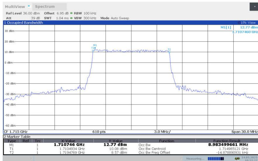
**LTE band 66 , 10MHz Bandwidth,LOW,64QAM (99% BW)**
