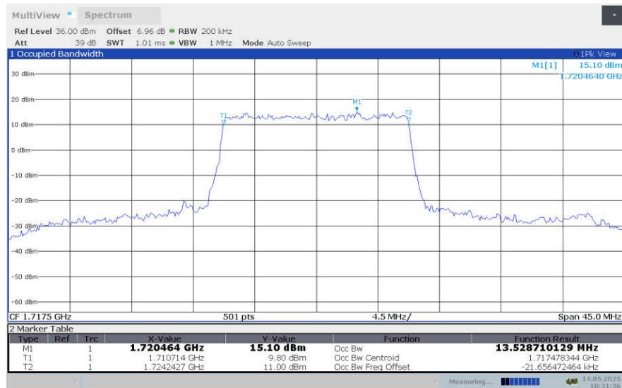
**LTE band 66 , 15MHz Bandwidth,LOW,16QAM (99% BW)**
