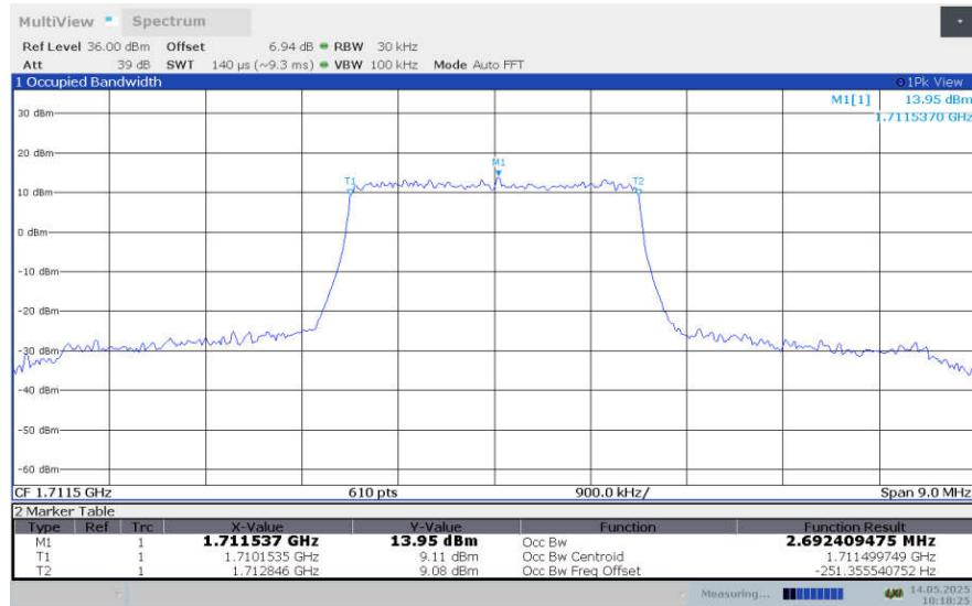
**LTE band 66 , 3MHz Bandwidth,LOW,16QAM (99% BW)**
