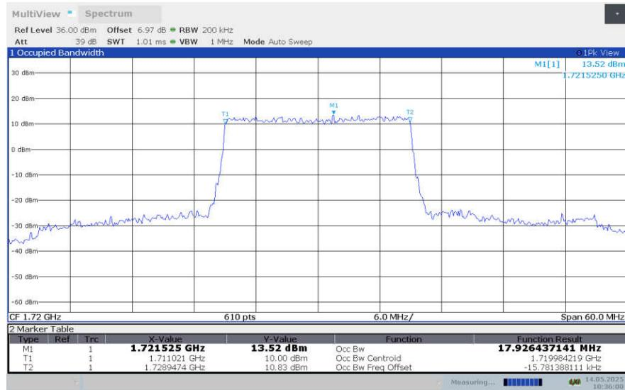
**LTE band 66 , 20MHz Bandwidth,LOW,16QAM (99% BW)**
