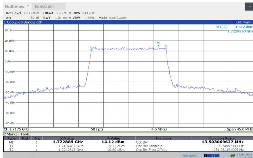
**LTE band 66 , 15MHz Bandwidth,LOW,64QAM (99% BW)**
