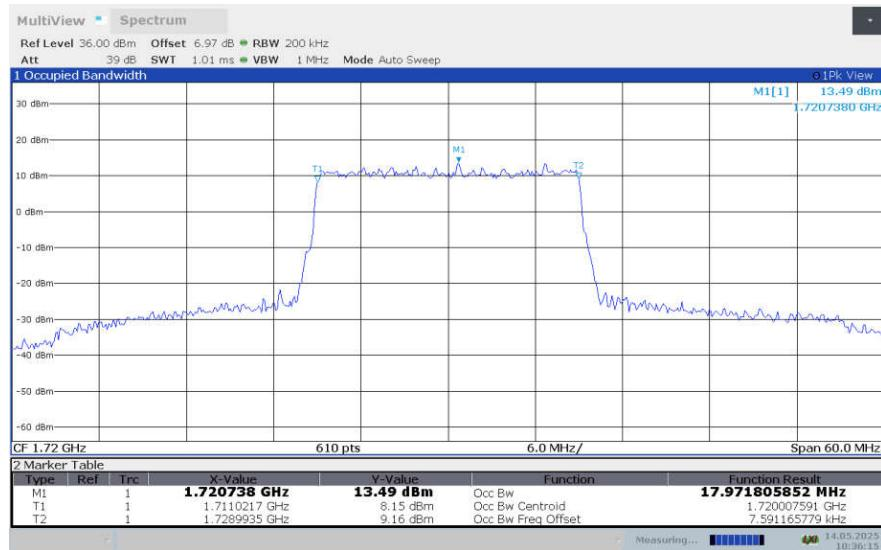
**LTE band 66 , 20MHz Bandwidth,LOW,64QAM (99% BW)**
