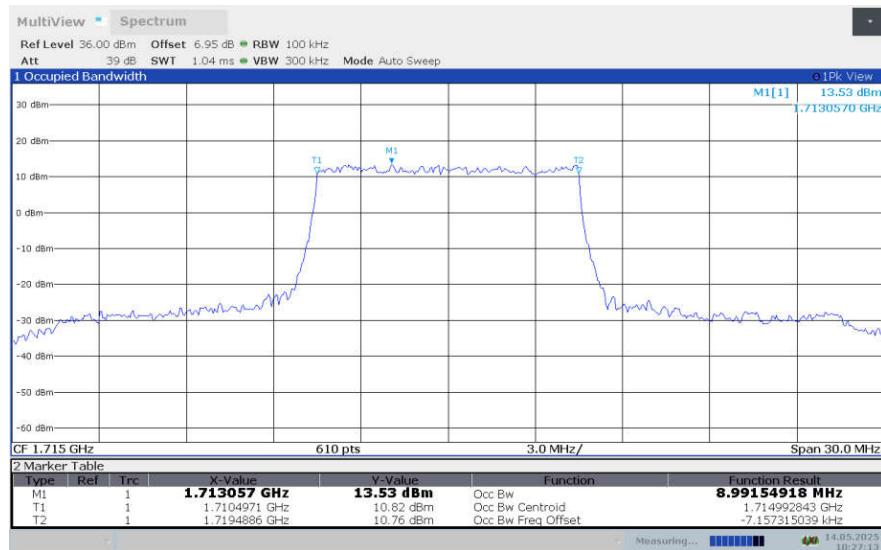
**LTE band 66 , 10MHz Bandwidth,LOW,16QAM (99% BW)**
