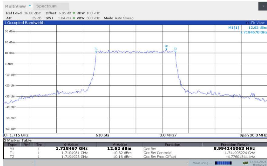
**LTE band 4 , 10MHz Bandwidth,LOW,64QAM (99% BW)**
