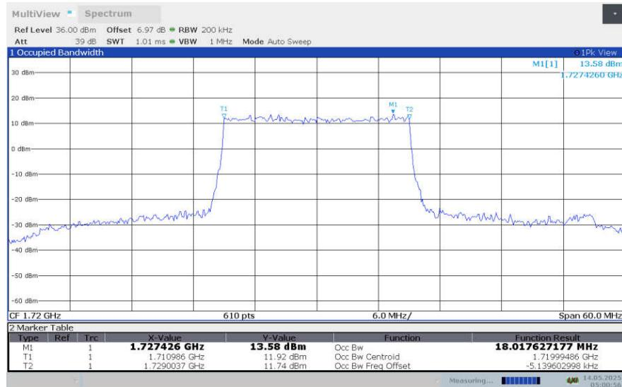
**LTE band 4, 20MHz Bandwidth,LOW,16QAM (99% BW)**
