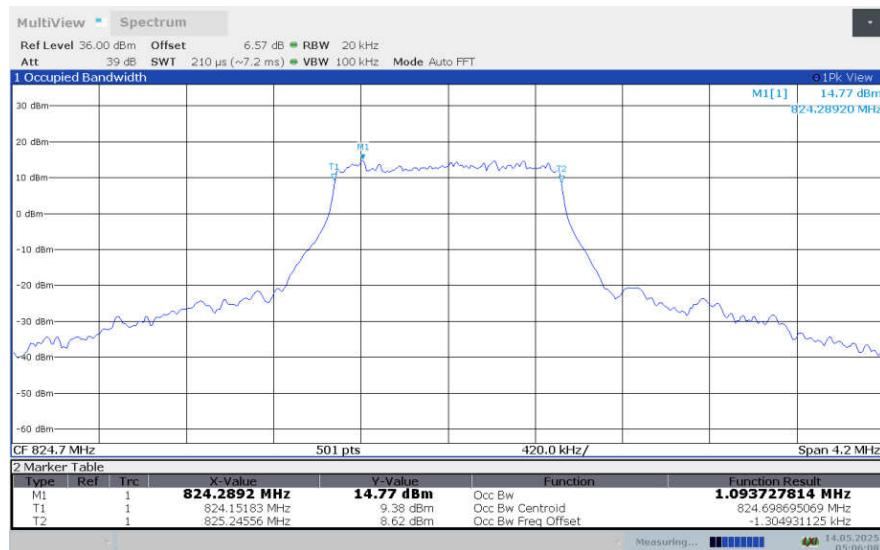
**LTE band 5 , 1.4MHz Bandwidth,LOW,64QAM (99% BW)**
