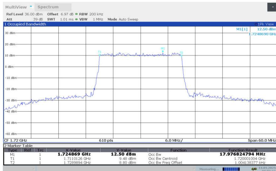
**LTE band 4, 20MHz Bandwidth,LOW,64QAM (99% BW)**
