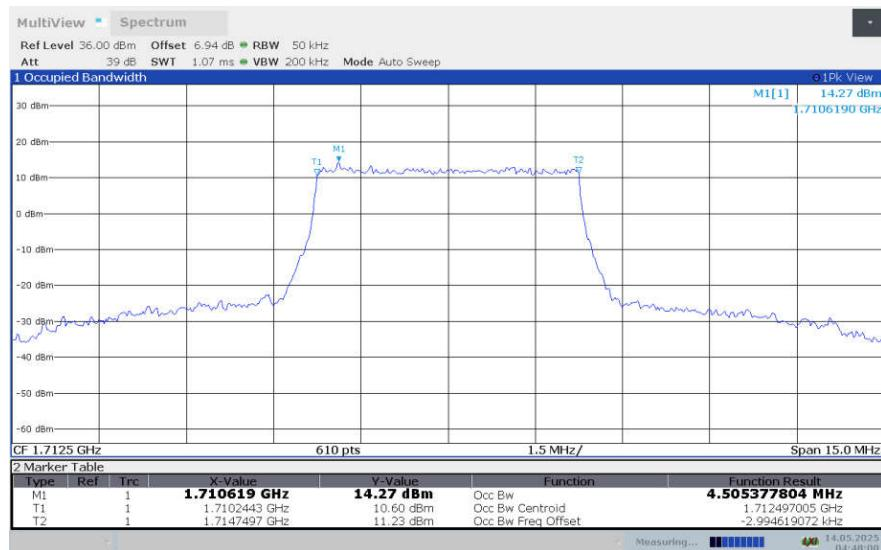
**LTE band 4, 5MHz Bandwidth,LOW,64QAM (99% BW)**
