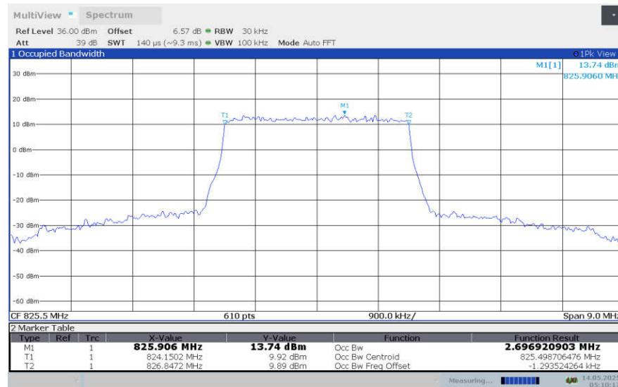
**LTE band 5 , 3MHz Bandwidth,LOW,16QAM (99% BW)**
