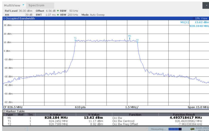
**LTE band 5 , 5MHz Bandwidth,LOW,64QAM (99% BW)**
