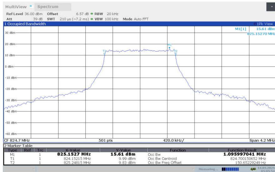
**LTE band 5 , 1.4MHz Bandwidth,LOW,16QAM (99% BW)**
