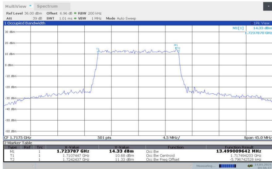
**LTE band 4 , 15MHz Bandwidth,LOW,64QAM (99% BW)**
