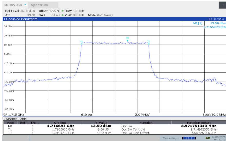
**LTE band 4 , 10MHz Bandwidth,LOW,16QAM (99% BW)**
