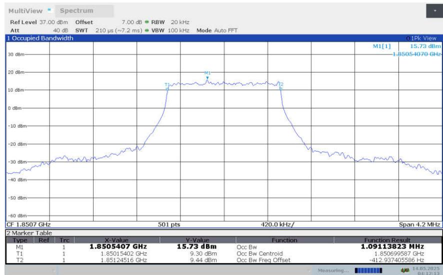
**LTE band 2 , 1.4MHz Bandwidth,LOW,16QAM (99% BW)**
