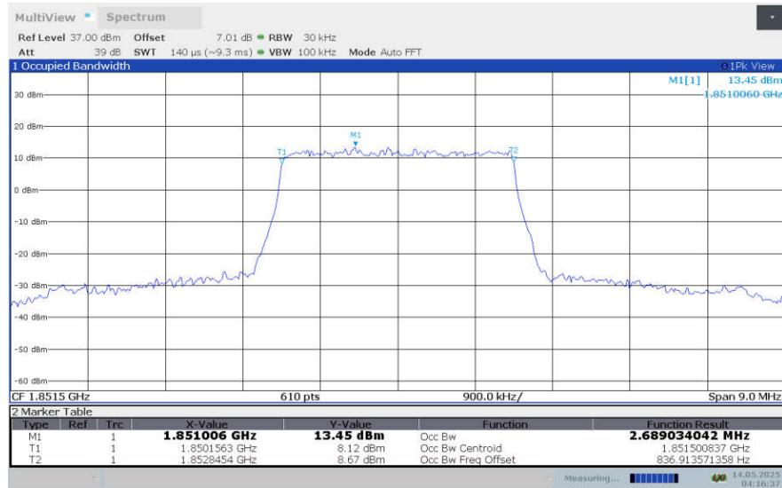
**LTE band 2 , 3MHz Bandwidth,LOW,16QAM (99% BW)**
