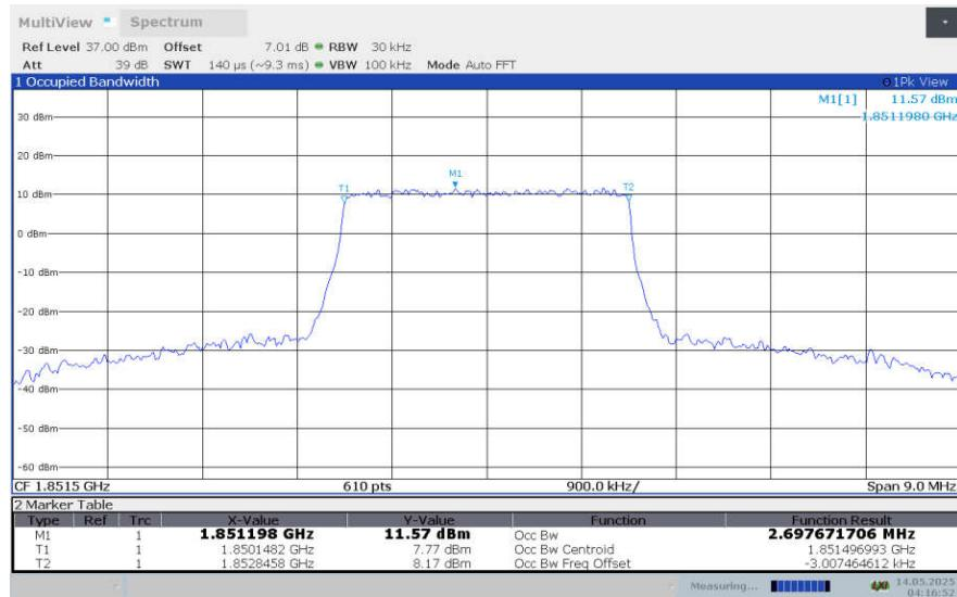
**LTE band 2 , 3MHz Bandwidth,LOW,64QAM (99% BW)**
