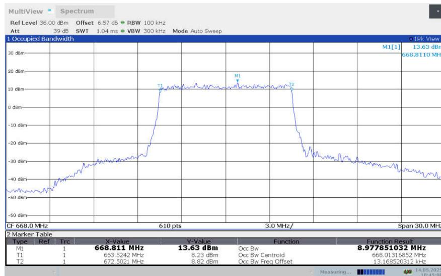
**LTE band 71 , 10MHz Bandwidth,LOW,64QAM (99% BW)**
