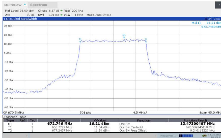
**LTE band 71 , 15MHz Bandwidth,LOW,16QAM (99% BW)**
