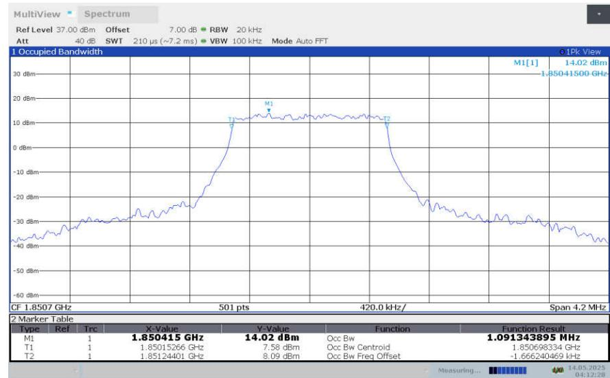
**LTE band 2 , 1.4MHz Bandwidth,LOW,64QAM (99% BW)**
