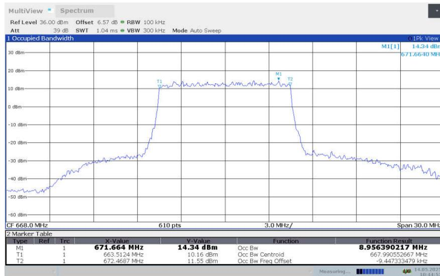
**LTE band 71 , 10MHz Bandwidth,LOW,16QAM (99% BW)**
