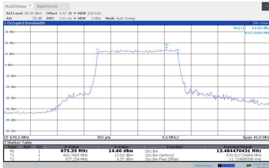
**LTE band 71 , 15MHz Bandwidth,LOW,64QAM (99% BW)**
