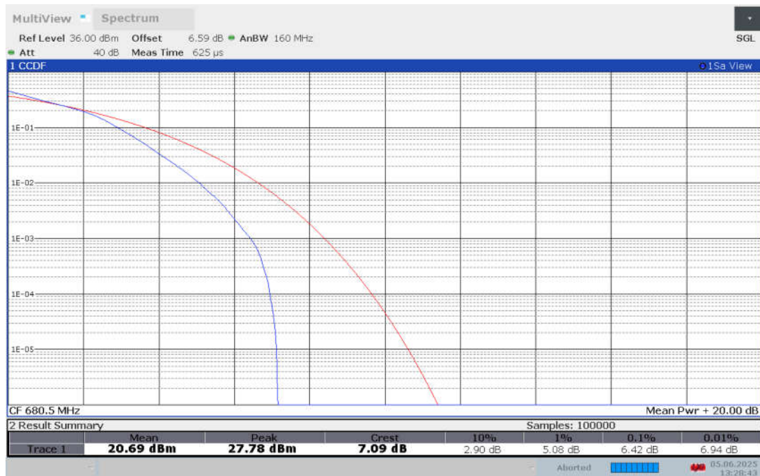
Band n71 , 20MHz Bandwidth,DFT-s-64QAM
