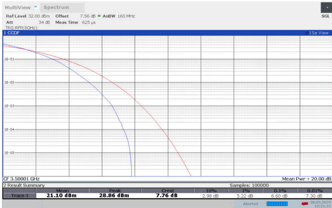
Band n77L , 40MHz Bandwidth,CP-QPSK
