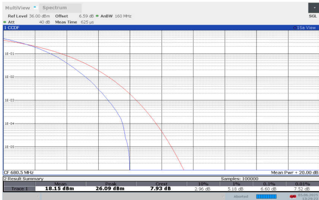
Band n71 , 20MHz Bandwidth,CP-QPSK
