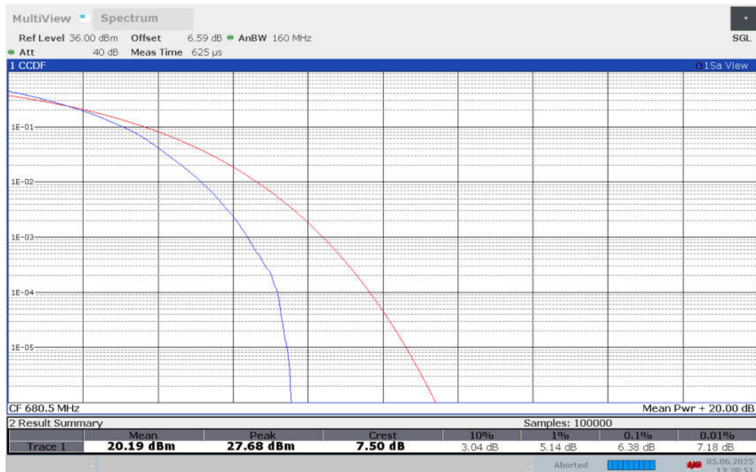
Band n71 , 20MHz Bandwidth,DFT-s-256QAM
