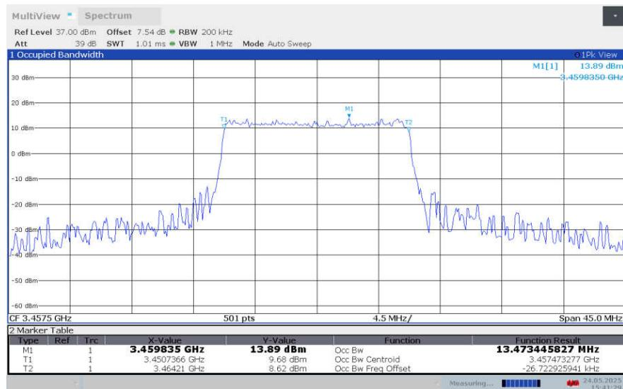
**LTE band 42 , 15MHz Bandwidth,LOW,64QAM (99% BW)**
