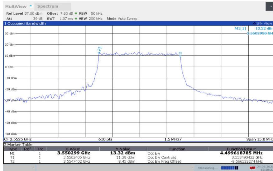
**LTE band 42 , 5MHz Bandwidth,LOW,64QAM (99% BW)**
