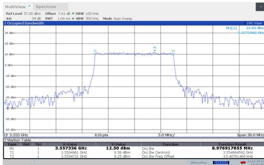
**LTE band 42 , 10MHz Bandwidth,LOW,64QAM (99% BW)**
