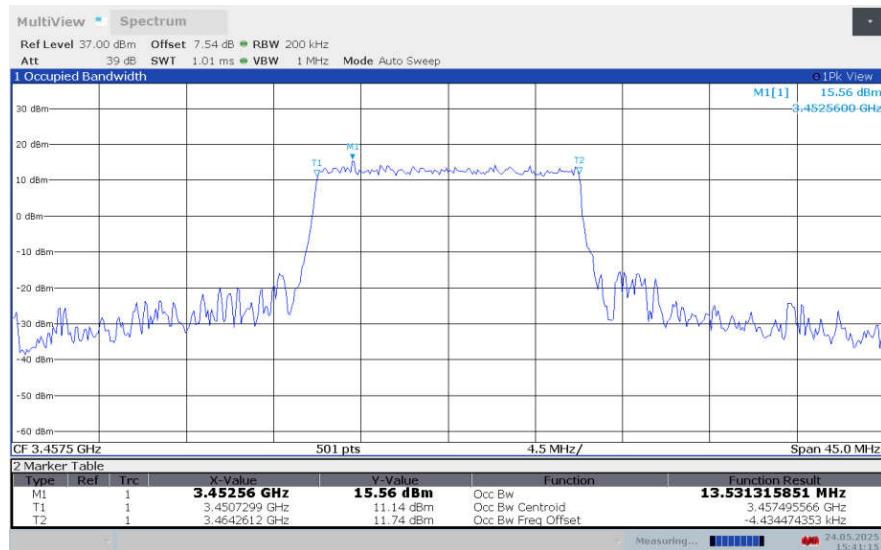
**LTE band 42 , 15MHz Bandwidth,LOW,16QAM (99% BW)**
