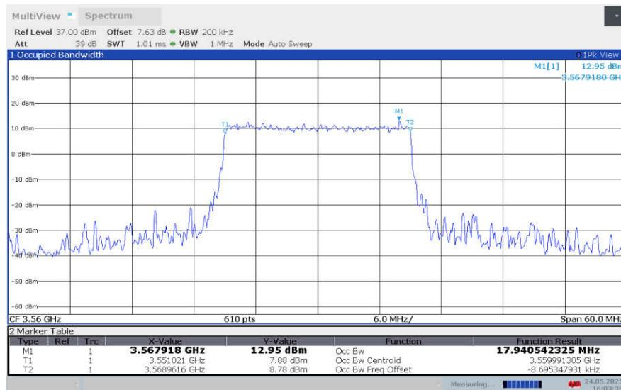
**LTE band 42 , 20MHz Bandwidth,LOW,64QAM (99% BW)**
