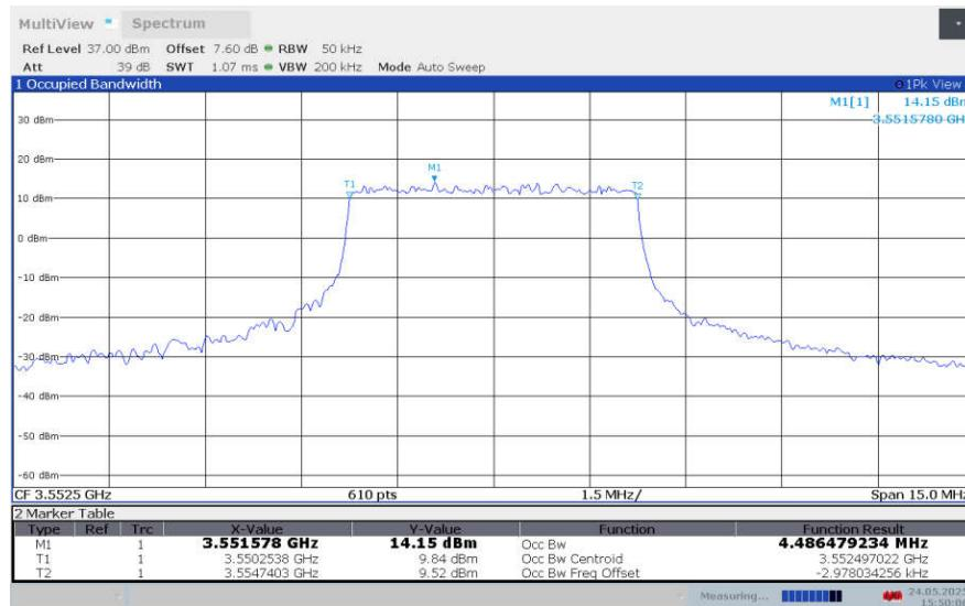
**LTE band 42 , 5MHz Bandwidth,LOW,16QAM (99% BW)**
