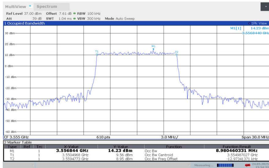
**LTE band 42 , 10MHz Bandwidth,LOW,16QAM (99% BW)**
