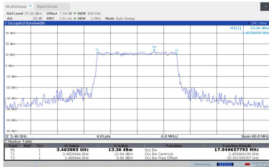
**LTE band 42 , 20MHz Bandwidth,LOW,16QAM (99% BW)**
