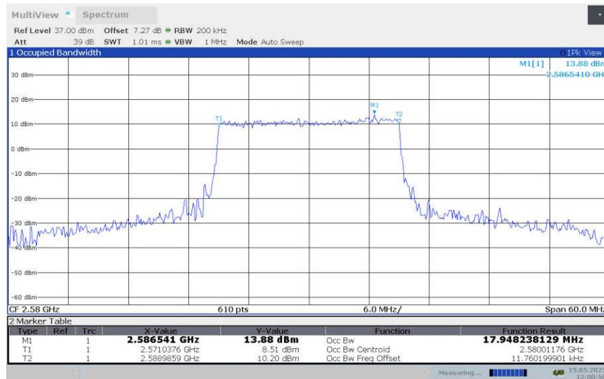
**LTE band 38 , 20MHz Bandwidth,LOW,16QAM (99% BW)**
