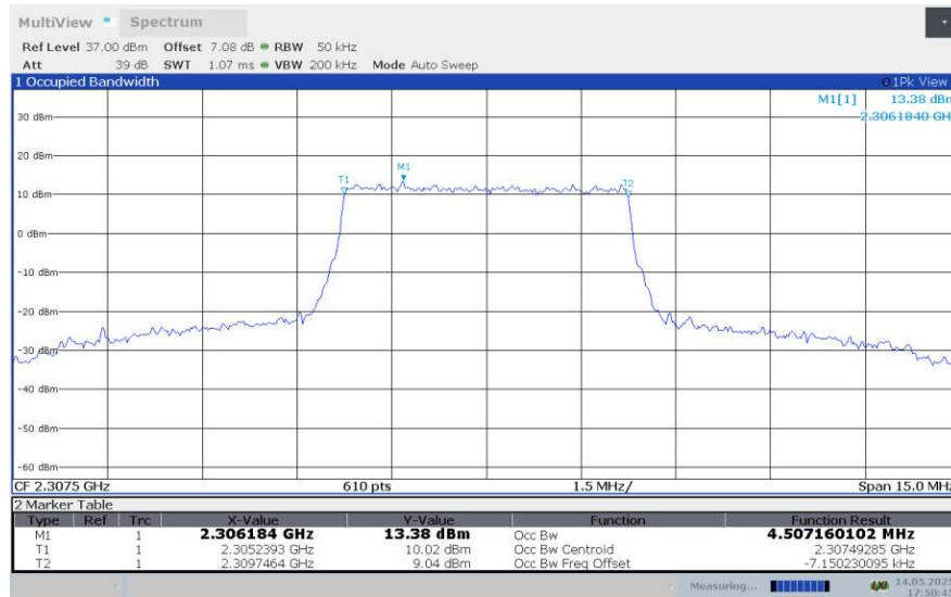
**LTE band 30 , 5MHz Bandwidth,LOW,64QAM (99% BW)**
