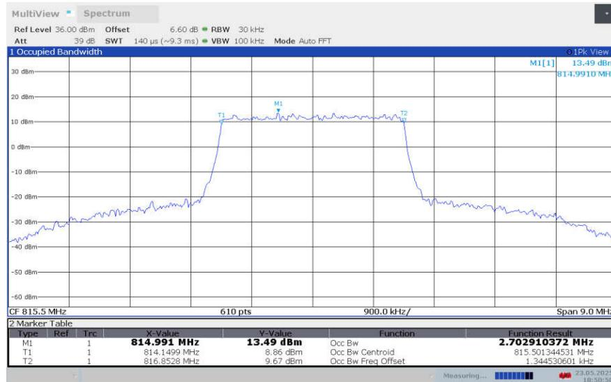
**LTE band 26 , 3MHz Bandwidth,LOW,16QAM (99% BW)**
