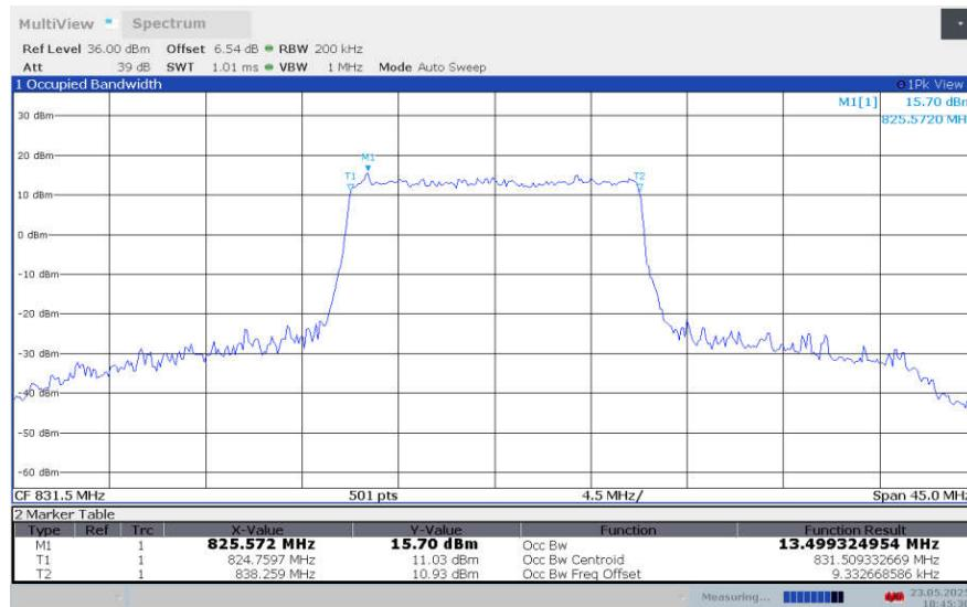
**LTE band 26 , 15MHz Bandwidth,LOW,16QAM (99% BW)**
