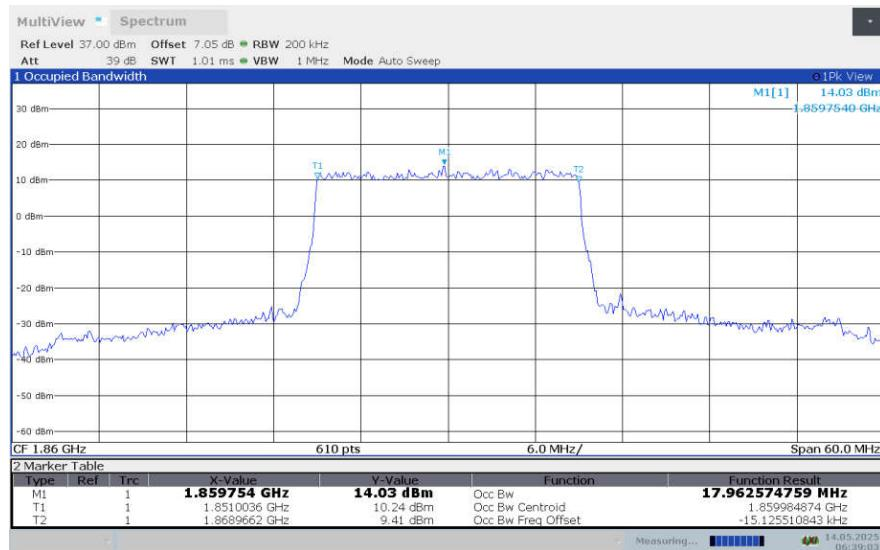
**LTE band 25 , 20MHz Bandwidth,LOW,16QAM (99% BW)**
