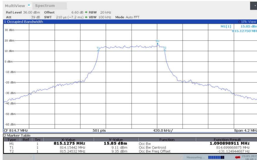
**LTE band 26 , 1.4MHz Bandwidth,LOW,16QAM (99% BW)**
