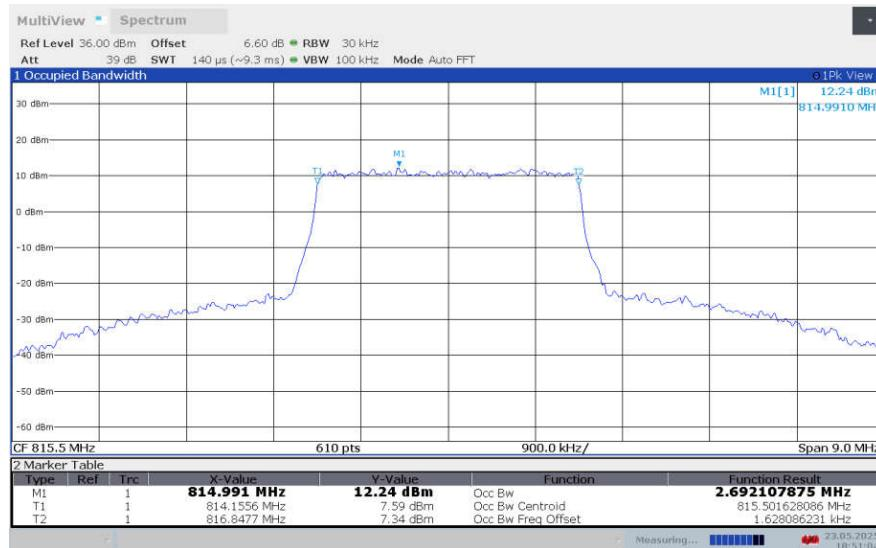
**LTE band 26 , 3MHz Bandwidth,LOW,64QAM (99% BW)**
