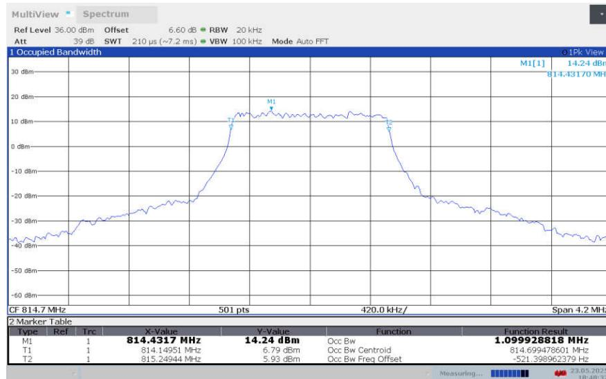
**LTE band 26 , 1.4MHz Bandwidth,LOW,64QAM (99% BW)**
