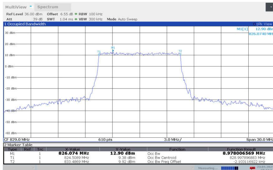
**LTE band 26 , 10MHz Bandwidth,LOW,64QAM (99% BW)**
