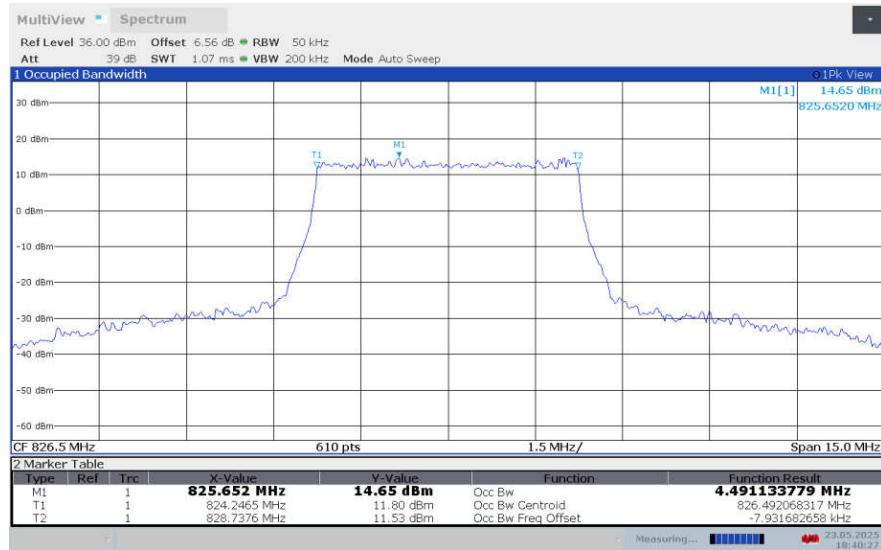
**LTE band 26 , 5MHz Bandwidth,LOW,16QAM (99% BW)**
