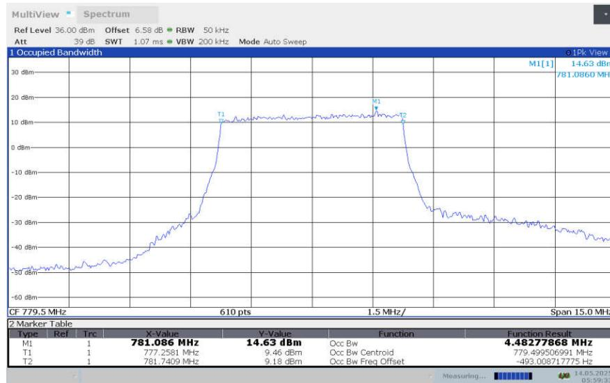
**LTE band 13, 5MHz Bandwidth,LOW,64QAM (99% BW)**
