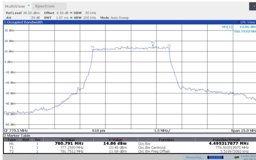
**LTE band 13, 5MHz Bandwidth,LOW,16QAM (99% BW)**
