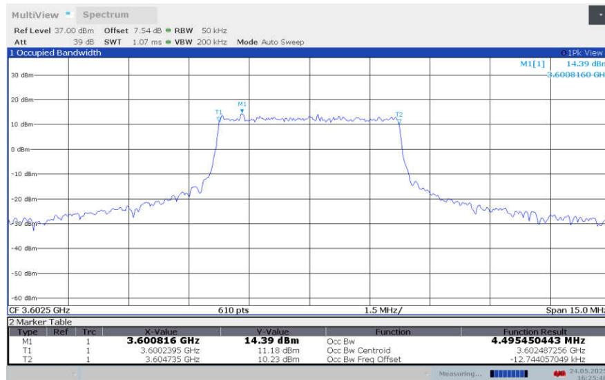
**LTE band 43 , 5MHz Bandwidth,LOW,16QAM (99% BW)**
