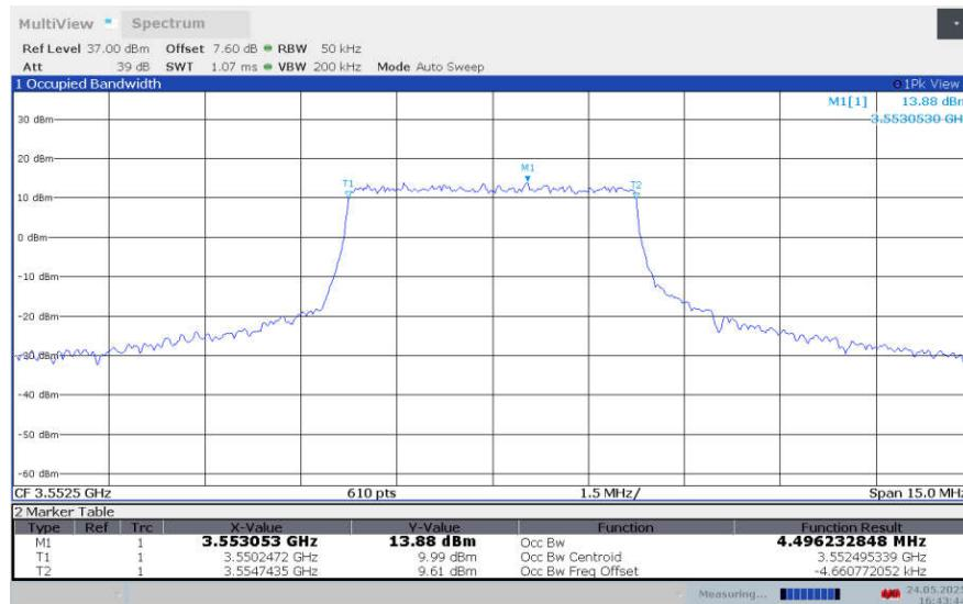
**LTE band 48 , 5MHz Bandwidth,LOW,16QAM (99% BW)**
