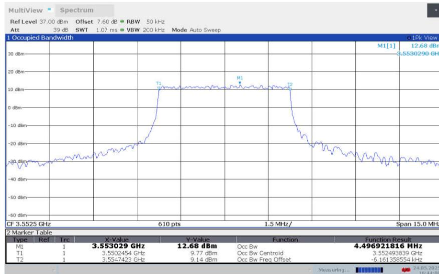
**LTE band 48 , 5MHz Bandwidth,LOW,64QAM (99% BW)**
