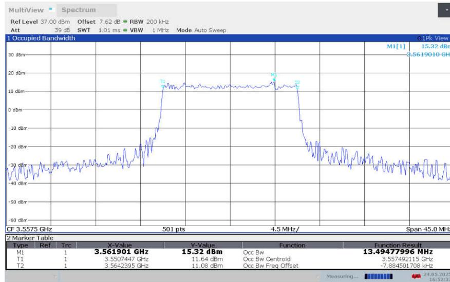
**LTE band 48 , 15MHz Bandwidth,LOW,16QAM (99% BW)**
