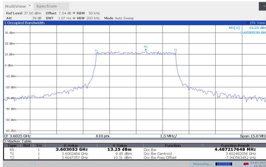
**LTE band 43 , 5MHz Bandwidth,LOW,64QAM (99% BW)**
