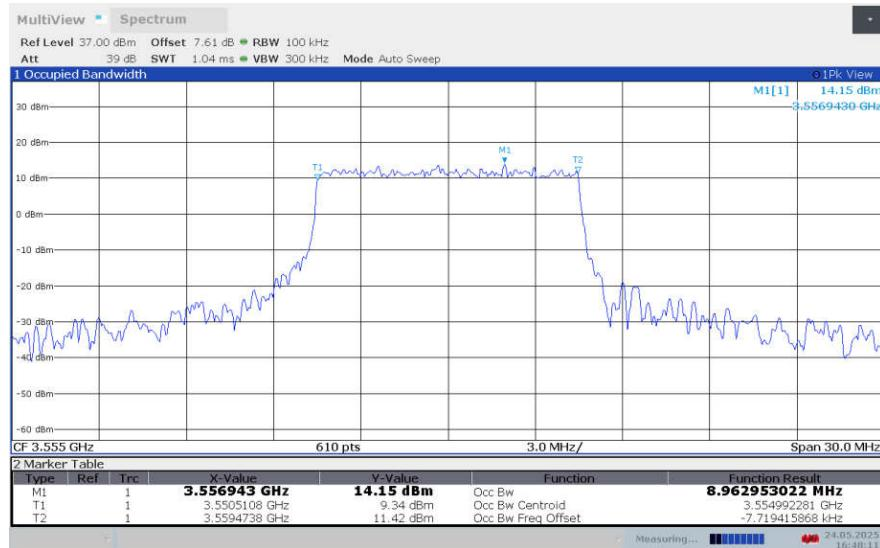
**LTE band 48 , 10MHz Bandwidth,LOW,16QAM (99% BW)**
