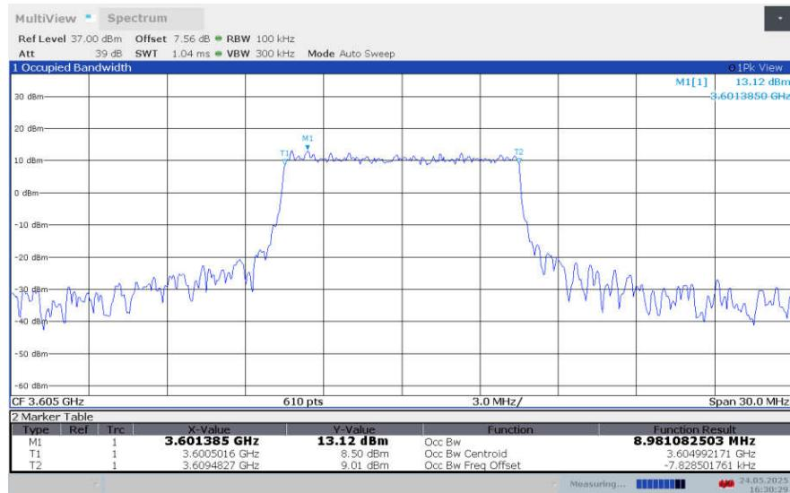
**LTE band 43 , 10MHz Bandwidth,LOW,64QAM (99% BW)**
