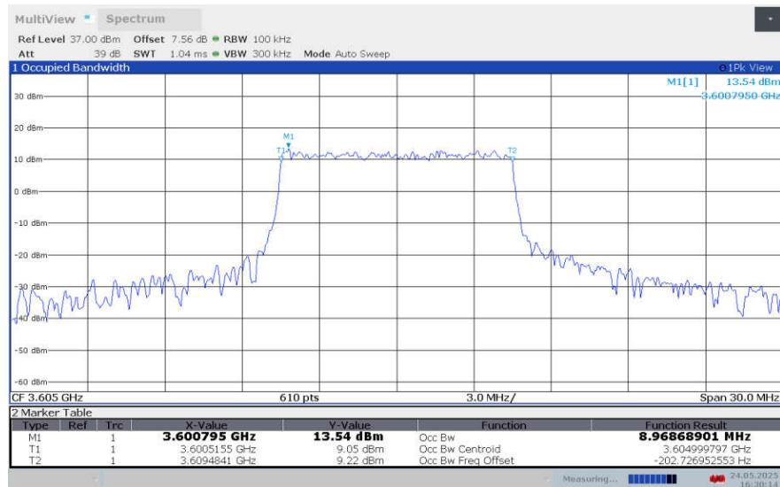
**LTE band 43 , 10MHz Bandwidth,LOW,16QAM (99% BW)**
