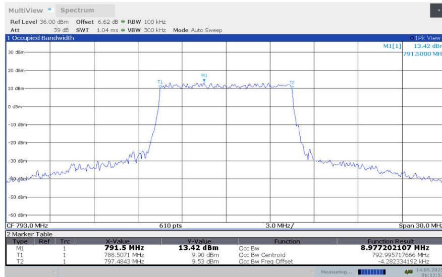
**LTE band 14 , 10MHz Bandwidth,LOW,64QAM (99% BW)**
