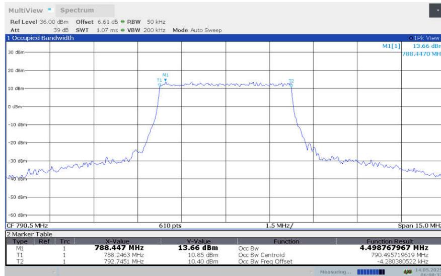
**LTE band 14, 5MHz Bandwidth,LOW,64QAM (99% BW)**
