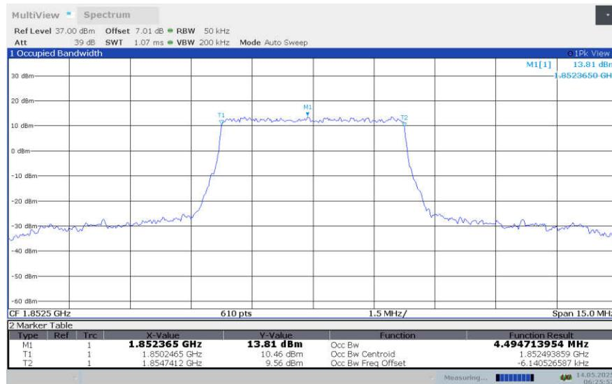
**LTE band 25, 5MHz Bandwidth,LOW,16QAM (99% BW)**
