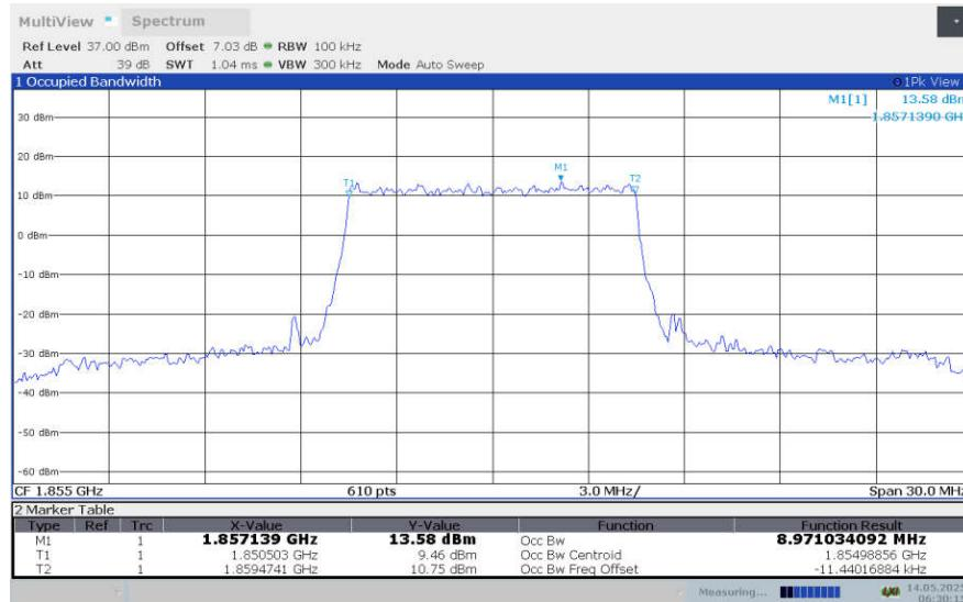
**LTE band 25 , 10MHz Bandwidth,LOW,16QAM (99% BW)**
