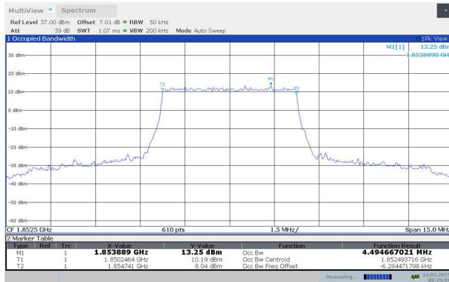
**LTE band 25, 5MHz Bandwidth,LOW,64QAM (99% BW)**
