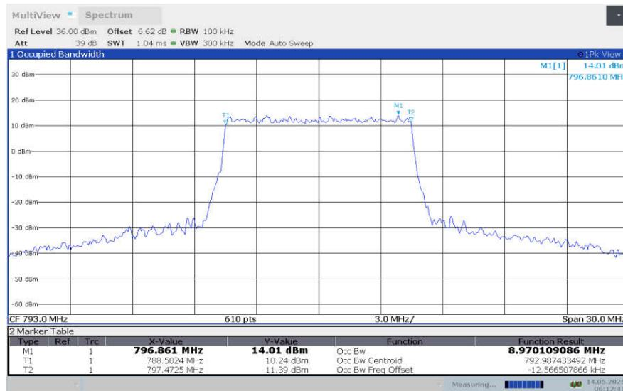
**LTE band 14 , 10MHz Bandwidth,LOW,16QAM (99% BW)**
