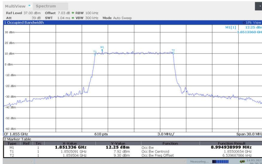
**LTE band 25 , 10MHz Bandwidth,LOW,64QAM (99% BW)**
