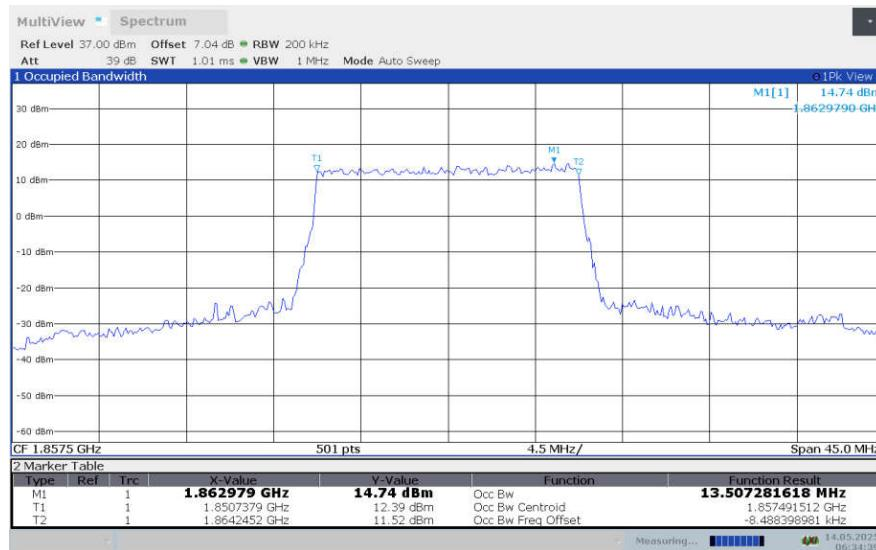
**LTE band 25 , 15MHz Bandwidth,LOW,16QAM (99% BW)**
