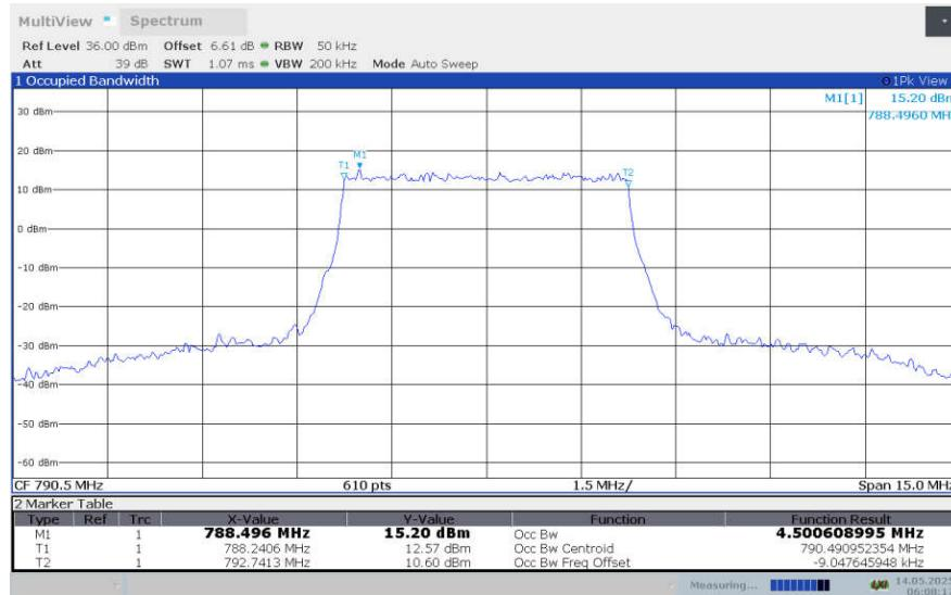
**LTE band 14, 5MHz Bandwidth,LOW,16QAM (99% BW)**
