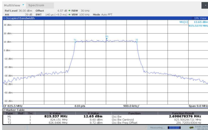
**LTE band 5 , 3MHz Bandwidth,LOW,64QAM (99% BW)**
