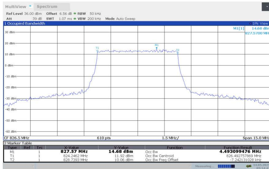
**LTE band 5 , 5MHz Bandwidth,LOW,16QAM (99% BW)**
