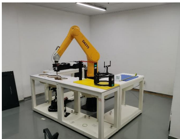
Picture D.6 Specific Absorption Rate Test Layout
