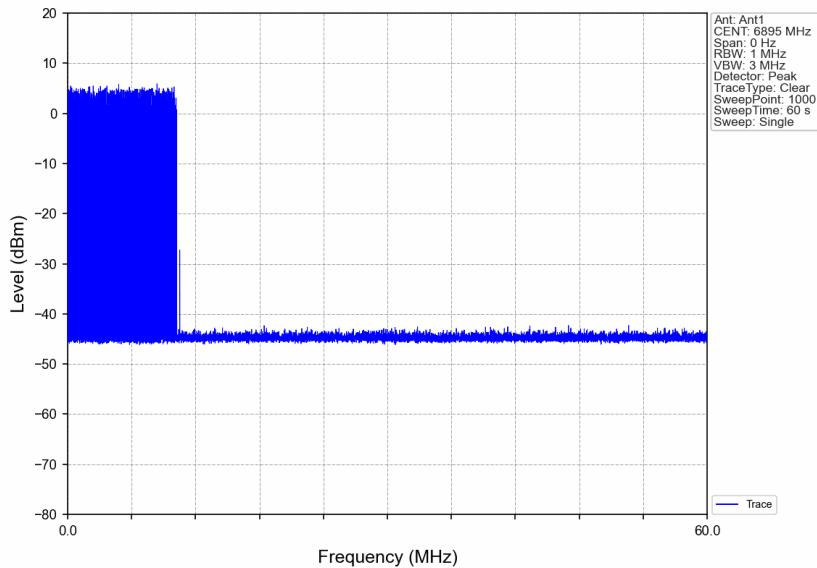
802.11ax(HEW20)\_LCH\_6895MHz\_Ant1\_NTNV\_- Inject Incumbent signal at 10th seconds and remove the signal at 50 seconds
