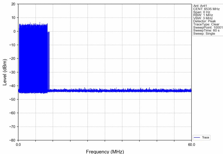
802.11ax(HEW20)\_LCH\_6535MHz\_Ant1\_NTNV\_- Inject Incumbent signal at 10th seconds and remove the signal at 50 seconds
