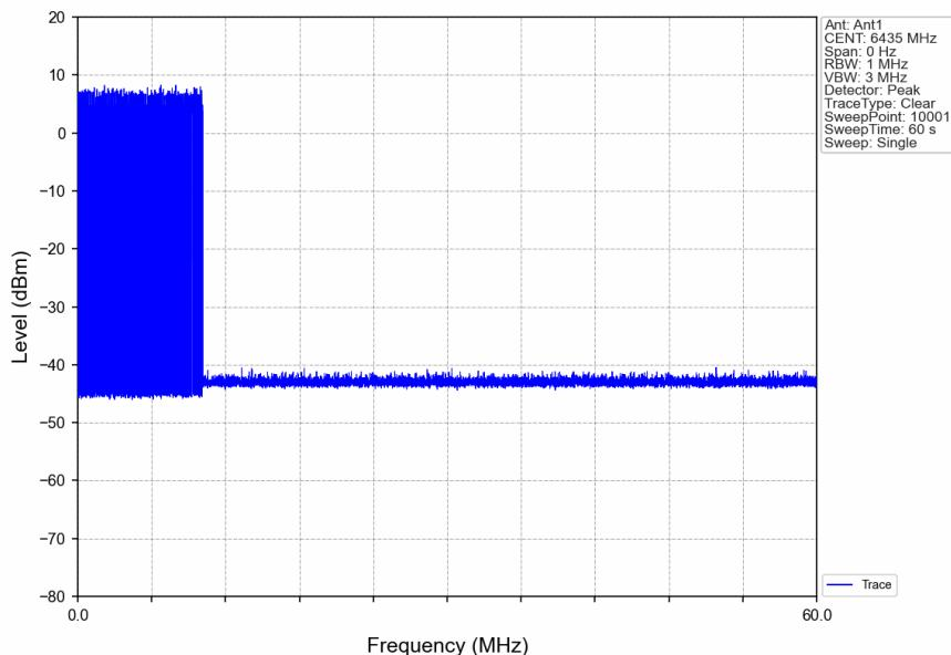
802.11ax(HEW20)\_LCH\_6435MHz\_Ant1\_NTNV\_- Inject Incumbent signal at 10th seconds and remove the signal at 50 seconds
