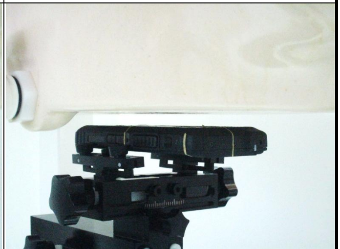
Rear Face of EUT with 1.0 cm Gap
