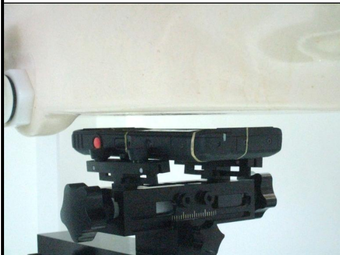
Front Face of EUT with 1.0 cm Gap
