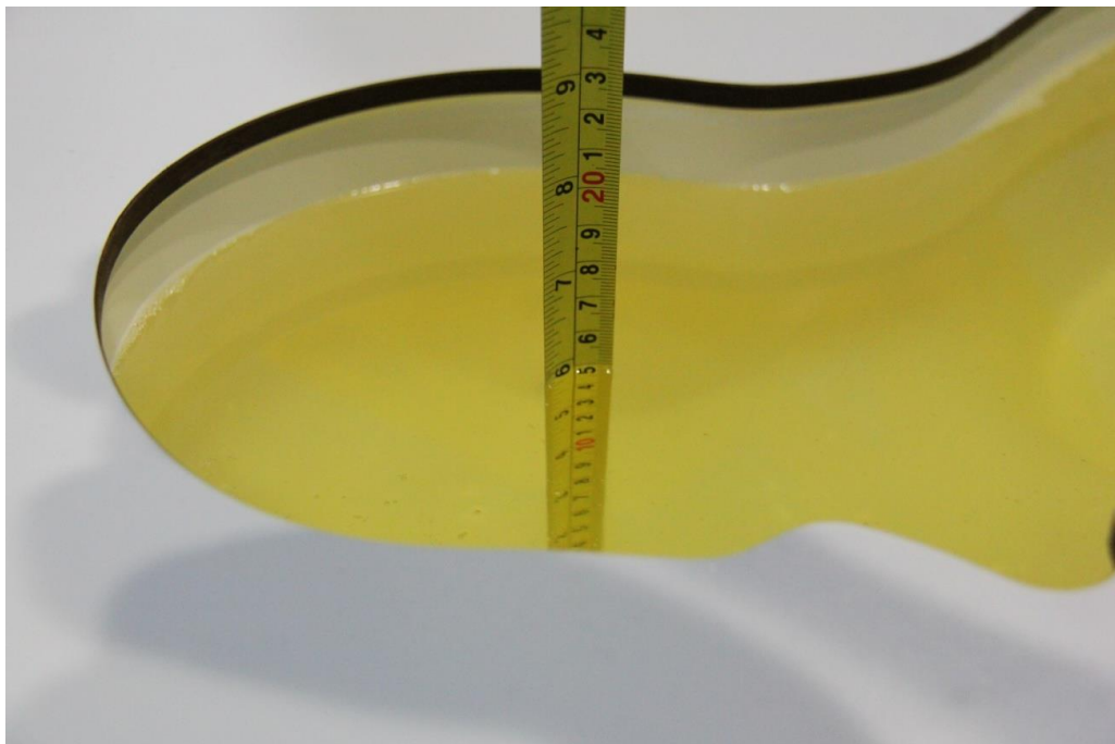
Picture 7-6: Liquid depth in the Head Phantom(2450MHz)
