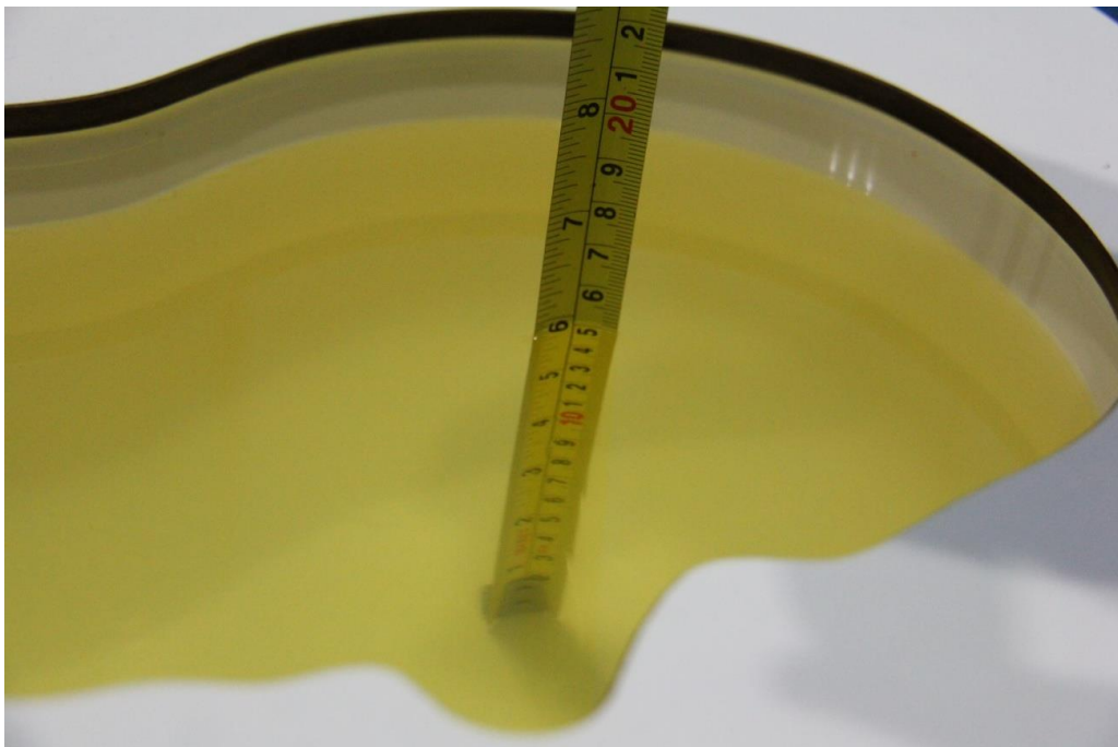
Picture 7-10: Liquid depth in the Head Phantom(3900MHz)
