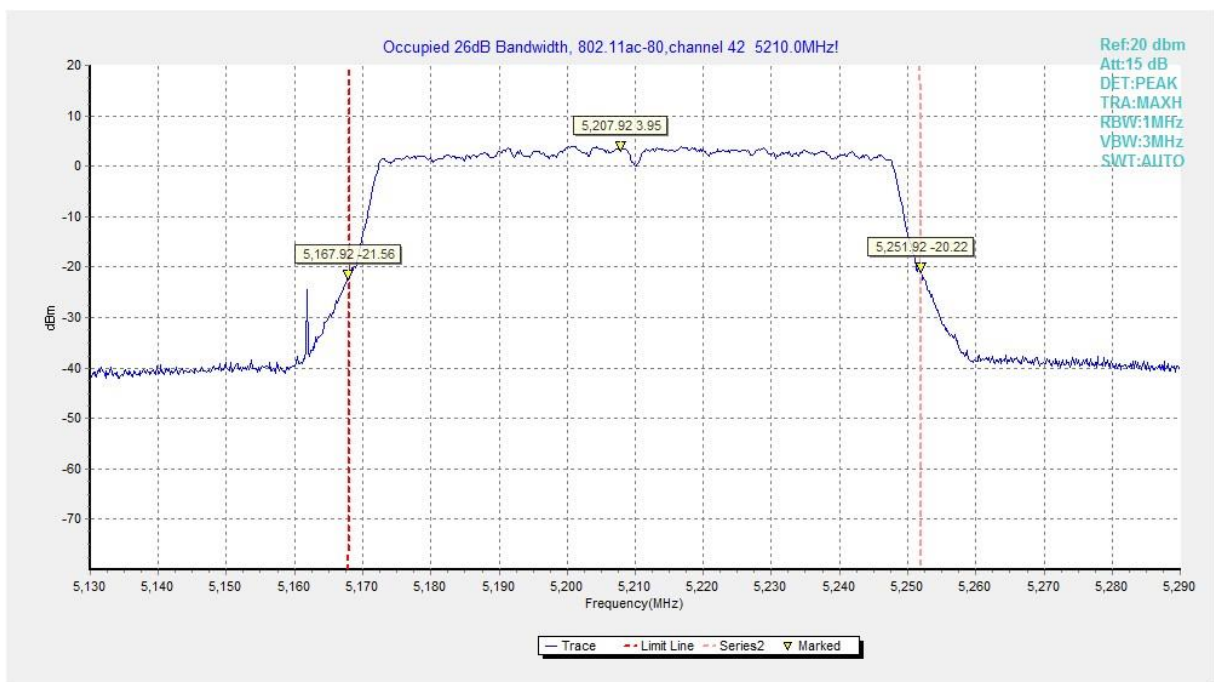
Fig.29 Occupied 26dB Bandwidth (802. 11ac-HT80, 5210MHz)
