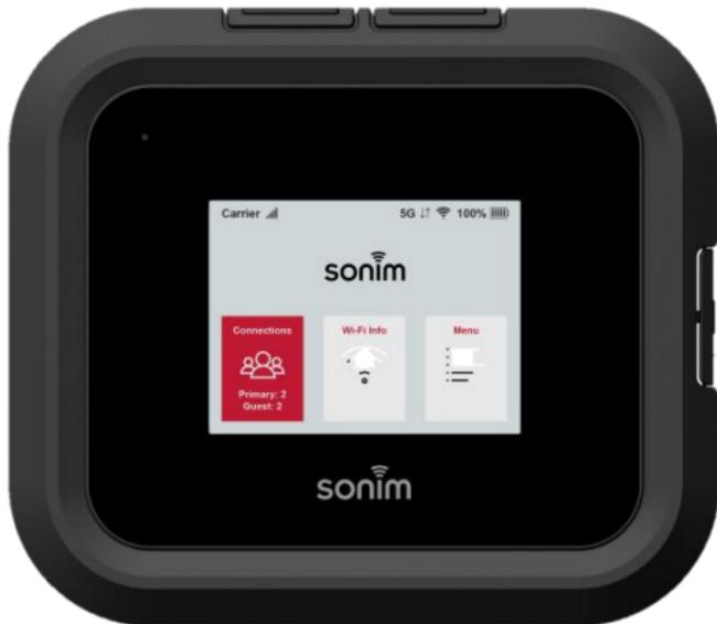
**The device screen is a 2.4 inch TFT LCD with Capacitive Touch.**
