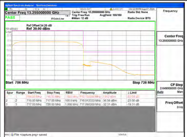
B12 / 10MHz / High CH / QPSK / FULL RB
