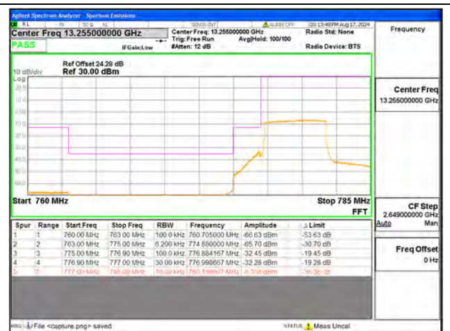
B13 / 5MHz / Low CH / QPSK / FULL RB
