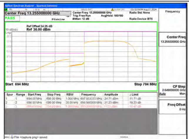
B12 / 3MHz / Low CH / QPSK / FULL RB
