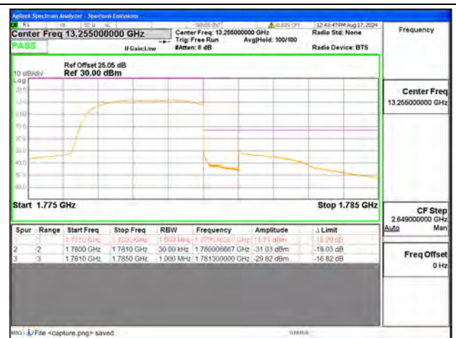
B66 / 3MHz / High CH / QPSK / FULL RB
