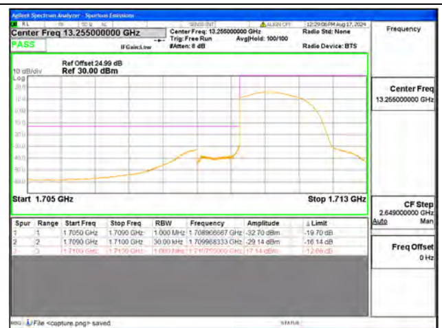
B4 / 1.4MHz / Low CH / QPSK / FULL RB
