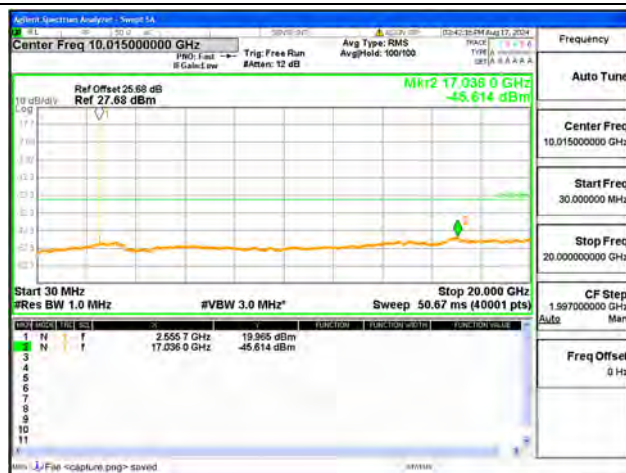
B7-30M-20G / 15MHz / High CH / QPSK
