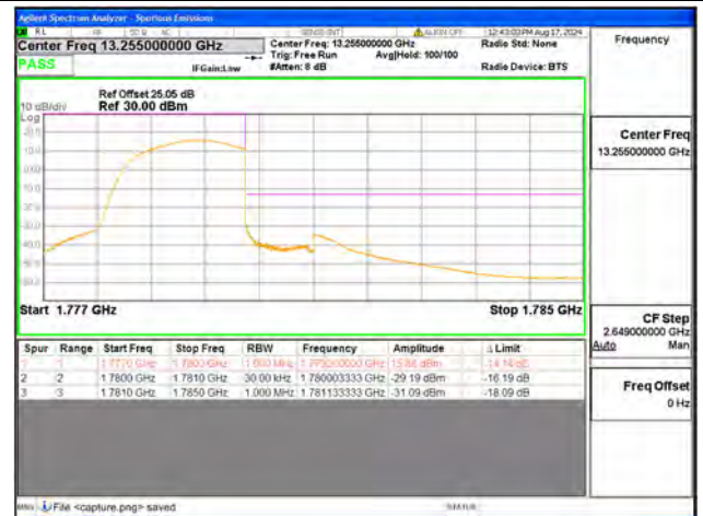
B66 / 1.4MHz / High CH / QPSK / FULL RB
