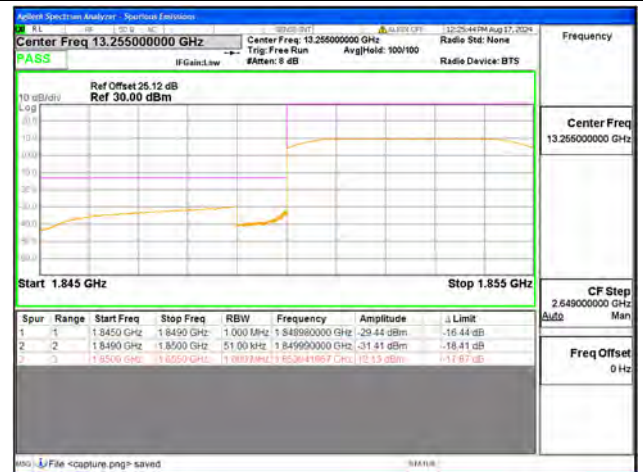
B2 / 5MHz / Low CH / QPSK / FULL RB
