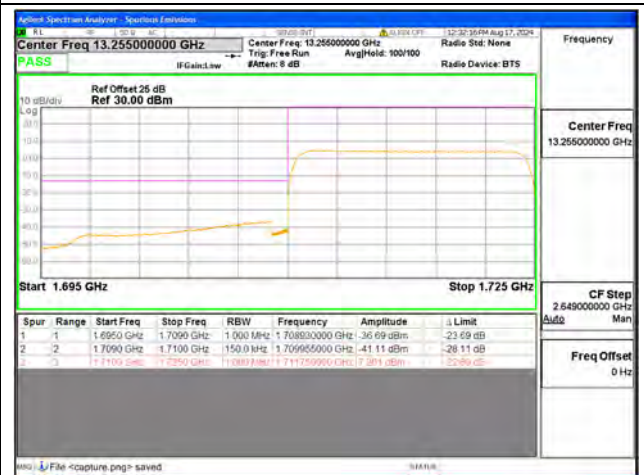
B4 / 15MHz / Low CH / QPSK / FULL RB
