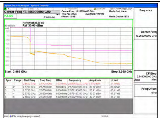
B7 / 10MHz / High CH / QPSK / FULL RB
