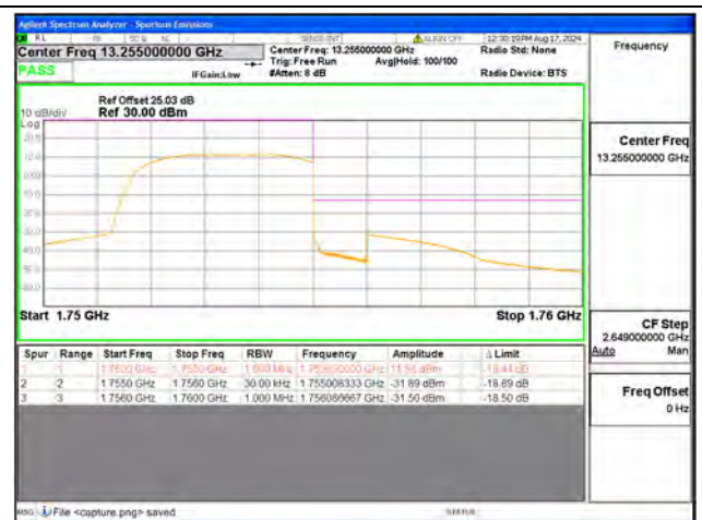
B4 / 3MHz / High CH / QPSK / FULL RB
