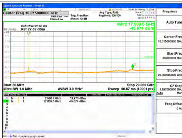
B7-30M-20G / 10MHz / High CH / QPSK
