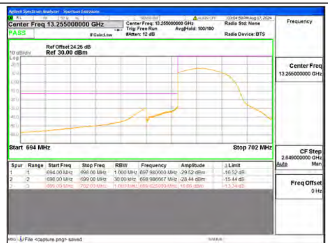
B12 / 1.4MHz / Low CH / QPSK / FULL RB
