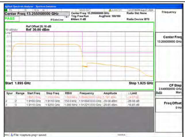
B2 / 15MHz / High CH / QPSK / FULL RB
