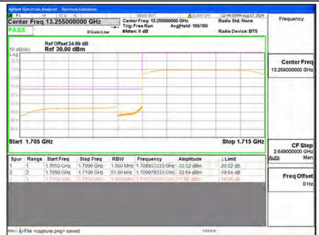
B66 / 5MHz / Low CH / QPSK / FULL RB
