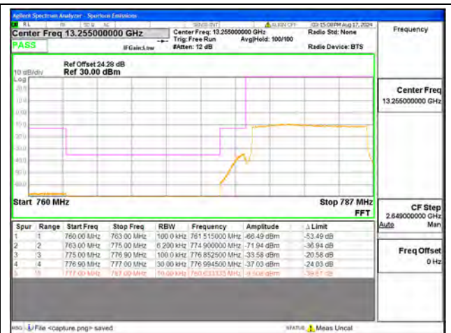
B13 / 10MHz / Low CH / QPSK / FULL RB
