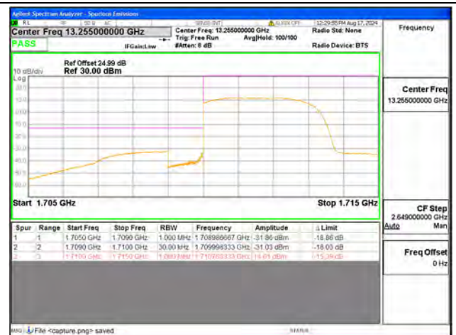
B4 / 3MHz / Low CH / QPSK / FULL RB
